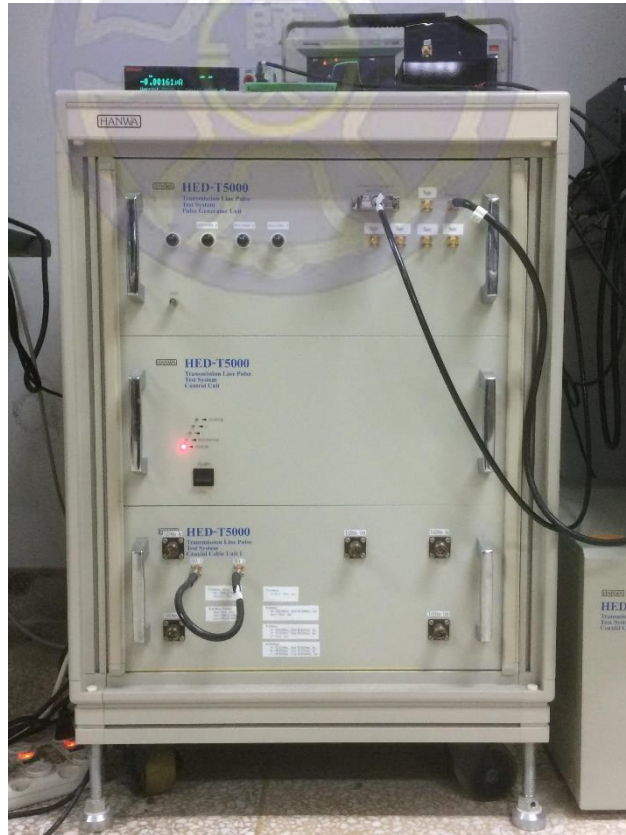
Fig. 3.30. Transmission-line pulsing (TLP) system.
