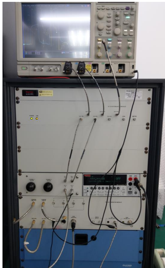
Fig. 2.33. The very-fast transmission-line pulse (VF-TLP) measured system [26].
