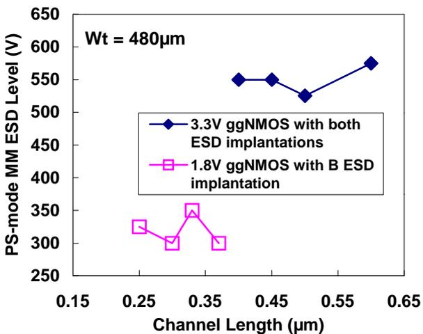
**Fig. 10:** The relation between PS-mode MM ESD level and channel length of ggNMOS with a total width of 480μm.
