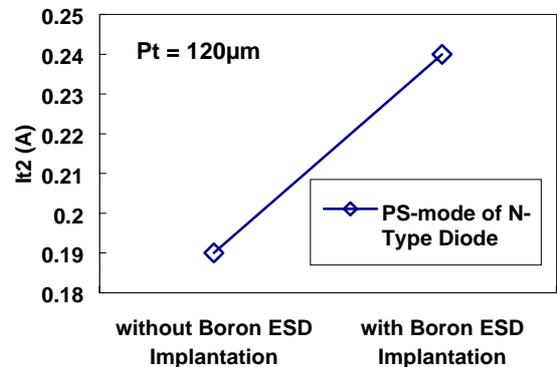
**Fig. 16:** The It2 of the N-type diode in reverse-biased condition with or without B ESD implantation.
