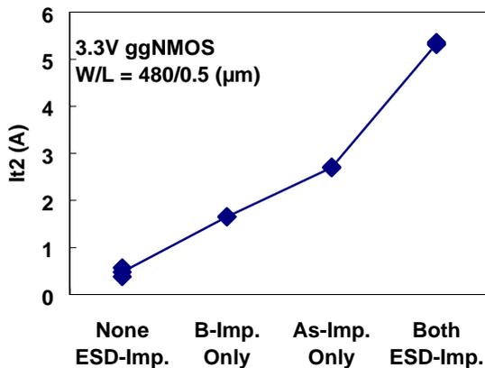
**Fig. 6:** The It2 of the 3.3V ggNMOS with different ESD implantations.
