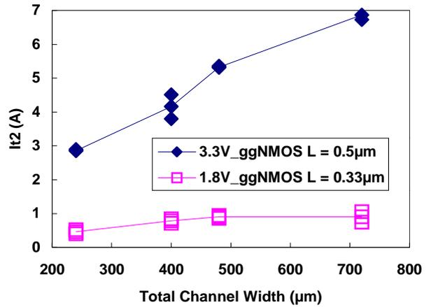
**Fig. 11:** Dependence of It2 on the total channel width of ggNMOS.
