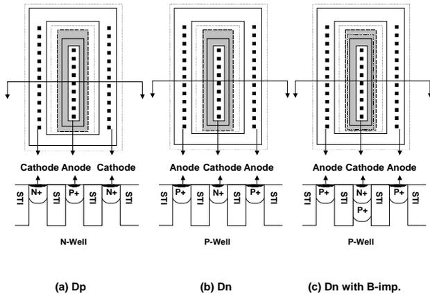
**Fig. 2:** The layout top view and device cross-sectional view for (a) P-type diode, (b) N-type diode, and (c) N-type diode with B ESD implantation.
