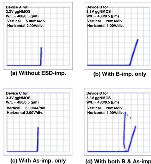
**Fig. 3:** The measured dc I-V curves of NMOS in the (a) device A, (b) device B, (c) device C, and (d) device D, under gate-grounded condition.
