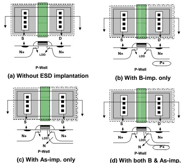
**Fig. 1:** The layout top view and device cross-sectional view of NMOS in (a) device A, (b) device B, (c) device C, and (d) device D, with different ESD implantations.
