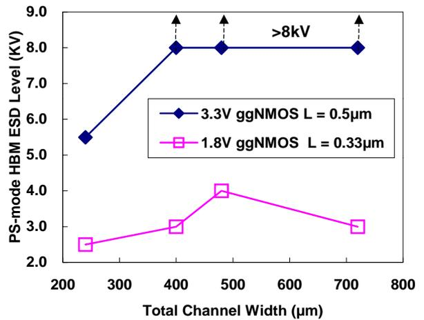
**Fig. 12:** Dependence of PS-mode HBM ESD level on the total channel width of ggNMOS.
