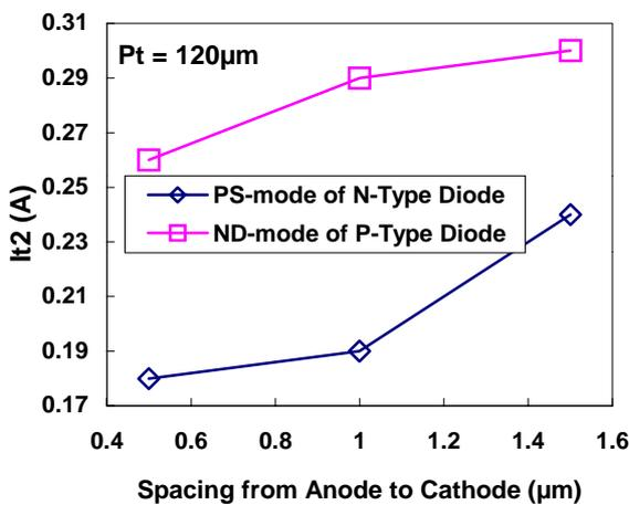
**Fig. 20:** The relation between  $I_{t2}$  and the spacing from anode to cathode of diode with a total perimeter of  $120\mu\text{m}$  under reverse-biased condition.
