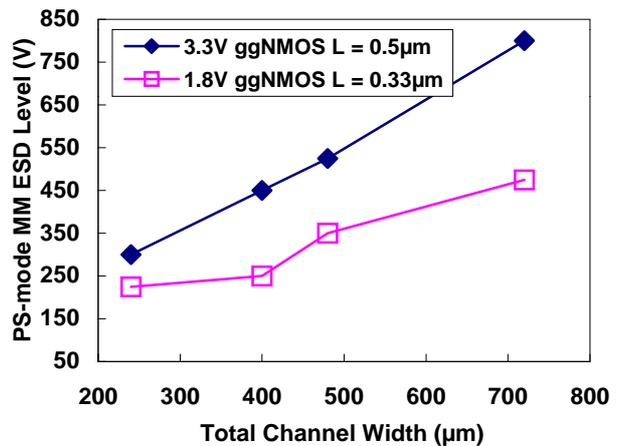
**Fig. 13:** Dependence of PS-mode MM ESD level on the total channel width of ggNMOS.
