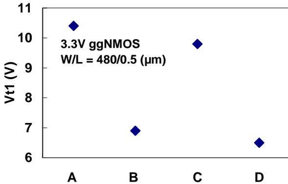
**Fig. 4:** The Vt1 defined at I=1mA of the 3.3V ggNMOS with different ESD implantations, whereas the four devices (A, B, C, and D) have the same W/L of 480μm/0.5μm.
