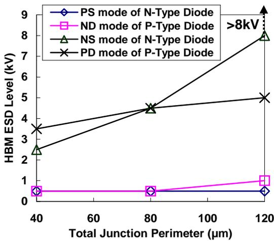
**Fig. 19:** Dependence of HBM VESD on the total junction perimeter of P-type and N-type diodes.
