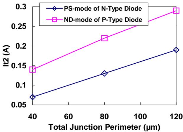
**Fig. 18:** Dependence of  $I_{t2}$  on the total junction perimeter of diode under reverse-biased condition.
