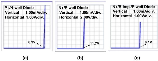
**Fig. 14:** The measured dc I-V curves of the (a) P-type diode, (b) N-type diode, and (c) N-type diode with B ESD implantation.
