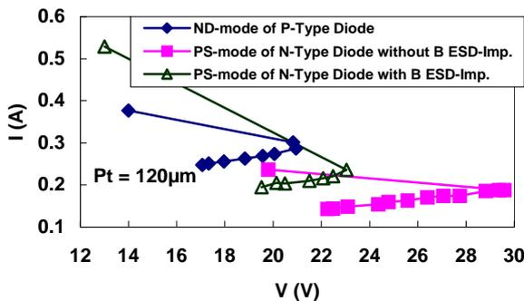
**Fig. 15:** The TLPG-measured I-V curves of the different diodes under reverse-biased condition.
