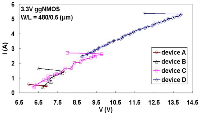
**Fig. 5:** The TLPG-measured I-V curves of the 3.3V gate-grounded NMOS with different ESD implantations.
