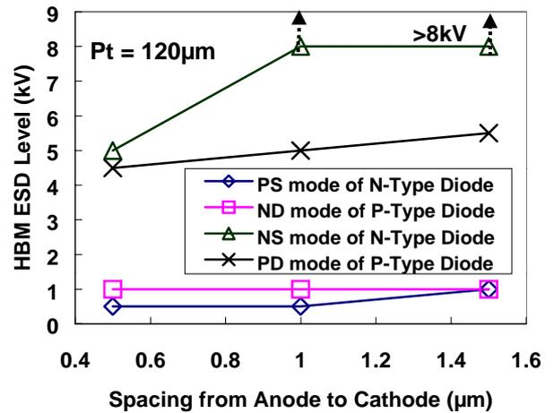
**Fig. 21:** The relation between HBM ESD level and the spacing from anode to cathode of diode.
