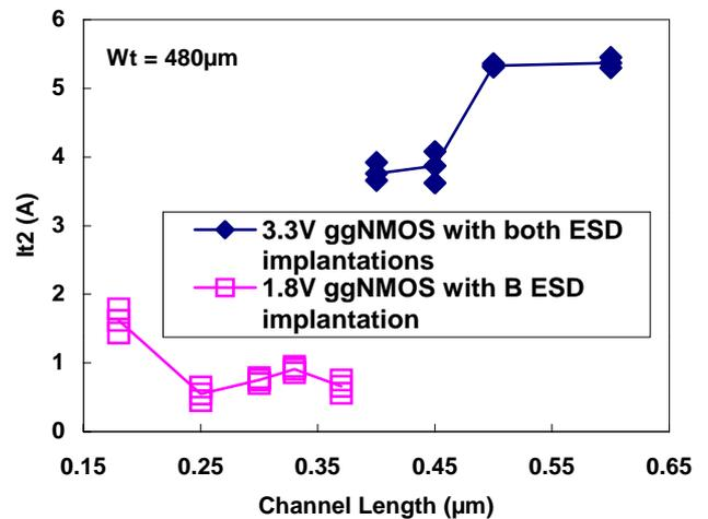
**Fig. 8:** The relation between It2 and channel length of ggNMOS with a total width of 480μm.
