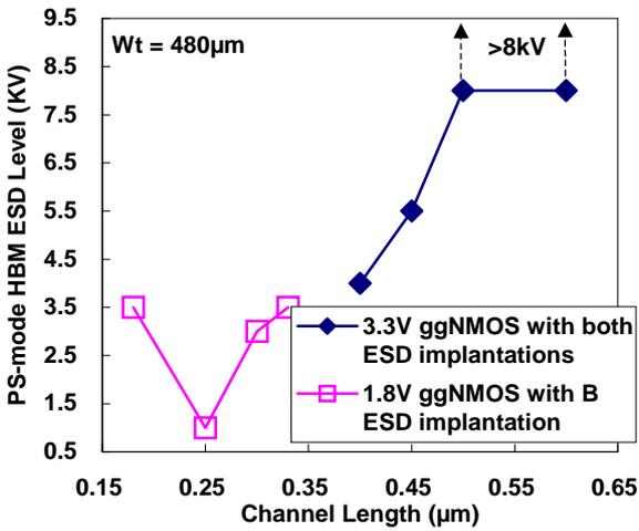
**Fig. 9:** The relation between PS-mode HBM ESD level and channel length of ggNMOS with a total width of 480μm.
