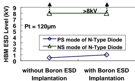
**Fig. 17:** The PS-mode and NS-mode HBM ESD levels of the N-type diodes with or without B ESD implantation.
