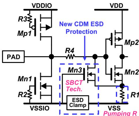
Fig. 2. CDM ESD protection with the proposed self-biased current trigger mechanism and source pumping design.
