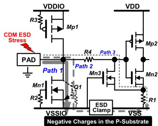
Fig. 3. CDM ESD current discharging paths in the CDM ESD protection with self-biased current trigger mechanism and source pumping design under negative CDM ESD stresses.
