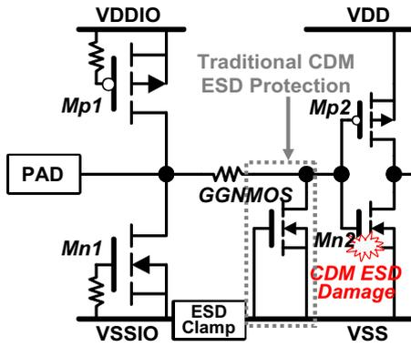
Fig. 1. Traditional CDM ESD protection with gate-grounded NMOS (GGNMOS) added to the gate of input stages.
