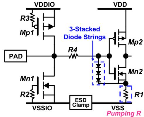
Fig. 4. CDM ESD protection with 3-stacked diode strings.
