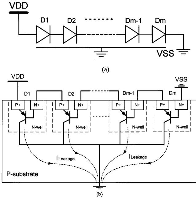
Fig. 2. (a) The schematic circuit diagram and (b) the cross-sectional view, of the pure diode string realized in a  $P$ -substrate  $N$ -well CMOS technology.
