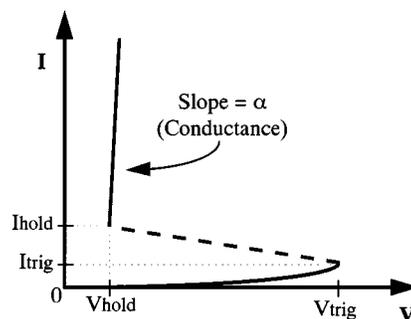
Fig. 6. The typical *I*–*V* curve of an NCLSCR device.
