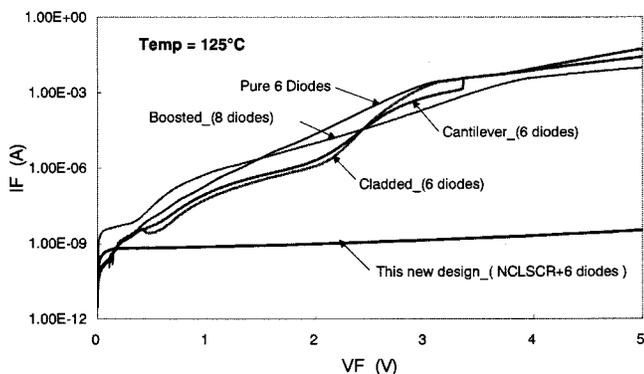
Fig. 9. The measured  $I-V$  curves of the diode strings among the different designs at the temperature of 125 °C ( $Y$  axis is drawn in the log scale).
