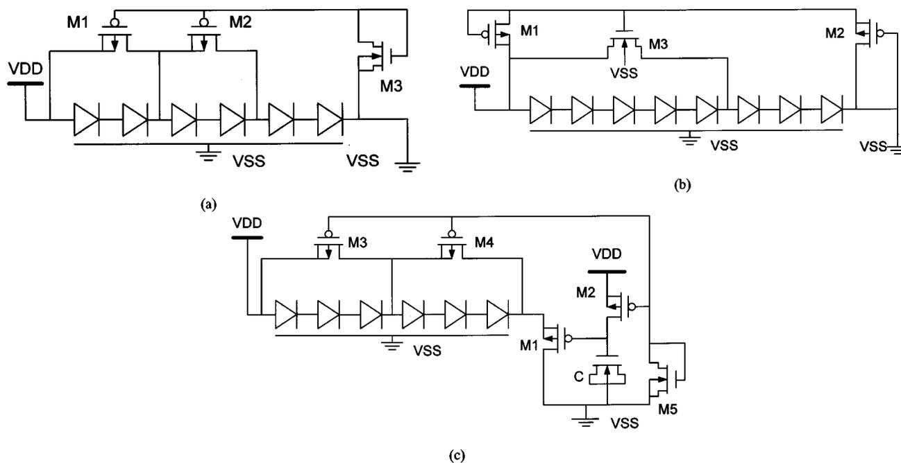
Fig. 3. The circuit diagrams of: (a) the *Cladded diode string*, (b) the *Boosted diode string*, and (c) the *Cantilever diode string*, in the previous diode string designs [15].
