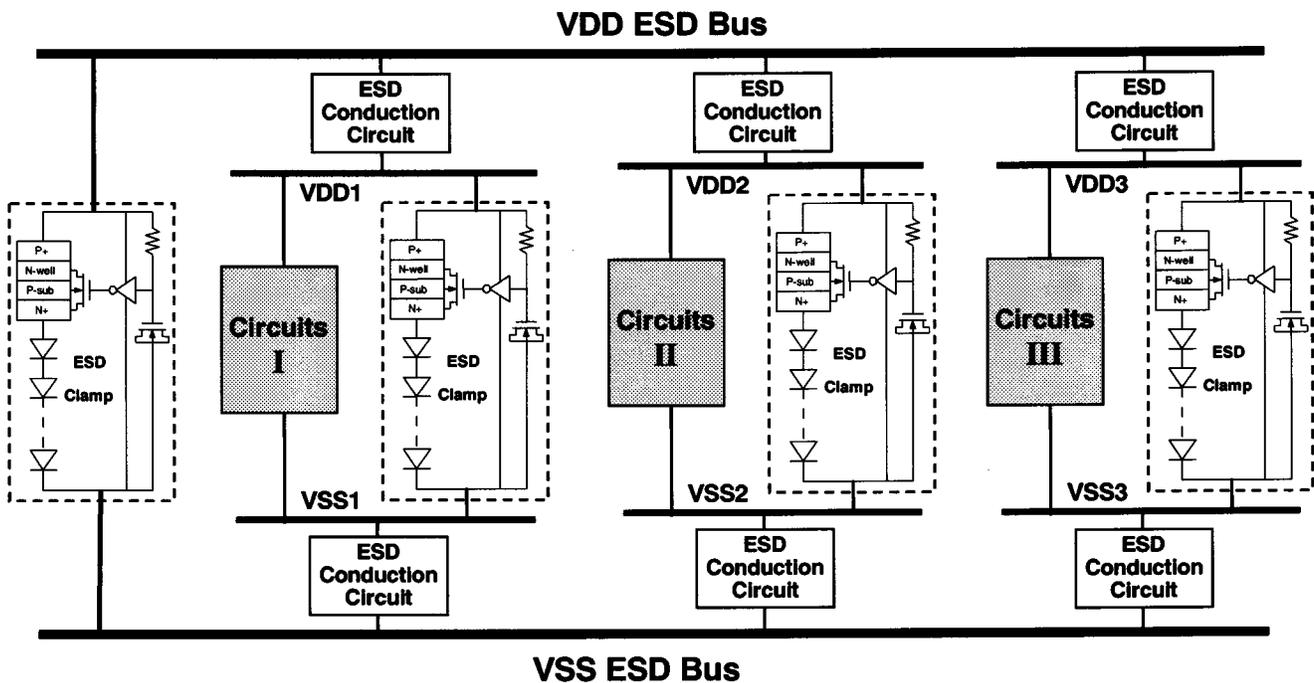
Fig. 15. Another application example of the new low-leakage diode string in a CMOS IC to achieve the whole-chip ESD protection scheme with the VDD and VSS ESD buses.
