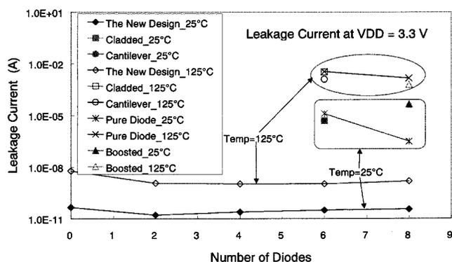
Fig. 10. The leakage currents among the different diode string designs at the temperatures of 25 °C and 125 °C under 3.3-V voltage bias ( $Y$  axis is drawn in the log scale).
