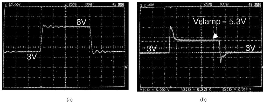
Fig. 13. (a) The voltage waveform the original 3–8-V voltage pulse, and (b) the degraded voltage waveform clamped by the VDD-to-VSS ESD clamp circuit with an NCLSCR and four stacked diodes. (Y axis = 2 V/Div., X axis = 100 ns/Div.).
