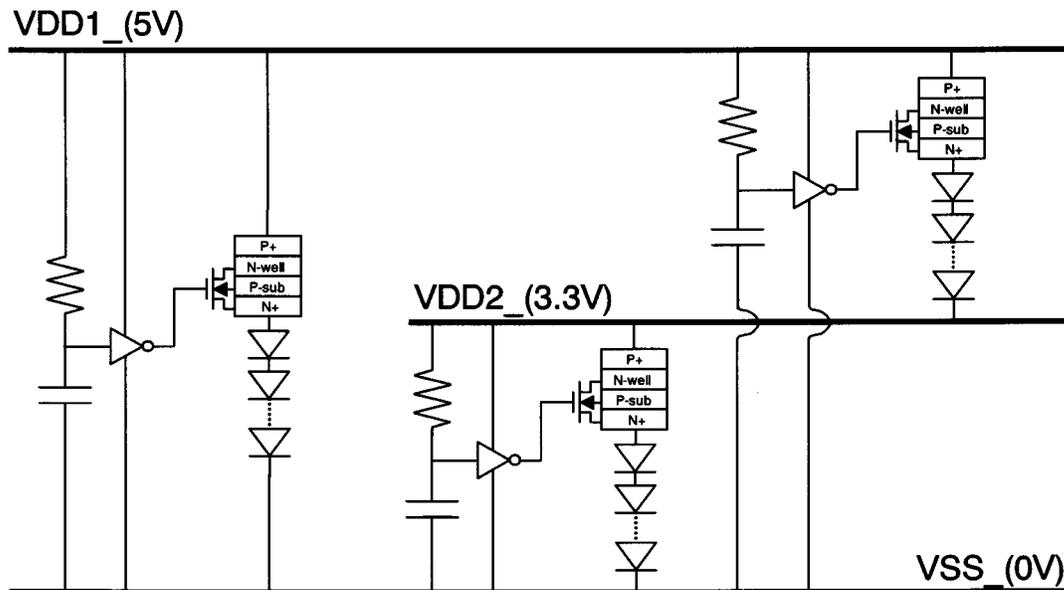
Fig. 14. The application of the new low-leakage diode string for using in the ESD clamp circuits between different power rails, which have different VDD voltage levels in a CMOS IC.
