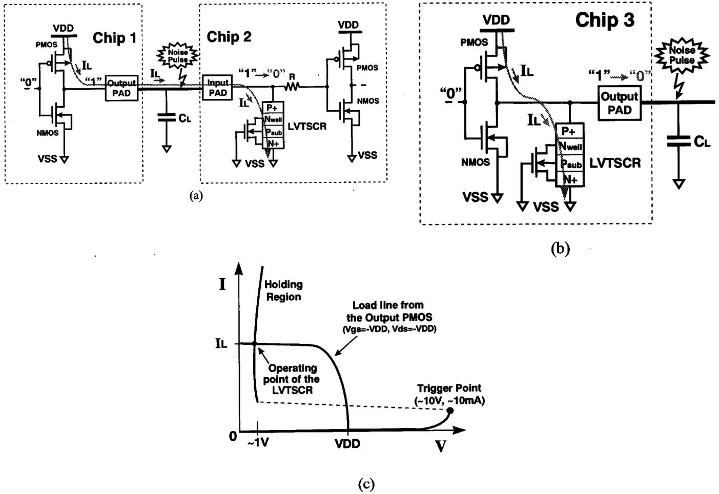
Fig. 4. The schematic diagram to show the LVTSCR in: (a) an input ESD protection circuit in Chip 2; (b) an output ESD protection circuit in Chip 3, being accidentally triggered on by the system-level overshooting noise pulses; and (c) intercept point between the  $I$ - $V$  curves of the output PMOS and the LVTSCR decides the voltage level on the pad and the leakage current  $I_L$  from VDD to VSS.
