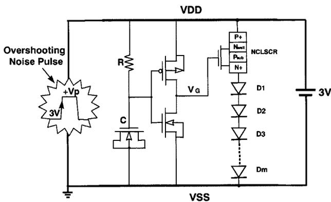
Fig. 12. The experimental setup to verify the latch-up issue of the VDD-to-VSS ESD clamp circuit with the new low-leakage diode string under 3-V VDD bias and a coupled overshooting noise pulse on the VDD power line.
