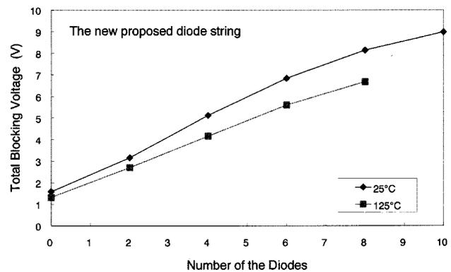
Fig. 8. The relation between the total blocking voltage of this new low-leakage diode string and the number of stacked diodes at the temperatures of 25  $^{\circ}\text{C}$  and 125  $^{\circ}\text{C}$ .
