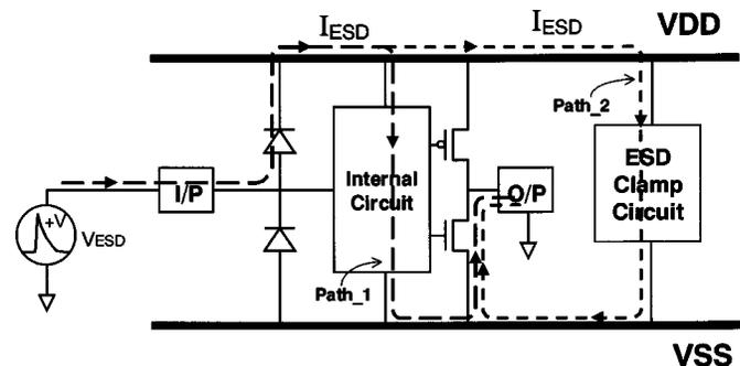
Fig. 1. The ESD current discharging paths in an IC during the pin-to-pin ESD stress condition. If the IC has no ESD clamp circuit between the VDD and VSS power rails, the ESD current is discharged through the Path\_1, which often causes ESD damage located at the internal circuits. If the IC has an effective ESD clamp circuit between the VDD and VSS power rails, the ESD current is discharged through the Path\_2.
