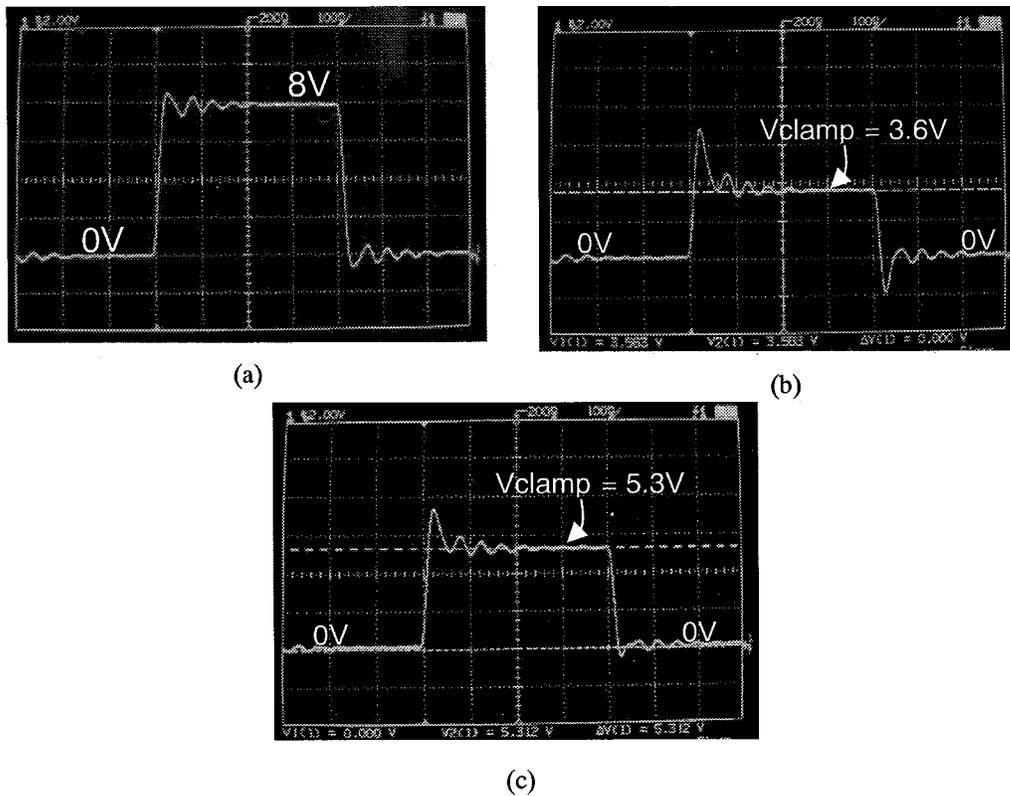
Fig. 11. The voltage waveforms of: (a) the original 0–8-V voltage pulse, (b) the degraded voltage pulse clamped by the VDD-to-VSS ESD clamp circuit with an NCLSCR and twostacked diodes, and (c) the degraded voltage pulse clamped by the VDD-to-VSS ESD clamp circuit with an NCLSCR and sixstacked diodes. (Y axis = 2 V/div., X axis = 100 ns/div.).
