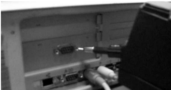
Fig. 10. The ESD gun hits the backside of the PC case to test the system-level ESD susceptibility of a keyboard in the PC system.
