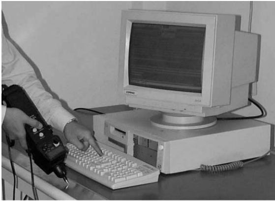
Fig. 9. The ESD gun hits the table to test the system-level ESD susceptibility of a keyboard in the PC system.
