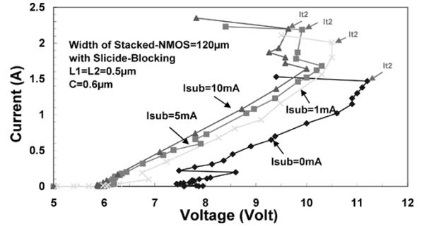
Fig. 8. TLP-measured  $I$ - $V$  curves of the stacked-nMOS device with different substrate-triggered currents.
