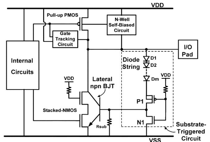
Fig. 4. Schematic circuit diagram of the substrate-triggered stacked-nMOS device with substrate-triggered circuit for the mixed-voltage I/O circuits.
