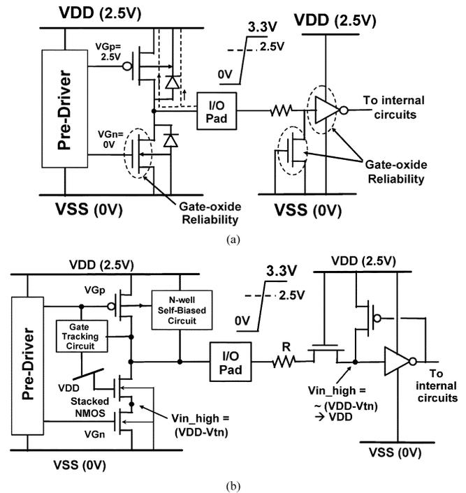
Fig. 1. Typical circuit diagrams for (a) the traditional CMOS I/O buffer, and (b) the mixed-voltage I/O buffer with the stacked-nMOS and the N-well self-biased pMOS.
