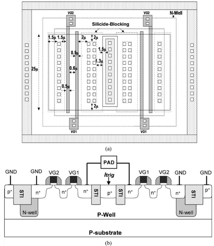
Fig. 3. (a) Finger-type layout pattern, and (b) the corresponding cross-sectional view, of the substrate-triggered stacked-nMOS device for mixed-voltage I/O circuit in a p-substrate CMOS process.
