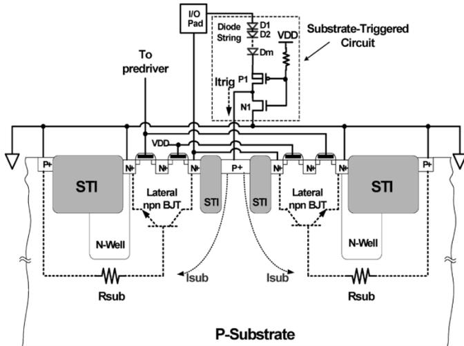
Fig. 5. Cross-sectional view of the substrate-triggered stacked-nMOS device with substrate-triggered circuit for the mixed-voltage I/O circuits.
