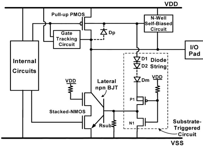
Fig. 6. Modified design of the substrate-triggered stacked-nMOS device with substrate-triggered circuit for the mixed-voltage I/O circuits without generating extra additional capacitance to the I/O pad.
