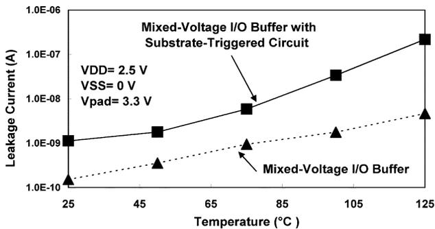
Fig. 11. Leakage currents of the mixed-voltage I/O buffers with or without the substrate-triggered circuit under different temperatures.
