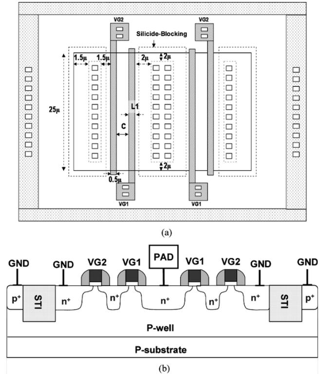
Fig. 2. (a) Finger-type layout pattern, and (b) the corresponding cross-sectional view, of the stacked-nMOS device for mixed-voltage I/O circuit in a p-substrate CMOS process.
