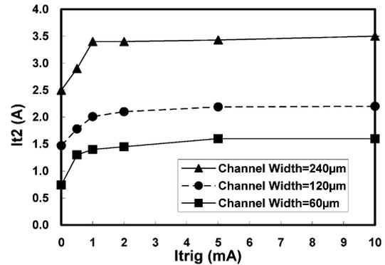
Fig. 9. Dependence of  $I_{t2}$  level on the substrate-triggered current ( $I_{trig}$ ) under the different channel widths of substrate-triggered stacked-nMOS device.
