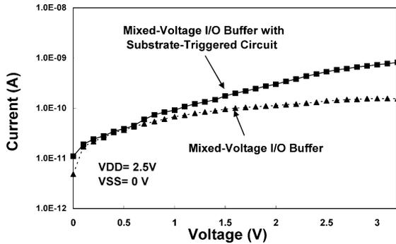
Fig. 10. Comparison of the leakage currents of the mixed-voltage I/O buffers with or without the proposed substrate-triggered circuit. The mixed-voltage I/O buffer in this measurement has a channel width of  $240\ \mu\text{m}$  in the stacked nMOS and a channel width of  $480\ \mu\text{m}$  in the pull-up pMOS.
