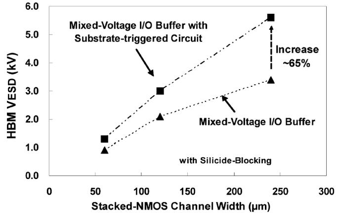
Fig. 12. Positive-to- $V_{SS}$  (PS-mode) HBM ESD levels of the mixed-voltage I/O buffers with or without the substrate-triggered circuit, realized in a  $0.25\text{-}\mu\text{m}$  CMOS process with silicide-blocking process.
