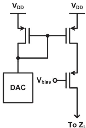
**Fig. 11.** Output driver implemented by current-mode DAC with output cascode transistor and current mirror.
