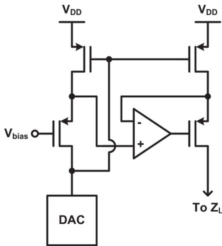
**Fig. 13.** Output driver implemented by DAC with current mirror and voltage-controlled resistor.
