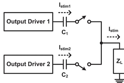
**Fig. 17.** Stimulator with fail-safe blocking capacitors realized by using high-frequency current-switching technique.
