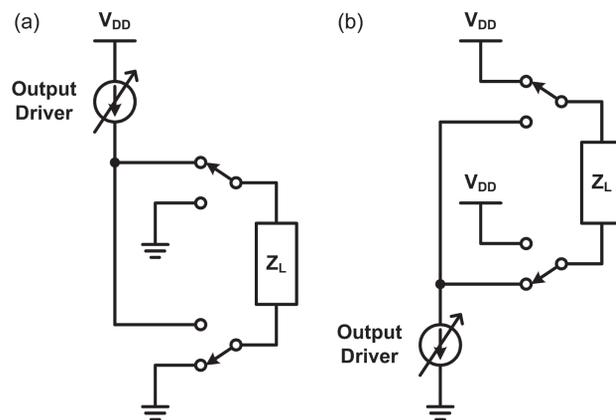
Fig. 6. Bipolar configuration with output driver of (a) current source and (b) current sink, for biphasic stimulation.
