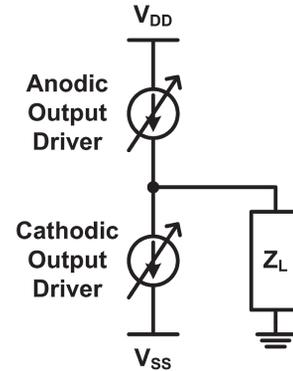
Fig. 5. Monopolar configuration with anodic and cathodic output drivers for biphasic stimulation.
