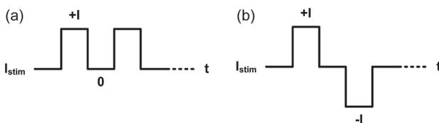
Fig. 3. Current waveforms of (a) monophasic stimulation and (b) biphasic stimulation.
