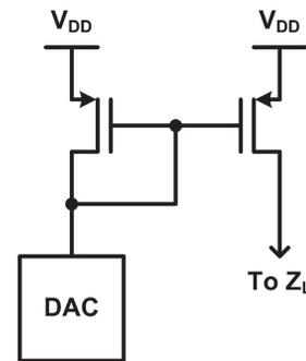
Fig. 8. Output driver implemented by current-mode DAC with current mirror.
