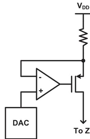
**Fig. 14.** Output driver implemented by voltage-mode DAC with voltage follower.
