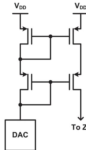
Fig. 9. Output driver implemented by current-mode DAC with fully cascode current mirror.
