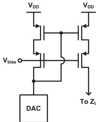
**Fig. 10.** Output driver implemented by current-mode DAC with wide-swing cascode current mirror.
