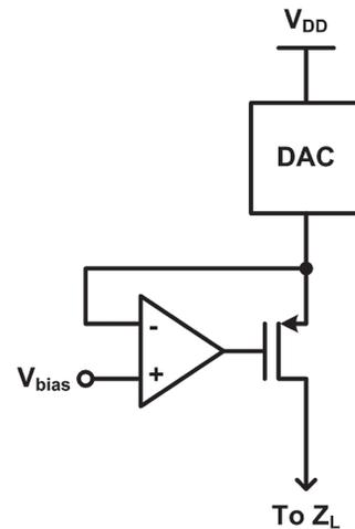
**Fig. 12.** Output driver implemented by DAC with voltage-controlled resistor.
