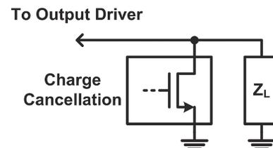
**Fig. 18.** Stimulator with charge cancellation to avoid charge accumulation.
