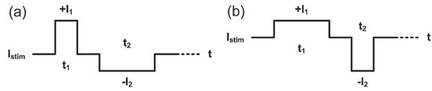
Fig. 4. Current waveforms of different biphasic, charge-balanced stimulation.
