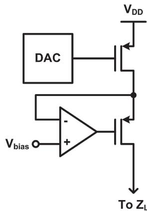
**Fig. 16.** Output driver implemented by voltage-mode-DAC-controlled resistor with voltage follower.
