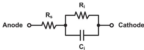
Fig. 2. Equivalent circuit model of electrode and tissue.
