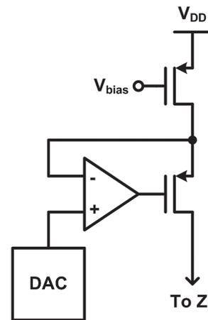
**Fig. 15.** Output driver implemented by voltage-mode DAC with voltage follower and active load.
