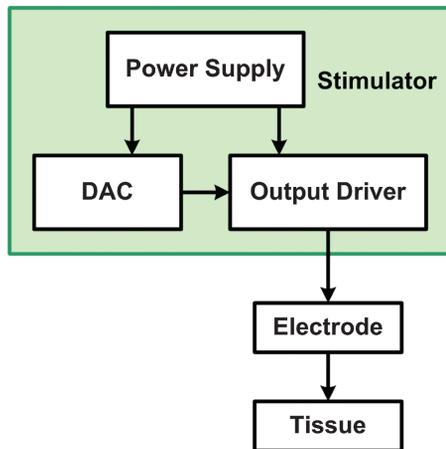
Fig. 1. Block diagram of electrical stimulator.
