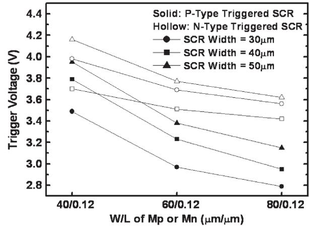
Fig. 10. TLP measured trigger voltage of the p- and n-type triggered design with different widths of Mp, Mn, and SCR devices.
