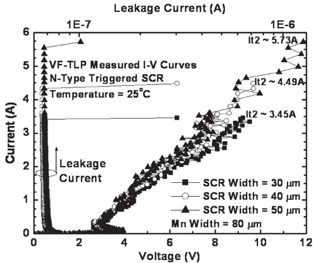
Fig. 13. VF-TLP measured  $I$ - $V$  curves of the fabricated power-rail ESD clamp circuits with the n-type triggered SCR device of different widths under positive VDD-to-VSS ESD stress. The VF-TLP is with a pulsewidth of 10 ns and a rise time of 200 ps.
