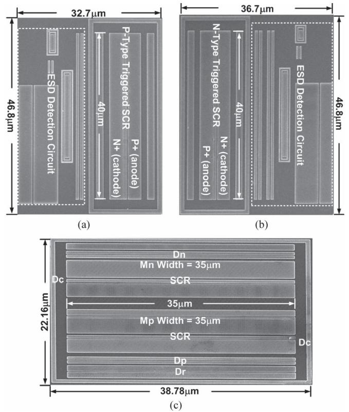
Fig. 8. Microphotograph of the fabricated power-rail ESD clamp circuits with the (a) p- and (b) n-type triggered SCR devices, as the ESD clamp devices, and (c) the embedded ESD-transient detection circuit.
