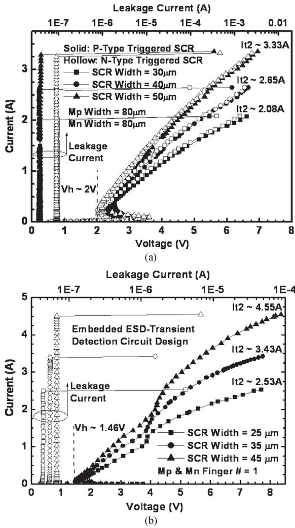
Fig. 9. TLP measured  $I-V$  curves of the fabricated power-rail ESD clamp circuits with the SCR devices of different widths under positive VDD-to-VSS ESD stress, (a) the p- and n-type triggered SCR designs, and (b) the embedded ESD-transient detection circuit design.
