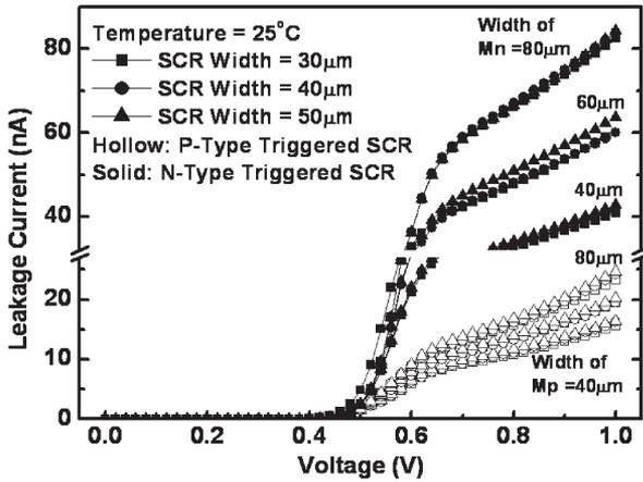
Fig. 11. Measured dc  $I$ - $V$  curves of the fabricated power-rail ESD clamp circuits with SCR devices of different widths.
