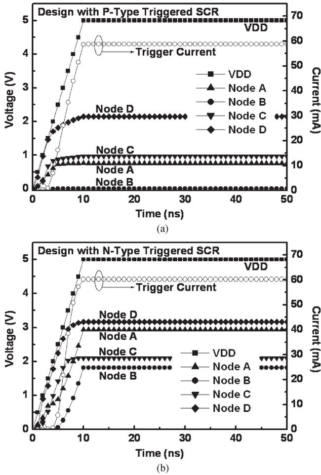
Fig. 7. Simulated voltages on the nodes and the trigger current of the ESD detection circuit with the (a) p- and (b) n-type triggered SCR devices in the 65-nm CMOS process under the ESD-like transition.
