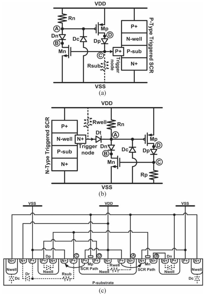
Fig. 5. Proposed ultralow standby leakage power-rail ESD clamp circuits with the (a) p- and (b) n-type triggered SCR devices, as the ESD clamp devices, and (c) the embedded ESD-transient detection circuit in the cross-sectional view.
