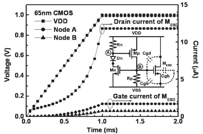
Fig. 3. Simulated node voltages of the capacitor-less power-rail ESD clamp circuit [17], the drain current, and the gate current flowing through the clamp device  $M_{ESD}$  under the normal power-on transition.
