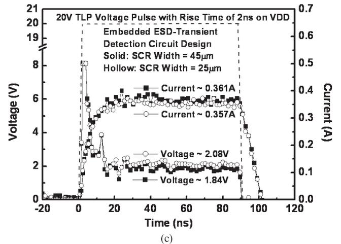
Fig. 12. Measured voltage and current waveforms of the fabricated power-rail ESD clamp circuits with the SCR devices under the TLP transition, the (a) p- and (b) n-type triggered SCR devices, and (c) the embedded ESD-transient detection circuit design.
