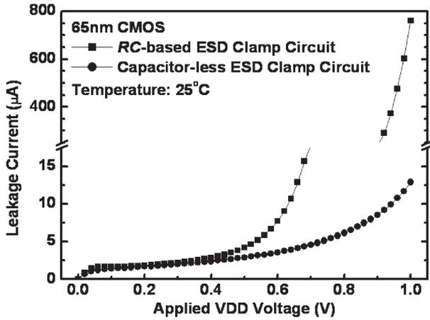
Fig. 4. Measured standby leakage currents of the traditional RC-based and the capacitor-less power-rail ESD clamp circuits.
