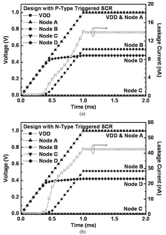
Fig. 6. Simulated voltage waveforms on the nodes and the leakage current of the ESD detection circuit with the (a) p- and (b) n-type triggered SCR devices in the 65-nm 1-V CMOS process under the normal power-on transition.
