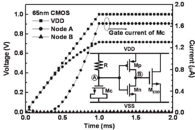
Fig. 2. Simulated node voltages of the traditional  $RC$ -based power-rail ESD clamp circuit [16] and the gate current flowing through MOS capacitor  $M_c$  under the normal power-on condition with a rise time of 1 ms in a 65-nm CMOS process.
