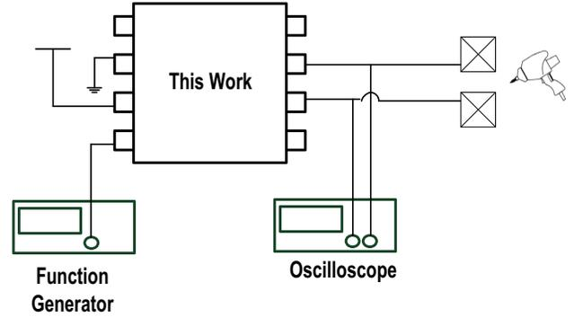
Fig. 12. System-level ESD testing setup for the co-packaged CAN bus transceiver IC with TVS chips.
