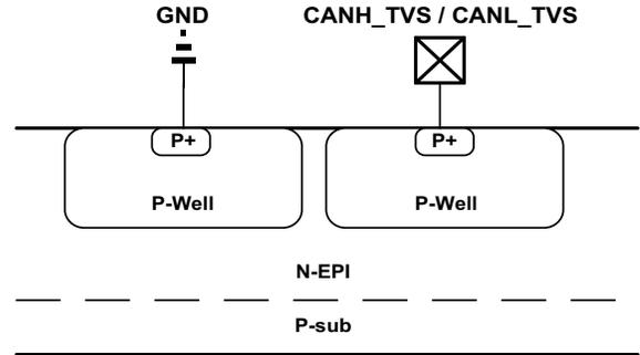
Fig. 4. Cross-sectional view of the proposed TVS device for CAN bus protection.
