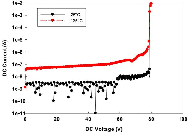
Fig. 8. DC measured I-V curves of the TVS device at 25°C and 125°C.
