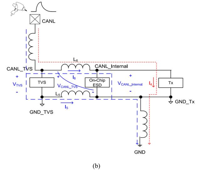
Fig. 10. Current discharge path of the proposed co-packaged TVS chips and CAN bus transceiver IC (a) CANH under negative ESD gun contact stress and (b) CANL under positive ESD gun contact stress.
