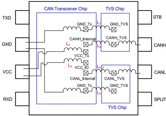
Fig. 6. Proposed protection scheme for the CAN bus with the co-packaged transceiver IC and TVS chips.
