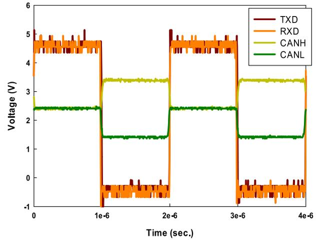
Fig. 11. Voltage waveforms of the signals at CANH and CANL during normal circuit operation.
