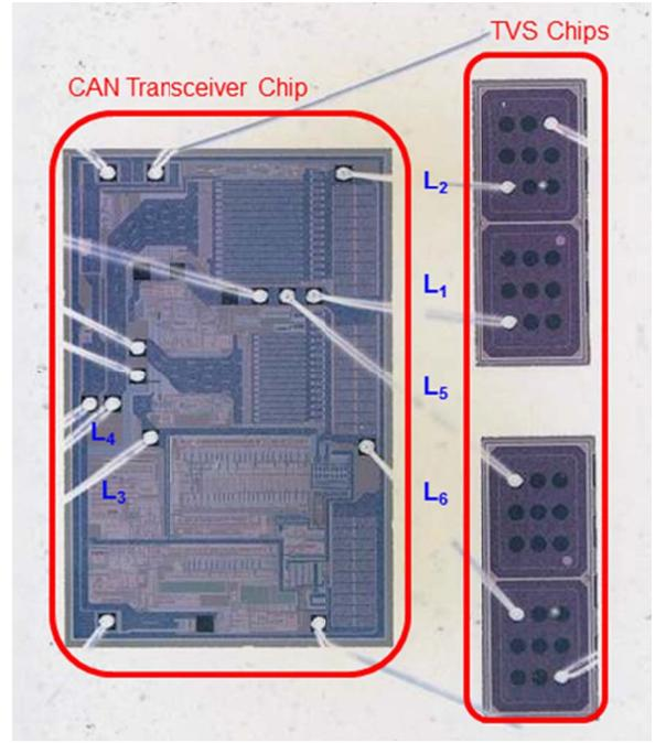
Fig. 7. Proposed whole chip of the co-packaged TVS chips and CAN bus transceiver IC. The TVS is a bi-directional high-voltage PNP device.
