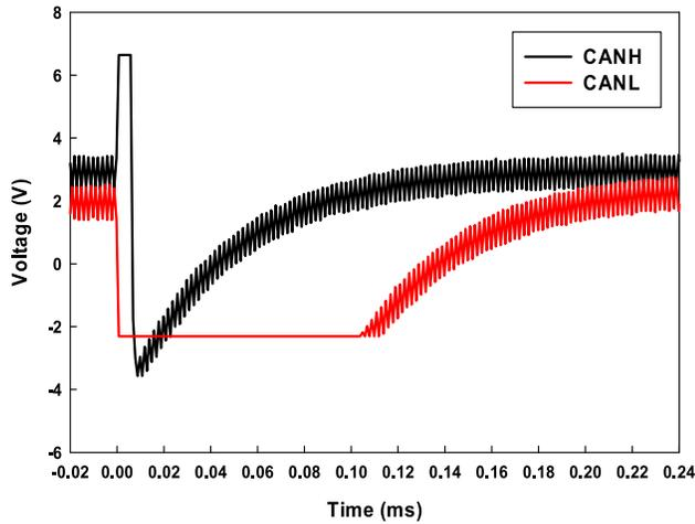
Fig. 13. Voltage waveforms of signals at CANH and CANL during IEC61000-4-2 ESD test of 8 kV at CANL.
