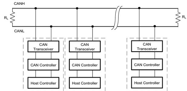
Fig. 1. System architecture of the CAN bus interface.
