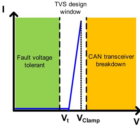
Fig. 5. ESD design window and I-V curve of the TVS device for the proposed CAN bus transceiver IC.
