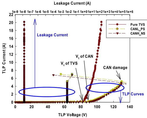
Fig. 9. TLP measured I-V curves of the TVS device and CAN transceiver without co-packaged TVS chips.
