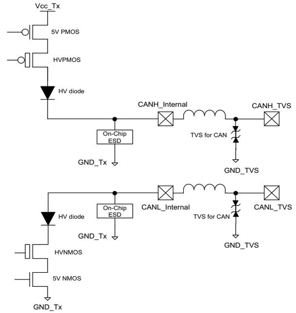
Fig. 3. Design scheme of the proposed co-packaged TVS chips and CAN bus transceiver.
