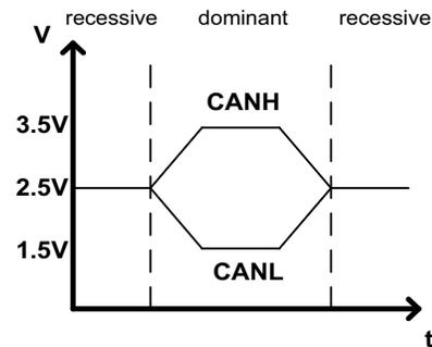
Fig. 2. CAN bus signal levels for the CANH and CANL at the recessive and dominant states.
