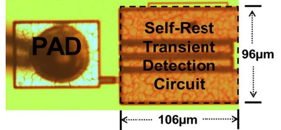
Fig. 6. Die photograph of the new proposed on-chip self-reset transient detection circuit fabricated in a  $0.18\text{-}\mu\text{m}$  CMOS process.
