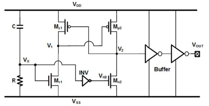
Fig. 2. New proposed on-chip self-reset transient detection circuit.
