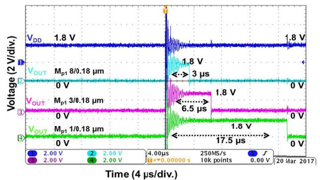
Fig. 12. Measured  $V_{DD}$  and  $V_{OUT}$  waveforms of the new proposed on-chip self-reset transient detection circuit with different channel widths of  $M_{p1}$  under EFT test with an EFT voltage of  $+300$  V.
