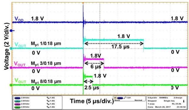
Fig. 9. Measured  $V_{DD}$  and  $V_{OUT}$  waveforms of the new proposed on-chip self-reset transient detection circuit with different channel widths of  $M_{p1}$  under system-level ESD test with an ESD voltage of  $+300$  V.
