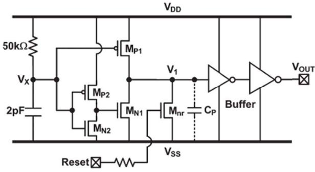
Fig. 1. Previous on-chip transient detection circuit [15].
