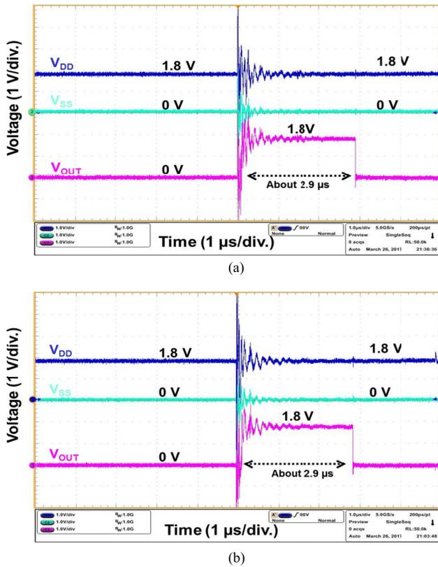
Fig. 8. Measured  $V_{DD}$ ,  $V_{SS}$ , and  $V_{OUT}$  waveforms of the new proposed on-chip self-reset transient detection circuit under system-level ESD tests with ESD voltages of (a)  $+0.2$  kV and (b)  $-0.2$  kV.
