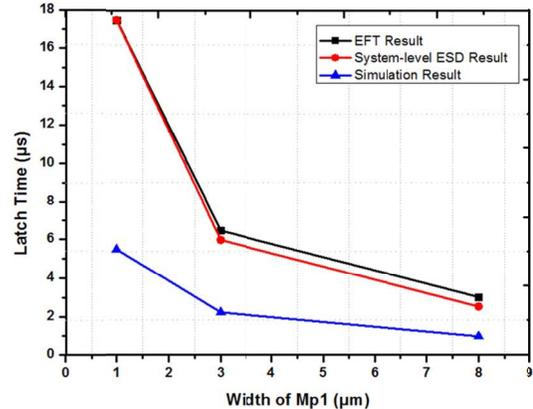
Fig. 13. Relations between the different channel widths of  $M_{p1}$  and the latch times under system-level ESD, EFT tests, and HSPICE simulation.
