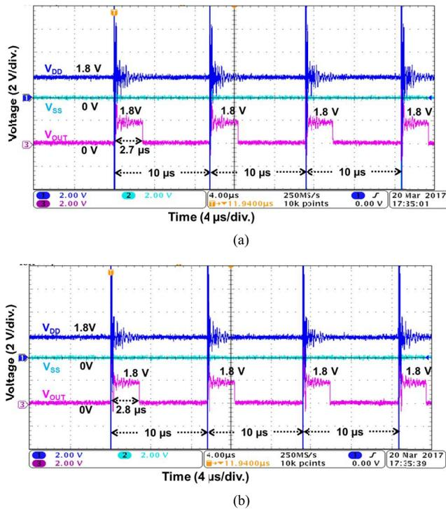
Fig. 11. Measured  $V_{DD}$ ,  $V_{SS}$ , and  $V_{OUT}$  waveforms of the new proposed on-chip self-reset transient detection circuit under EFT tests with EFT voltage of (a)  $+0.2$  kV and (b)  $-0.2$  kV. The repetition rates are 100 kHz.
