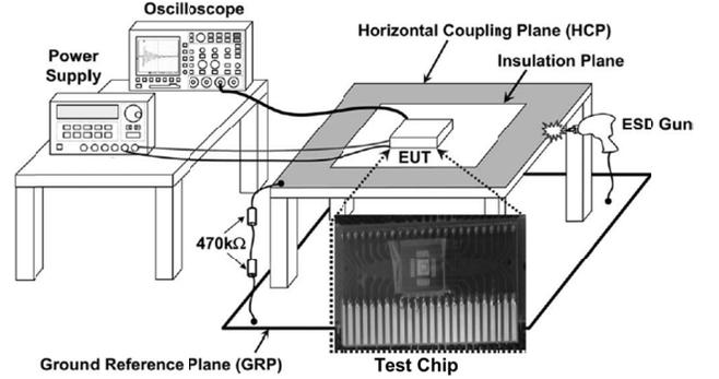
Fig. 7. Measurement setup for a system-level ESD test with indirect contact-discharge test mode [15].
