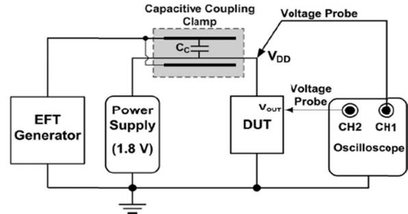
Fig. 10. Measurement setup for an EFT test combined with a capacitive coupling clamp.
