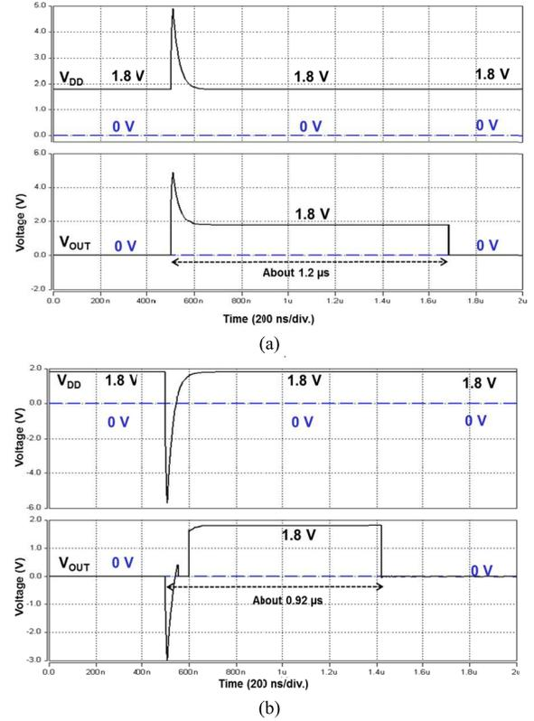
Fig. 4. Simulated  $V_{DD}$  and  $V_{OUT}$  waveforms of the new proposed on-chip self-reset transient detection circuit under EFT tests with (a) positive and (b) negative exponential voltages pulse coupled to  $V_{DD}$ .
