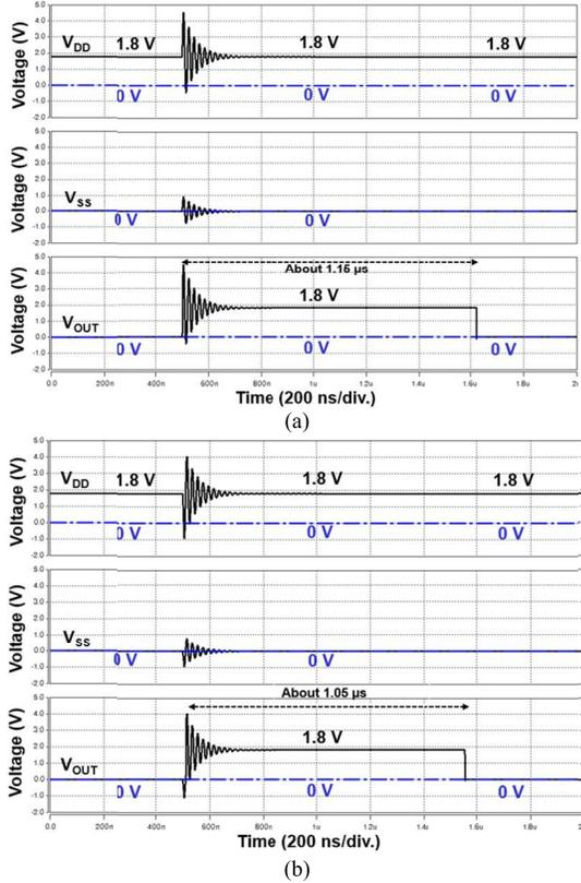
Fig. 3. Simulated  $V_{DD}$ ,  $V_{SS}$ , and  $V_{OUT}$  waveforms of the new proposed on-chip self-reset transient detection circuit under system-level ESD tests with (a) positive-going and (b) negative-going underdamped sinusoidal voltages.
