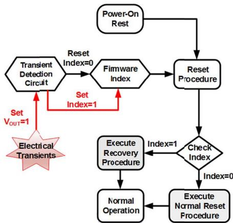
Fig. 14. Firmware flowchart combined with the self-reset transient detection circuit to recover system when electrical transients happen.
