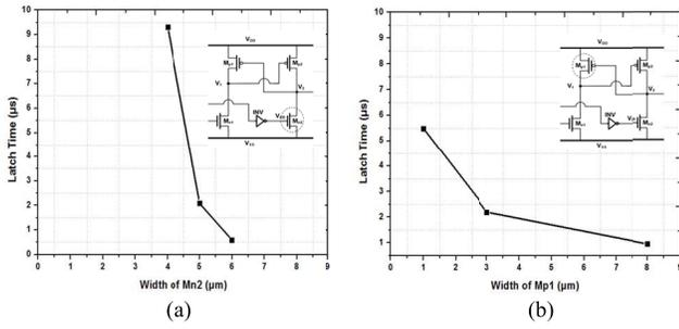
Fig. 5. Relations between latch time and (a) width of  $M_{n2}$ , (b) width of  $M_{p1}$ . The channel lengths of  $M_{n2}$  and  $M_{p1}$  are fixed at  $0.18 \mu\text{m}$ .
