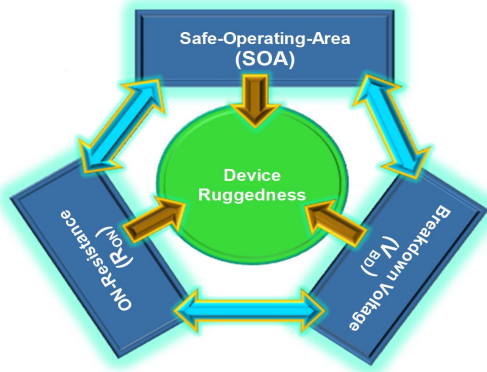
Fig. 1. Correlation between the device ruggedness and related trade-offs with ON-resistance, the BV, and the SOA.
