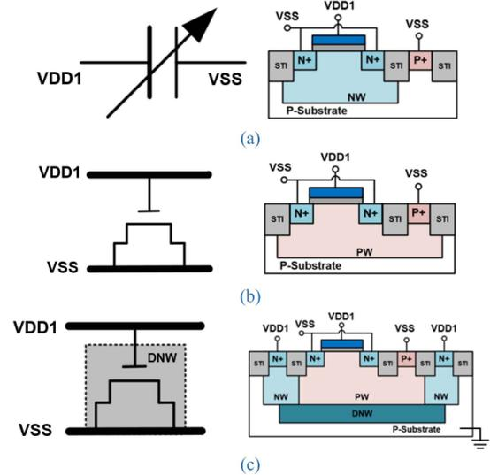
**FIGURE 6.** The symbols and cross-sectional views of (a) varactor, (b) NMOS capacitor, and (c) NMOS capacitor with DNW.
