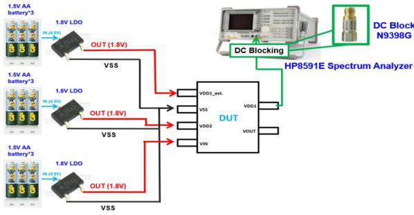
**FIGURE 13.** The setup to measure the power line noise spectrum by the spectrum analyzer. The DUT is powered by the clean 1.8-V voltage sources those generated from the standalone batteries with 1.8-V LDO regulators. The VDD1 pin is connected through a DC blocking component into the spectrum analyzer to observe the noise spectrum waveform on the VDD1 power line.
