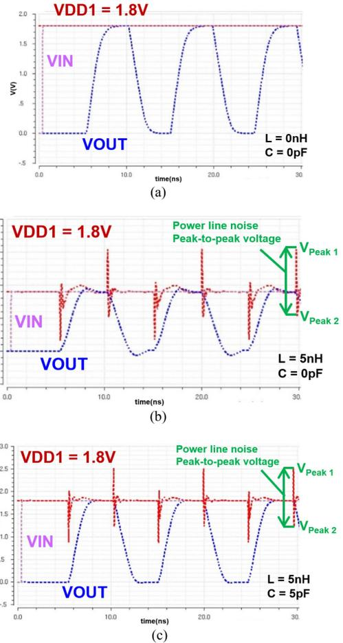
**FIGURE 2.** Simulation results of the test circuit (a) without parasitic inductance, (b) with parasitic inductance of 5nH, and (c) with parasitic inductance of 5nH and decoupling capacitor of 5pF. Power line noise induced by the parasitic inductance can be suppressed by decoupling capacitor (the output freq. of ring oscillator is 97MHz).
