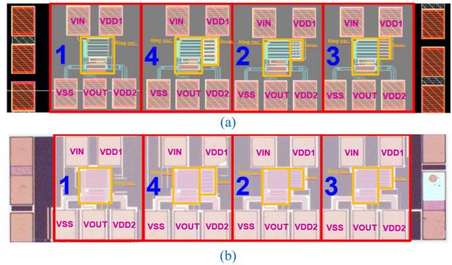
**FIGURE 7. The illustrations of (a) layout top view and (b) optical microscope (OM) micrograph of the test circuits in a silicon chip. The numbers on the illustration are corresponding to the symbol numbers of test circuits in Table 2. The additional pad pairs at two sides are specially designed to extend the length of bonding wire for testing with the increased parasitic inductance.**
