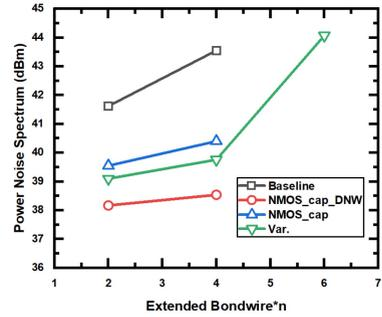
**FIGURE 15.** Comparisons among the measured power line noise spectrums on the four test circuits without or with different decoupling capacitors under different lengths of bonding wires.
