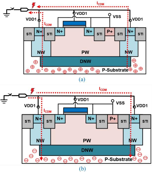
**FIGURE 20.** Cross-sectional view of the decoupling capacitor realized by NMOS capacitor with DNW during (a) positive, and (b) negative, CDM ESD stressing on VDD1 pin. The CDM ESD current is discharged through the parasitic junction that formed between P-substrate and the DNW to result in a higher CDM ESD robustness.
