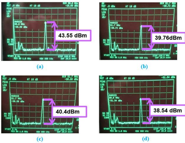
**FIGURE 14.** The measured spectrum waveforms on the VDD1 power lines of the test circuits, (a) without decoupling capacitor, with decoupling capacitors of (b) varactor, (c) NMOS capacitor, and (d) NMOS capacitor with DNW. The x-axis represents frequency, and the y-axis represents power spectrum. The peak tones of power line noise on VDD1 are all located at 81 MHz.
