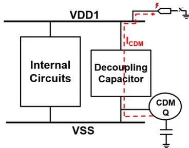
**FIGURE 4.** The illustration to show CDM ESD current path that will be concentrated to flow through the decoupling capacitor during CDM ESD events, especially when the CDM ESD is discharging from the power pin (VDD1) of internal circuits.
