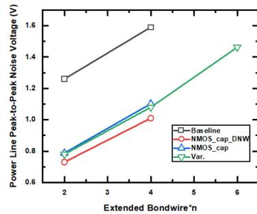
**FIGURE 12.** Comparisons among the measurement results of four test circuits without or with different decoupling capacitors under different lengths of bonding wires.
