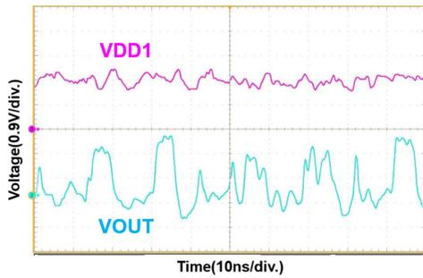
**FIGURE 19.** The measured voltage waveform of VOUT in the test circuit with decoupling capacitor of varactor after CDM ESD stress of  $-250\text{V}$ , the output function is incorrect.
