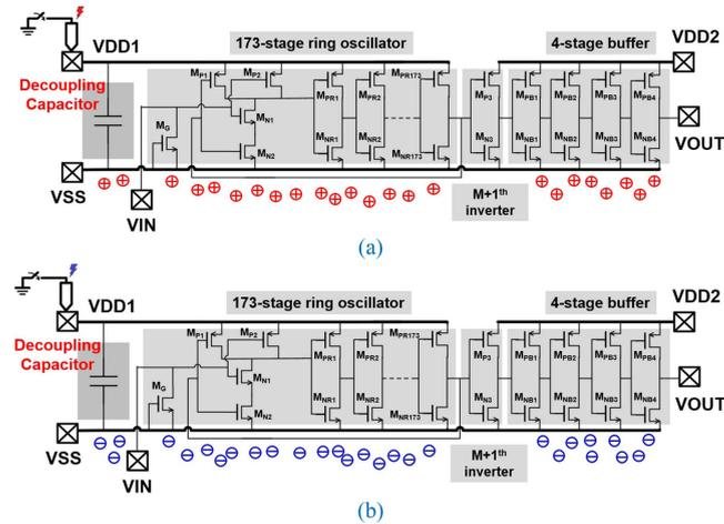
**FIGURE 17.** Schematic diagrams to illustrate CDM ESD discharging on the VDD1 pin of the test chip under (a) positive, and (b) negative, CDM ESD polarities.
