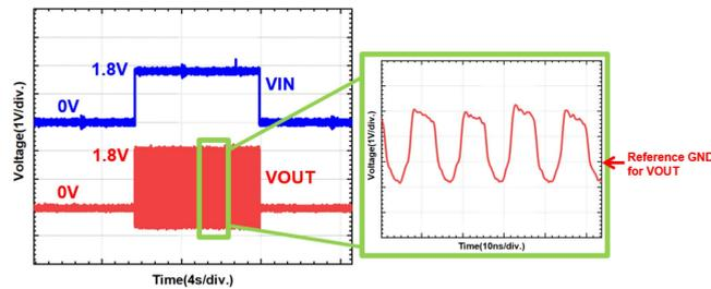
**FIGURE 10.** Function verification on the fabricated test circuits. The ring oscillator starts to generate the clock-like output waveform (VOUT), when the input signal (VIN) is switched from 0V to 1.8V.
