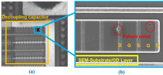
**FIGURE 22.** Failure analysis results of the ring oscillator with decoupling capacitor of the varactor. The (a) EFA and (b) SEM results after +500V CDM stress on the VDD1 pin are shown.
