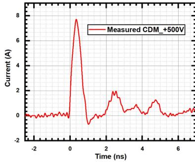
**FIGURE 3.** Measured CDM ESD current waveform (+500V) from the device under test (DUT) with an equivalent capacitance of 41 pF. The current reaches 7.68A within 275ps, and the main current pulse is within ~1 ns.
