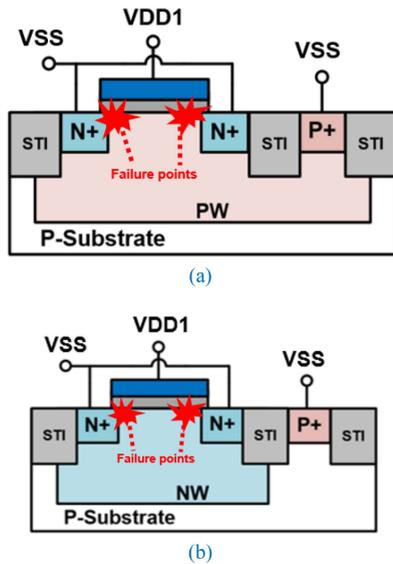
**FIGURE 23.** Cross-sectional view to illustrate the failure location on the gate oxide of (a) NMOS capacitor and (b) varactor, after the CDM ESD stress.
