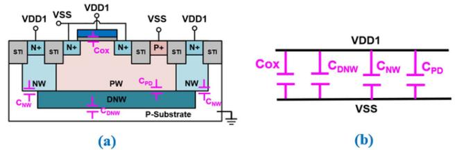
**FIGURE 16.** (a) The cross-sectional view of the NMOS capacitor with DNW, and (b) the equivalent circuit to show the total capacitance between power lines.
