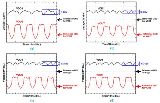
**FIGURE 11.** The measured voltage waveforms on VDD1 and VOUT of the test circuits (a) without decoupling capacitor, (b) with decoupling capacitor of the varactor, (c) with decoupling capacitor of NMOS, and (d) with decoupling capacitor of NMOS with DNW.
