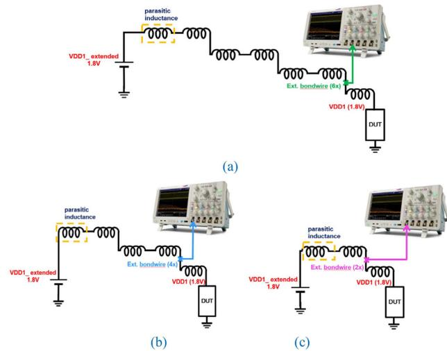
**FIGURE 9.** Measurement setups for observing the power line noise induced by (a) 6x extending bonding wires, (b) 4x extending bonding wires, and (c) 2x extending bonding wires, through VDD1 pin on IC and VDD1\_extended pin on the package.
