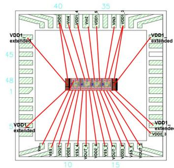
**FIGURE 8. Wire bonding plan for the fabricated silicon chip with the test circuits. Bonding two wires in series to the pin of IC to extend the length of bonding wire for testing with increased inductance through the VDD1\_extended pin.**
