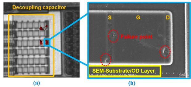
**FIGURE 21.** Failure analysis results of the ring oscillator with decoupling capacitor of NMOS capacitor. The (a) EFA and (b) SEM results after  $-500\text{V}$  CDM stress on the VDD1 pin are shown.
