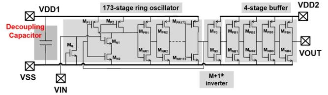
**FIGURE 5.** The ring oscillator of 173-stage inverter chain with decoupling capacitor was used as the internal circuits of test chip for CDM ESD study, which was designed and fabricated in a 0.18- $\mu$ m 1.8V CMOS process.
