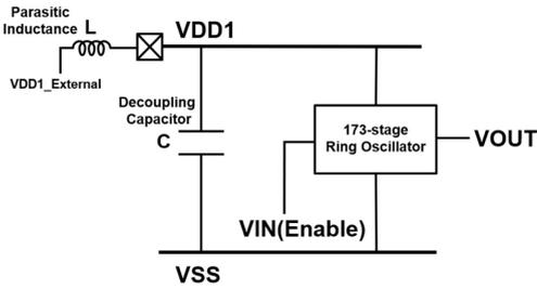
**FIGURE 1.** Block diagram of the test circuit and the parasitic inductance induced by the bonding wire. The test circuit includes a ring oscillator of 173-stage inverter chain and a decoupling capacitor.
