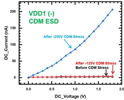
**FIGURE 18.** DC I-V characteristics on VDD1 of the test circuit with decoupling capacitor of varactor before and after CDM ESD stress.
