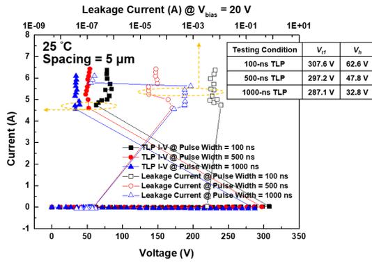
Fig. 4.  $I$ - $V$  curves of the TLP measurement with the pulsewidth of 100, 500, and 1000 ns, respectively.
