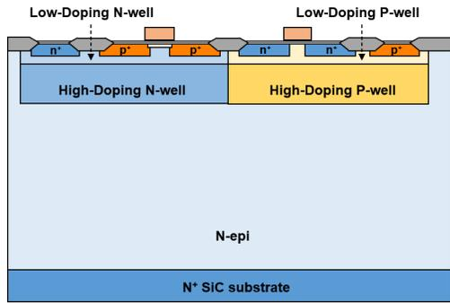
Fig. 9. Schematic of the CMOS structure with retrograde well.
