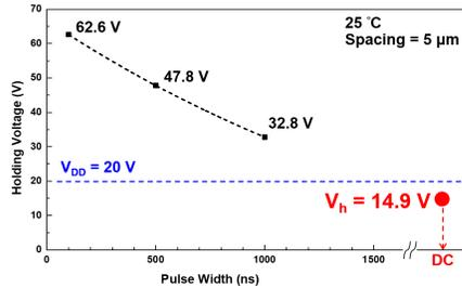
Fig. 5. Correlation between TLP pulsewidth, dc measurement, and holding voltage ( $V_h$ ).
