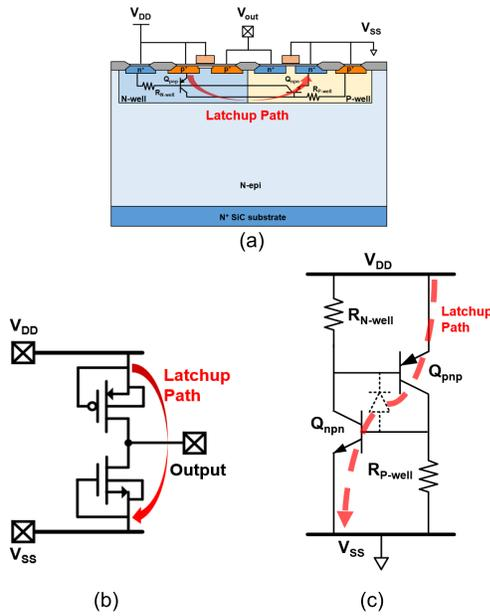
Fig. 1. (a) Cross-sectional view, (b) schematic, and (c) parasitic SCR structure with its corresponding latchup path in the CMOS structure.
