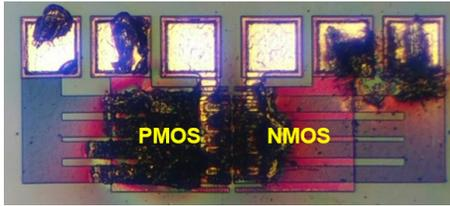
Fig. 6. Die image of the latchup failure photographed by the optical microscope.
