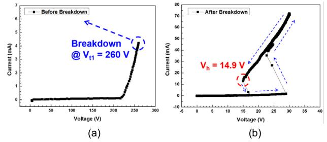
Fig. 3.  $I-V$  curves (a) measured by the curve tracer before the device breakdown and (b) remeasured by the curve tracer after the device breakdown.
