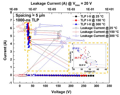
Fig. 7.  $I$ - $V$  curves of the TLP measurement at 25 °C, 150 °C, and 300 °C, respectively.
