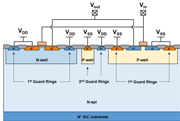
Fig. 10. Schematic of the CMOS structure surrounded by double guard rings.
