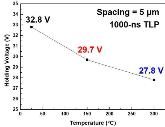
Fig. 8. Correlation between temperature and holding voltage ( $V_h$ ).
