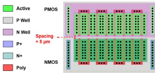
Fig. 2. Layout view of the CMOS structure with GDPMOS and GGNMOS.
