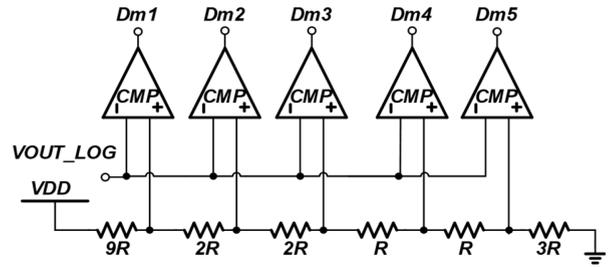
**FIGURE 3.** Circuit view of magnitude discriminator in the ESD event detector.
