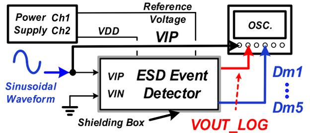
FIGURE 8. Measurement testbench for magnitude discriminator.
