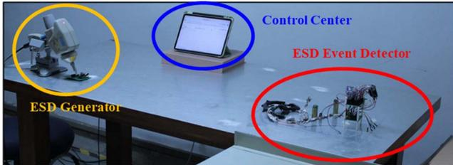
**FIGURE 22.** Experimental setup for ESD event detector field application.
