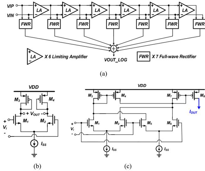
**FIGURE 2.** (a) Block diagram of the logarithmic amplifier, (b) circuit of limiting amplifier (LA), and (c) circuit of full-wave rectifier (FWR).
