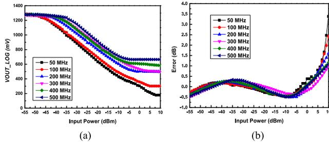
FIGURE 7. Measurement results of the logarithmic amplifier (a) responses vs. input power and (b) error vs. input power at different frequencies.
