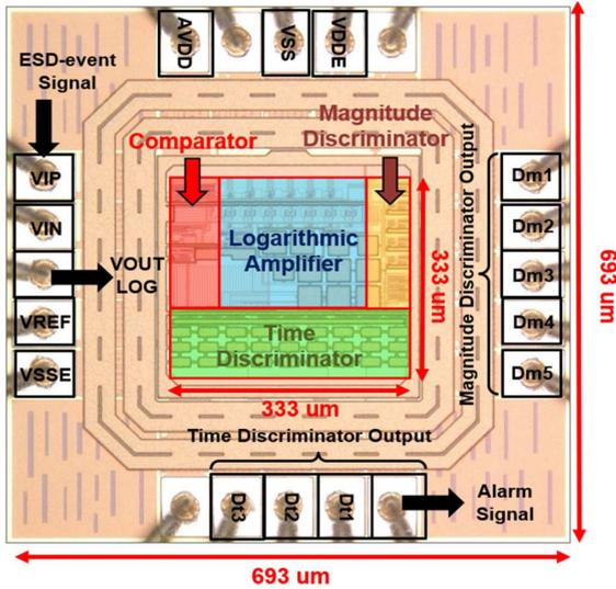
FIGURE 6. Die microphotograph of the proposed ESD event detector.
