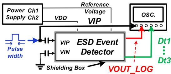
FIGURE 10. Measurement testbench for time discriminator.
