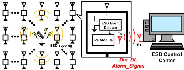
**FIGURE 21.** Multiple ESD event detectors can be positioned around IC manufacturing environments. Once an ESD event occurs, the RF Wi-Fi module on each ESD event uploads the information to the ESD control center.
