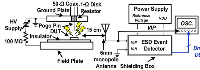
FIGURE 19. Schematic of the experimental setup for the ESD field test with the Onion3 CDM Tester with antenna 15 cm away from the Pogo pin zapping point.
