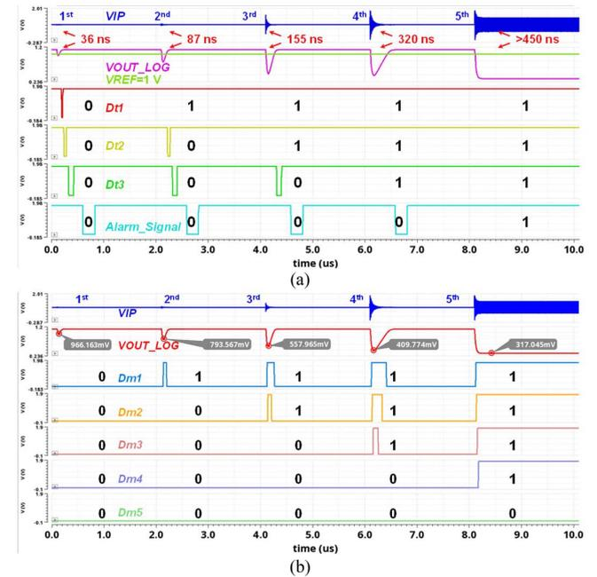
**FIGURE 5.** Simulation result of (a) time discriminator and (b) magnitude discriminator.
