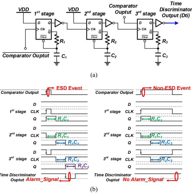
**FIGURE 4.** (a) Circuit view of time discriminator and (b) output waveform analysis.
