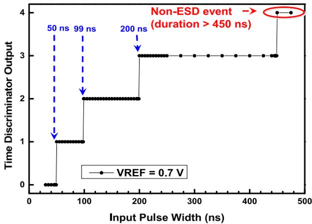
**FIGURE 12. Time discriminator output vs. input pulse duration.**
