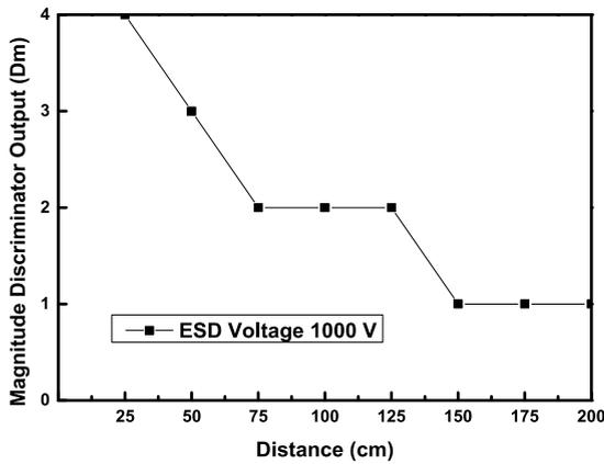
**FIGURE 15.** Relationship between the magnitude discriminator output and the distance from the zapping point of the ESD generator to the antenna with an ESD voltage of 1000 V.
