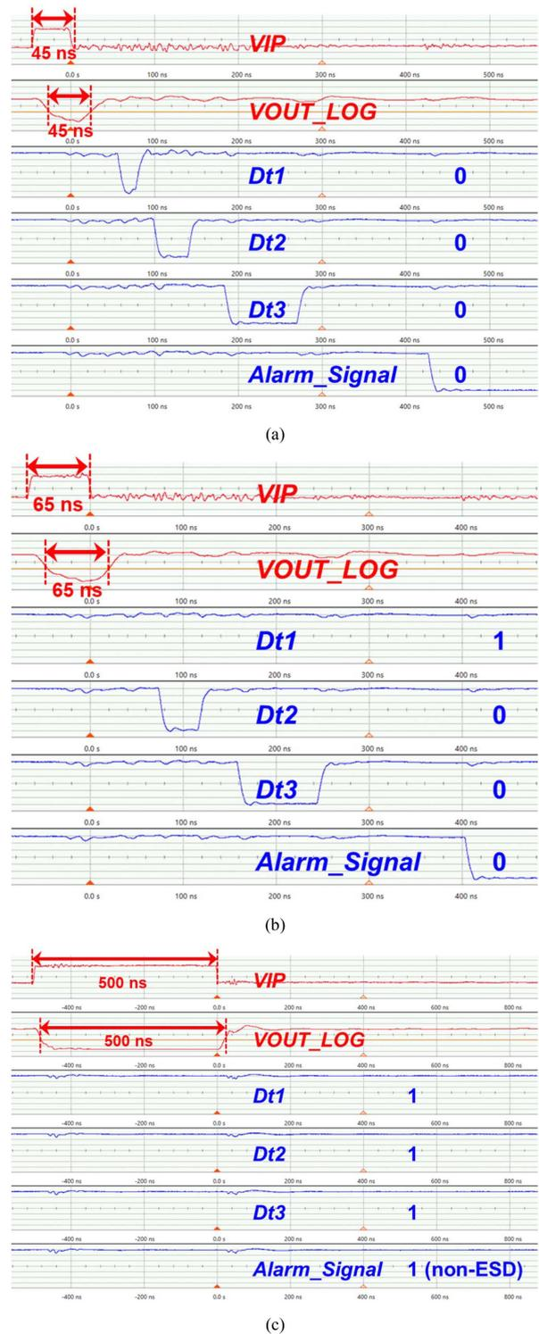
FIGURE 11. Measured results of the time discriminator with the input pulse of 60 mV,  $V_{REF}=0.7$  V, and the pulse duration (a) 45 ns, (b) 65 ns, and (c) 500 ns.
