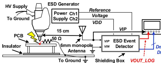
**FIGURE 13. Experimental setup for ESD field test with the IEC ESD generator.**
