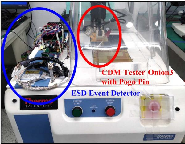
FIGURE 18. Experimental setup for ESD field test with the Onion3 CDM Tester.
