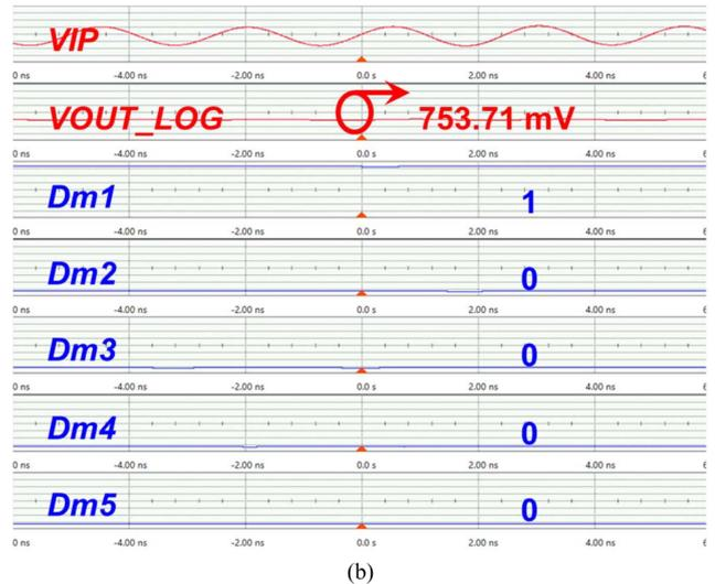
FIGURE 9. Measured results of the magnitude discriminator with (a) input power  $-10$  dBm and (b) input power  $-15$  dBm, under  $400$  MHz operating frequency.
