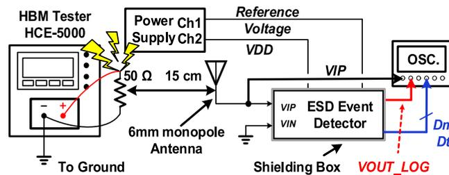
**FIGURE 16.** Experimental setup for ESD field test with HBM Tester HCE-5000.
