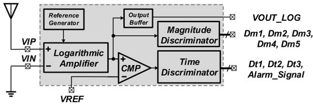
**FIGURE 1.** Block diagram of the new proposed ESD-event detector.
