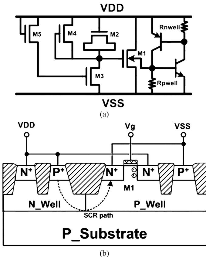
Fig. 7. (a) Power-rail ESD clamp circuit with the hot-carrier triggered SCR (HCTSCR) device. (b) Device structures of primary protection devices including SCR and nMOS M1.
