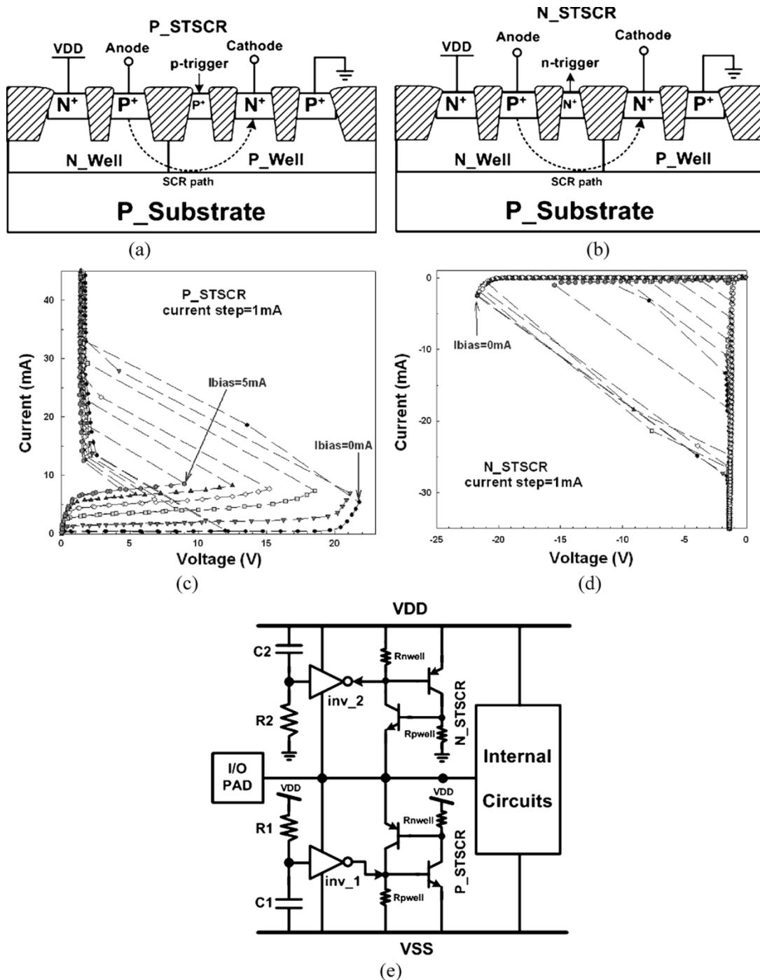
Fig. 9. Device structures of (a) the p-type substrate-triggered SCR (P-STSCR) and (b) the n-type substrate-triggered SCR (N-STSCR) devices. The  $I$ - $V$  characteristics of (c) the P-STSCR and (d) the N-STSCR devices in a  $0.25\text{-}\mu\text{m}$  CMOS process. (e) The ESD protection circuit with the P-STSCR and N-STSCR devices for I/O pad.
