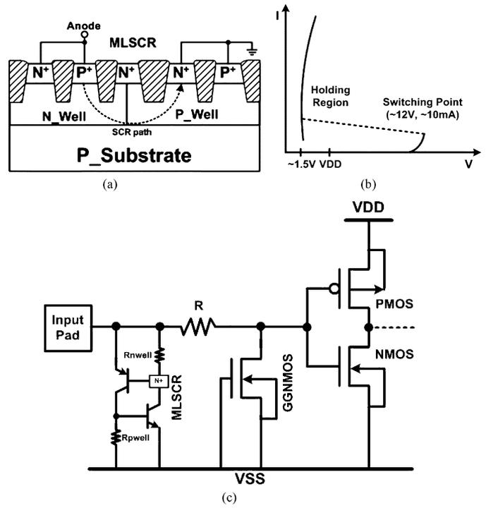
Fig. 4. (a) Device structure of the modified LSCR (MLSCR) in CMOS process. (b)  $I$ - $V$  characteristics of the MLSCR in a  $0.25\text{-}\mu\text{m}$  CMOS process. (c) Input ESD protection circuit with the MLSCR device.
