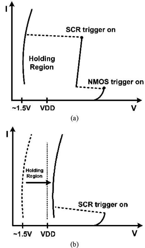
Fig. 14. Two solutions to overcome latchup issue in the ESD protection design with SCR-based device: (a) increasing the trigger current and (b) increasing holding voltage to avoid the SCR-based devices being accidentally triggered on by noise pulse.
