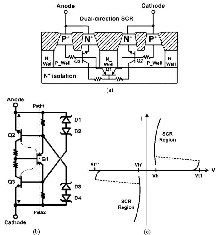
Fig. 13. (a) Device structure of the dual-direction SCR. (b) Circuit schematic of the low-trigger-voltage ESD protection circuit consists of a core dual-direction SCR and two back-to-back Zener diodes. (c)  $I$ - $V$  characteristics of the dual-direction SCR device.
