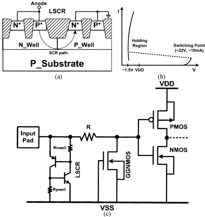
Fig. 3. (a) Device structure of the lateral SCR (LSCR) in CMOS process. (b)  $I$ - $V$  characteristics of the LSCR in a  $0.25\text{-}\mu\text{m}$  CMOS process. (c) Input ESD protection circuit with the LSCR device.
