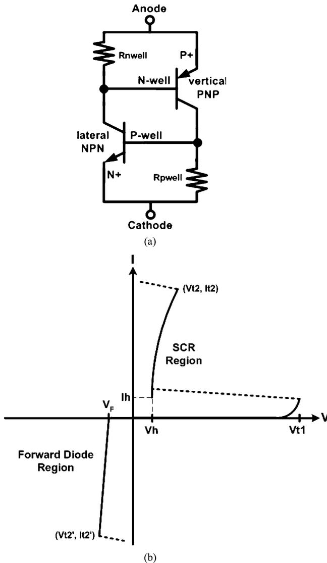
Fig. 2. (a) Equivalent circuit schematic of a SCR device. (b)  $I$ - $V$  characteristics of SCR device in CMOS process under positive and negative voltage biases.
