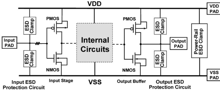
Fig. 1. Typical design of on-chip ESD protection circuits in CMOS ICs.
