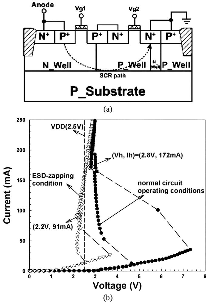
Fig. 15. (a) Device structure of dynamic holding voltage SCR (DHVSCR) in CMOS process. (b)  $I$ - $V$  characteristics of the DHVSCR under normal circuit operating conditions and ESD-zapping conditions in a  $0.25\text{-}\mu\text{m}$  CMOS process.
