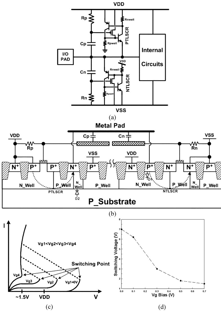
Fig. 6. (a) ESD protection circuit with the gate-coupled LVTSCR devices. (b) Device structure of the gate-coupled LVTSCR device in CMOS process. (c)  $I-V$  characteristics of the gate-coupled LVTSCR device in a  $0.25\text{-}\mu\text{m}$  CMOS process. (d) Dependence of switching voltage of SCR device on the gate bias voltage of the NTLSCR device.
