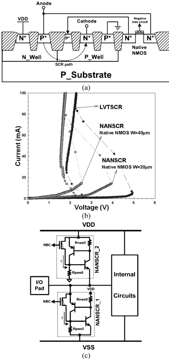
Fig. 11. (a) Device structure of the native-NMOS-triggered SCR (NANSCR). (b) Comparison of DC  $I$ - $V$  curves between NANSCR and LVTSCR in a  $0.13\text{-}\mu\text{m}$  CMOS process. (c) ESD protection circuit with the NANSCR device.
