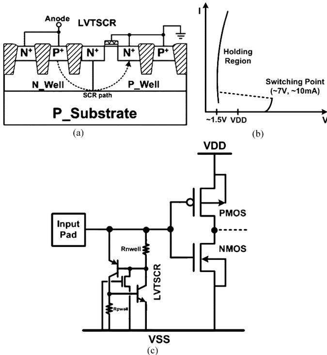
Fig. 5. (a) Device structure of the low-voltage triggering SCR (LVTSCR) in CMOS process. (b)  $I$ - $V$  characteristics of the LVTSCR in a  $0.25\text{-}\mu\text{m}$  CMOS process. (c) Application example of input ESD protection circuit with the LVTSCR device.
