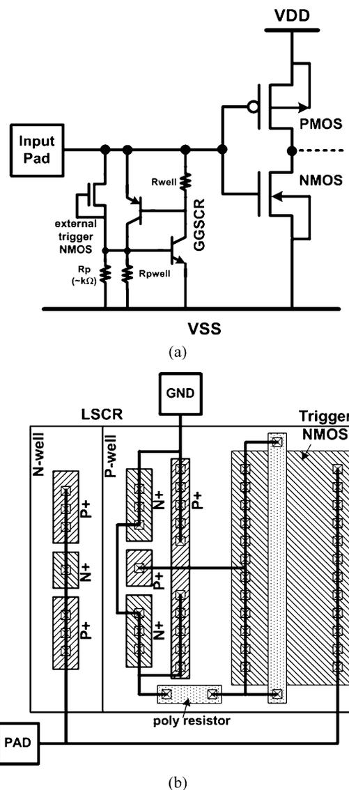
Fig. 8. (a) Input ESD protection circuit with the grounded-gate nMOS triggered SCR (GGSCR) device. (b) Layout top view of the GGSCR in a CMOS process.
