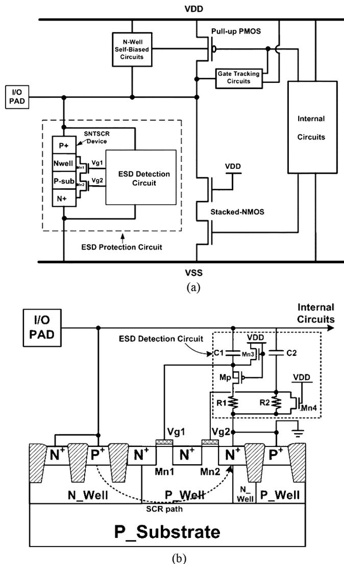
Fig. 12. (a) ESD protection circuit with stacked-NMOS triggered SCR (SNTSCR) device for mixed-voltage I/O interface. (b) ESD detection circuit and the device structure of the SNTSCR.
