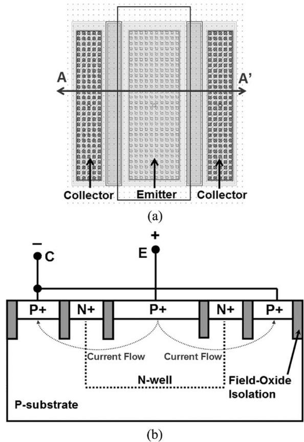
Fig. 7. (a) Single-finger layout style of the LVTp-n-p, and (b) cross-sectional view along the line AA' in the single-finger layout of LVTp-n-p.
