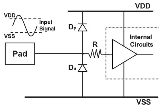
Fig. 1. Input signals with voltage levels higher than VDD and lower than VSS in some mixed-voltage I/O interfaces.
