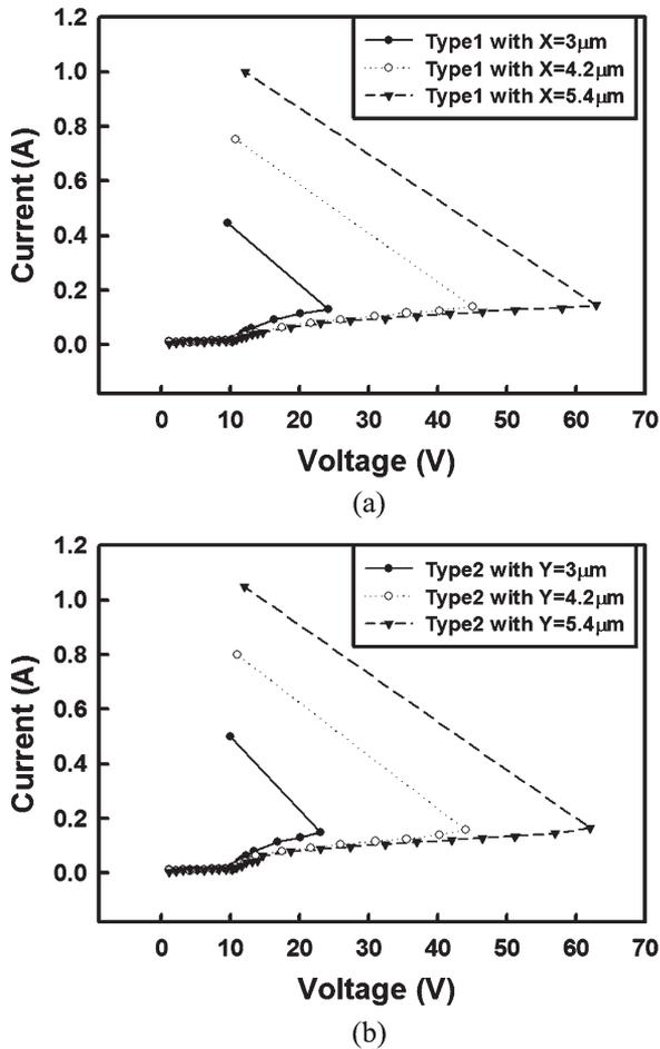
Fig. 6. TLP-measured  $I-V$  curves of (a) the type1 LVTp-n-p with different  $X$  spacings, and (b) the type2 LVTp-n-p with different  $Y$  spacings, under the positive-to-VSS stress condition.
