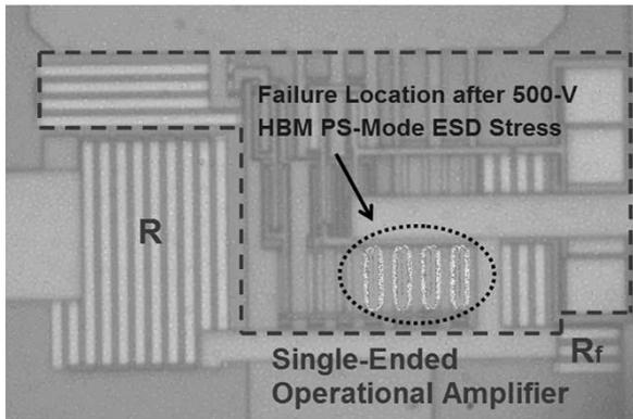
Fig. 13. EMMI picture on the ADSL input stage without ESD protection circuit after HBM PS-mode ESD stress of 500 V.
