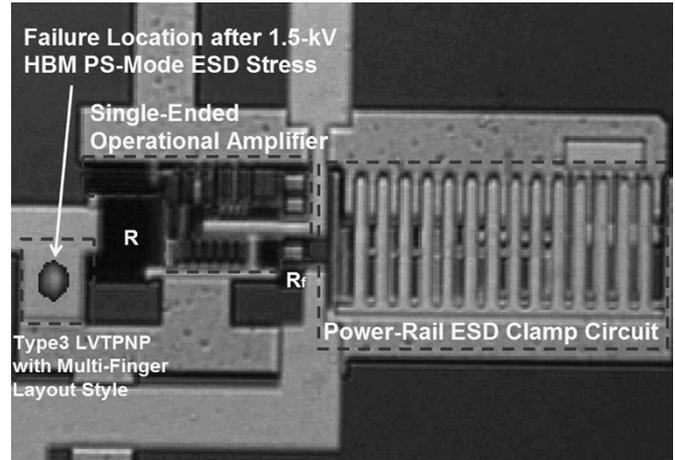
Fig. 14. OBIRCH picture on the ADSL input stage with ESD protection circuit after 1.5-kV HBM PS-mode ESD stress. The failure location is on the type3 LVTPNP device of the ESD protection circuit.
