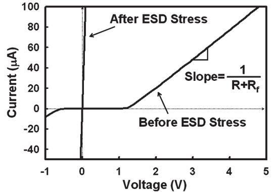
Fig. 12.  $I$ - $V$  curves of the ADSL input stage with ESD protection circuit before and after PS-mode HBM ESD stress of 1.5 kV, which was measured by applying a swept voltage from  $-1$  to  $5$  V on the input pad with  $V_{SS}$  grounded and  $V_{DD}$  floating.
