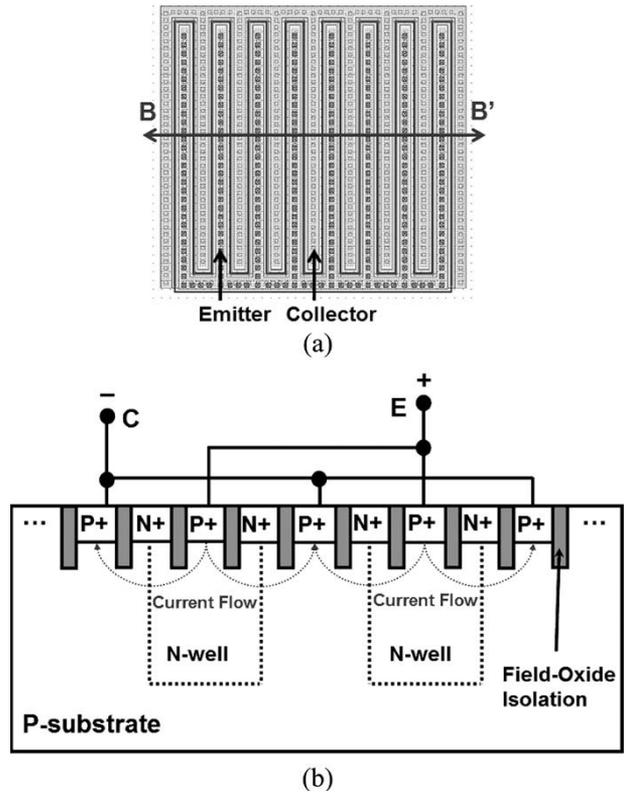
Fig. 8. (a) Multifinger layout style of the LVTp-n-p, and (b) cross-sectional view along the line BB' in the multifinger layout of LVTp-n-p.
