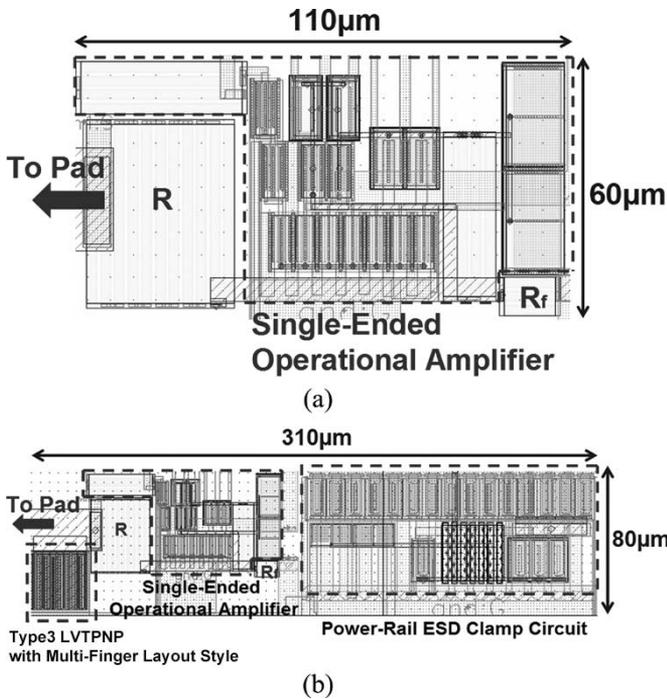
Fig. 11. Layout views of the ADSL input stage (a) without ESD protection, and (b) with ESD protection circuit.
