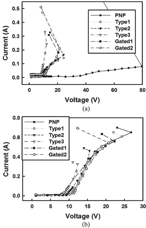
Fig. 4. TLP-measured  $I$ - $V$  curves among traditional p-n-p and different LVTp-n-p devices under (a) the positive-to-VSS (PS-mode), and (b) the negative-to-VSS (NS-mode) stress conditions.
