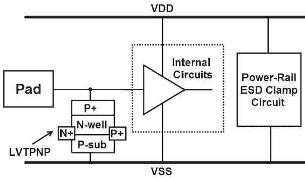
Fig. 2. New proposed ESD protection design with LVTp-n-p device for the mixed-voltage I/O interface with input voltage levels higher than VDD and lower than VSS.
