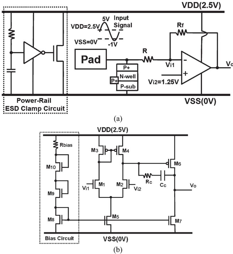
Fig. 10. (a) ESD protection design for the ADSL input stage with single-ended opamp and voltage divider in a 0.25- $\mu\text{m}$  salicided CMOS process. (b) Schematic of the two-stage opamp.
