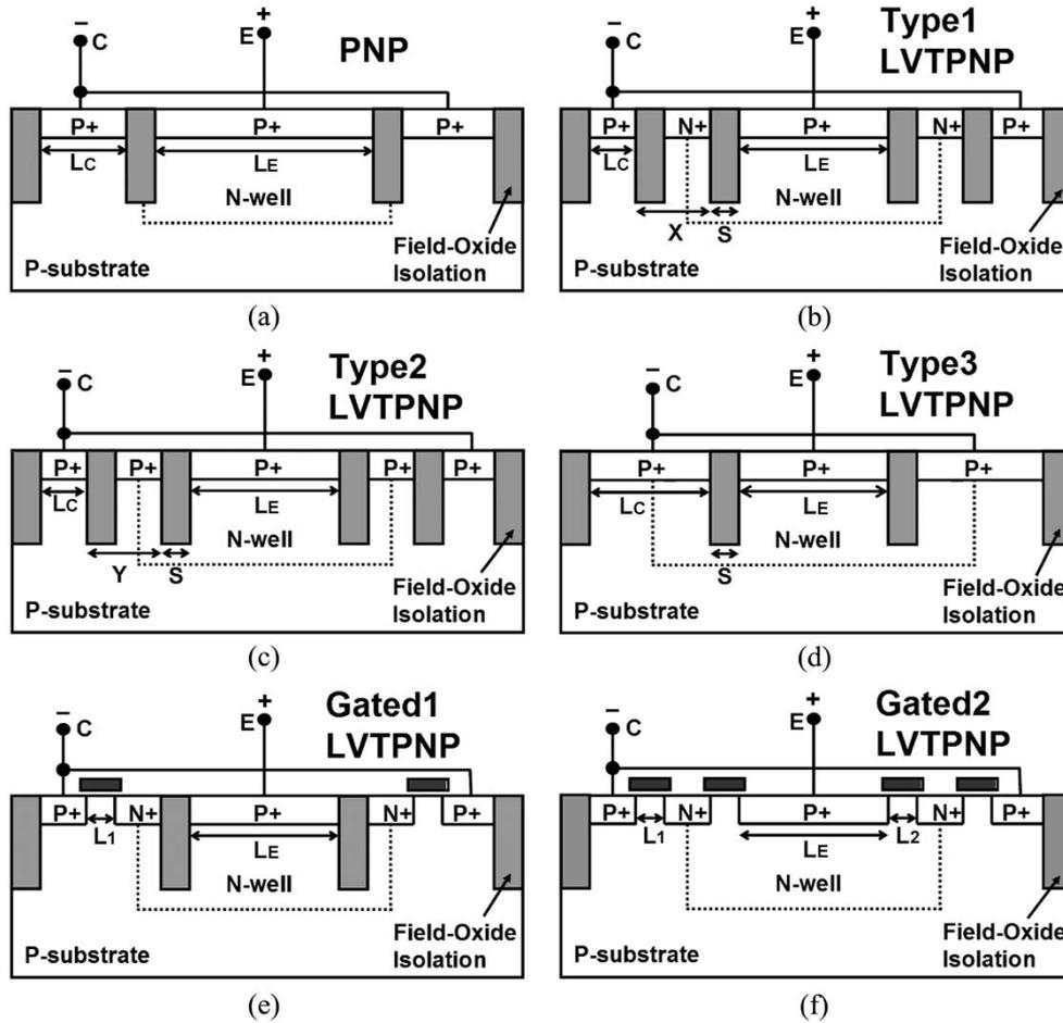
Fig. 3. Device structures of (a) the traditional p-n-p, (b) the type1 LVTp-n-p, (c) the type2 LVTp-n-p, (d) the type3 LVTp-n-p, (e) the gated1 LVTp-n-p, and (f) the gated2 LVTp-n-p.
