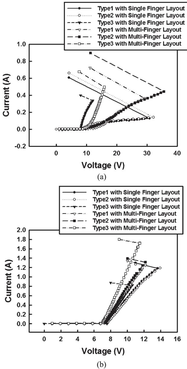
Fig. 9. TLP-measured  $I-V$  curves of the LVTp-n-p devices realized with the single-finger layout style or the multifinger layout style in a  $0.25\text{-}\mu\text{m}$  salicided CMOS process under (a) the positive-to-VSS, and (b) the negative-to-VSS stress conditions.
