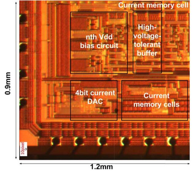
Fig. 12. Die photo of the fabricated stimulator.
