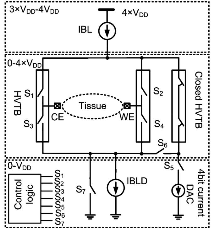
Fig. 2. Block schematic of the proposed neuro-stimulator.
