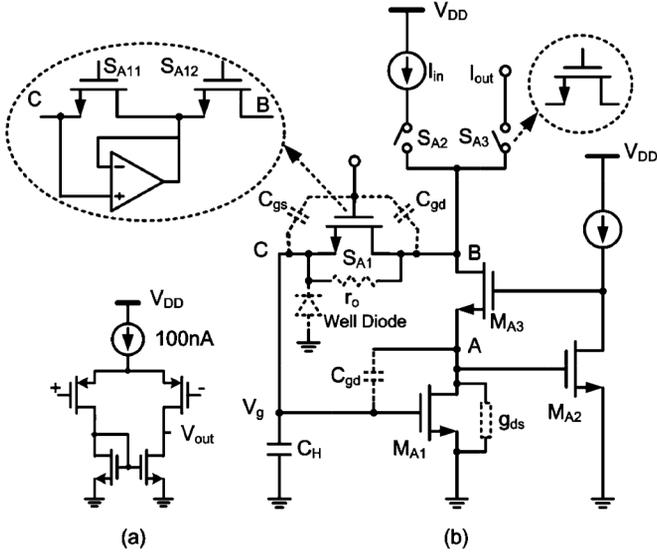
Fig. 5. (a) Basic current memory cell with leakage current compensation. (b) The simple schematic of the amplifier.
