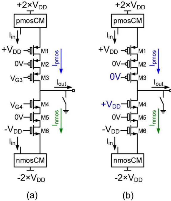
Fig. 1. (a) Stimulator using stacked LV transistors reported in [25]. (b) The stimulator with bias voltages during anodic phase.
