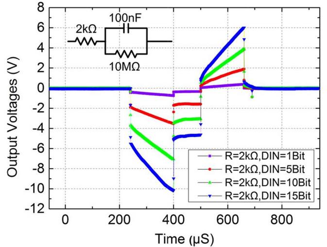
Fig. 13. Output voltages measured with different stimulus currents. The upper inset shows the equivalent circuit with quasi-static loss model.
