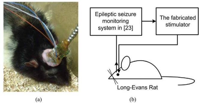
Fig. 18. (a) The Long-Evans Rat with implanted electrodes for detection and stimulation. (b) Measurement setup for animal test [23].
