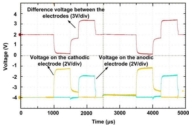
Fig. 19. The voltages on the electrodes in animal test with  $28\text{-}\mu\text{A}$  stimulus current.
