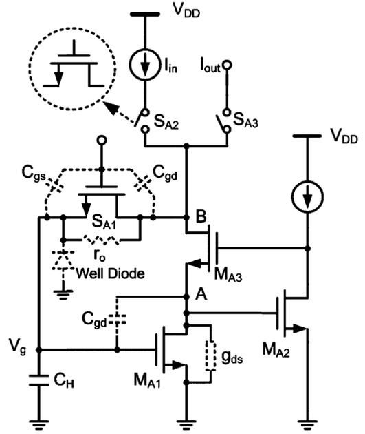
Fig. 4. Basic current memory cell with parasitic.
