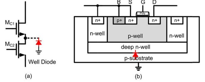
Fig. 7. (a) Principle of two stacked transistors. (b) NMOS devices with deep n-well layer and the parasitic well diode.
