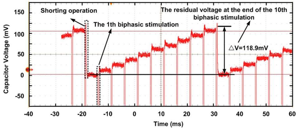
Fig. 14. An oscilloscope capture of the voltage on the 100-nF Teflon capacitor at 3000- $\mu$ A stimulus current, which allow measurements of the accumulated residual voltage at the end of the 10th biphasic stimulation.
