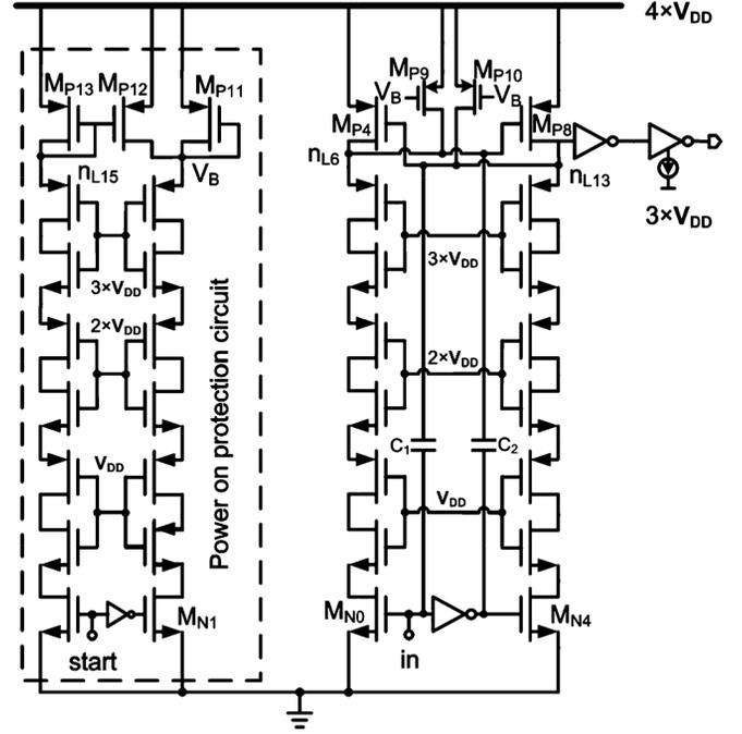
Fig. 10. High-voltage-tolerant level shifter with power-on protection.
