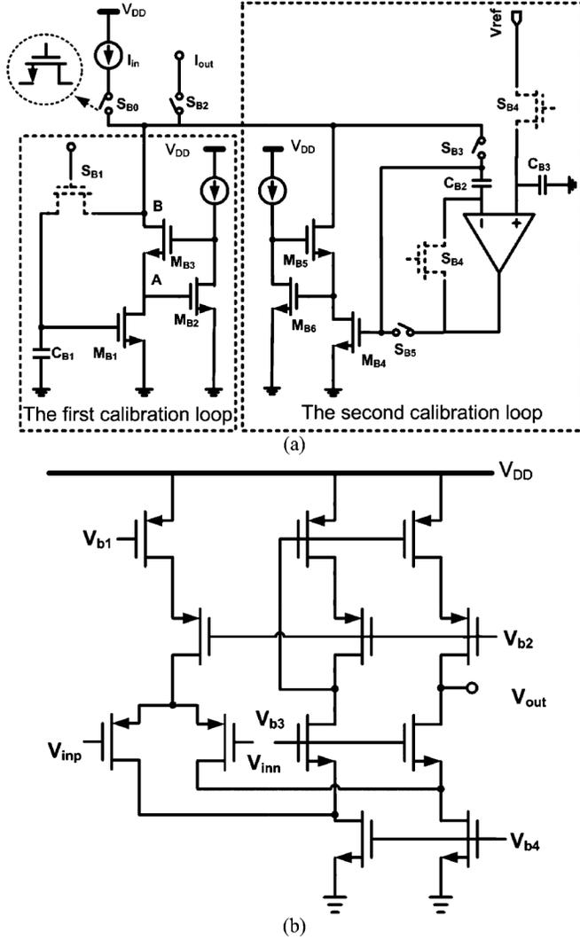
Fig. 6. (a) Basic current memory cell with leakage current compensation and dual calibration loops. (b) Differential operational amplifier.
