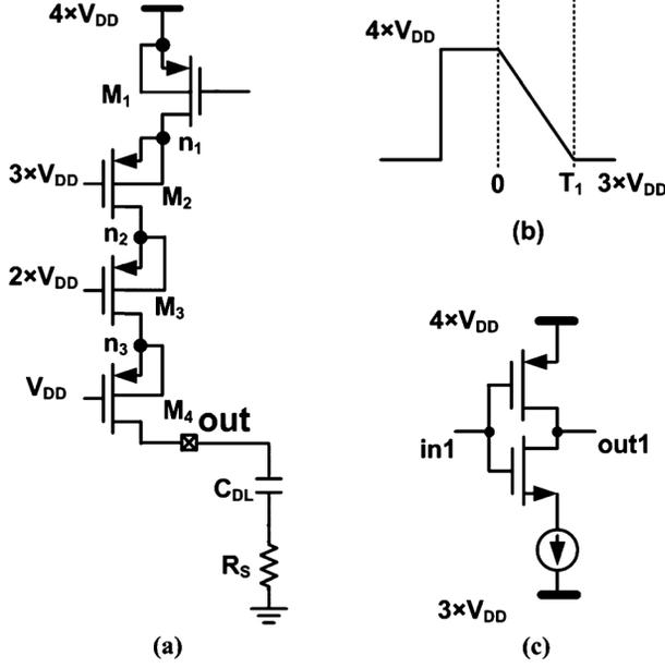
Fig. 9. (a) Simple schematic of the high-voltage-tolerant buffer with loading capacitor and resistor when it switches from 0 V to  $V_{DD}$ . (b) The gate voltage of the transistor  $M_1$ . (c) Simple schematic of driver for transistor  $M_1$ .
