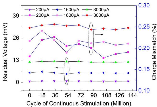
Fig. 17. Reliability measurement results under different stimulus currents as the function of continuous stimulus cycles.
