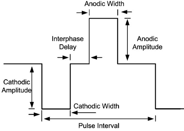
Fig. 3. Biphasic current pulse with interphase delay.
