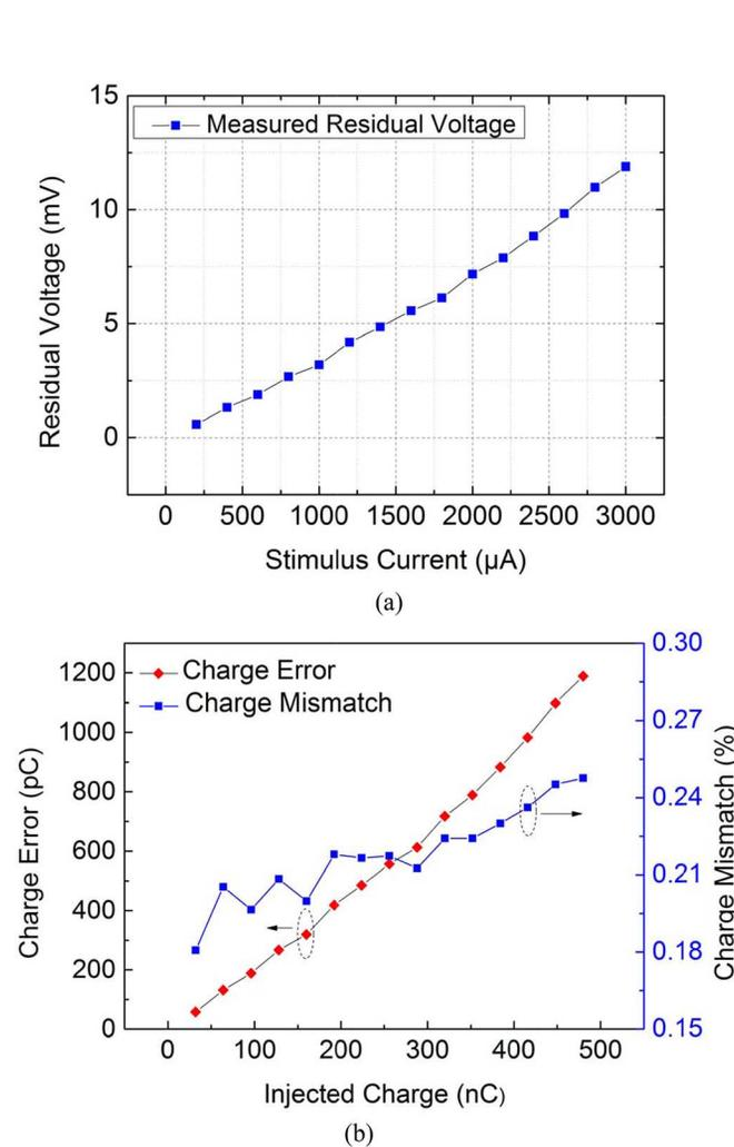
Fig. 15. (a) Residual voltage over the range of DAC current after one-cycle biphasic stimulation. (b) Charge error and charge mismatch factor as the function of injected charge.
