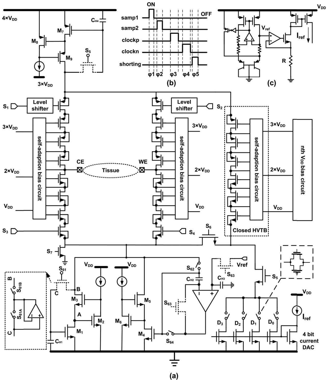
Fig. 11. (a) The fully circuit of neuro-stimulator. (b) Control signal. (c) Current reference circuit.
