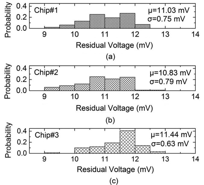
Fig. 16. The probability distribution, mean ( $\mu$ ), and standard deviation ( $\sigma$ ) of the post-stimulation residual voltage on the loading capacitor. Three chips have been measured, (a) chip #1, (b) chip #2, and (c) chip #3.
