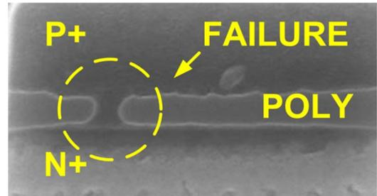
Fig. 15. FA image after vf-TLP failure of the proposed DSCR. Failure is located on  $D_2$ .
