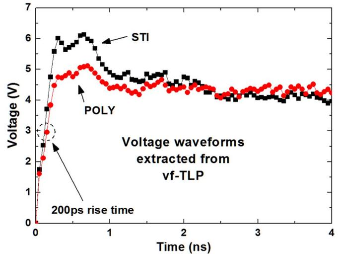
Fig. 10. Extracted voltage waveforms from vf-TLP measurements.
