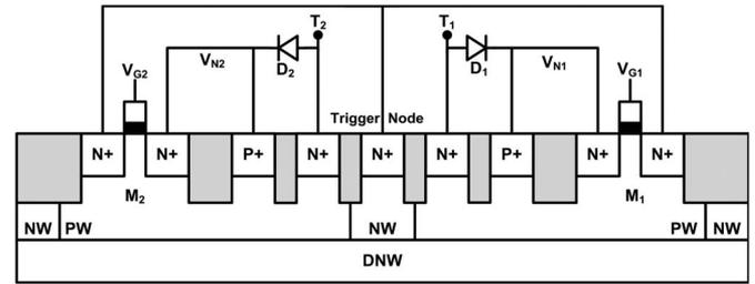
Fig. 14. Proposed modified circuit using a p-well-based DSCR structure. The connection to the RCR circuit (not shown) is identical to the one in Fig. 1(b).
