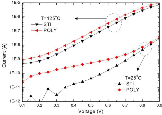
Fig. 7. Leakage current measurement for different bias voltages under controlled temperature.
