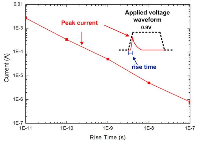
Fig. 4. Simulated peak current for a 0.9-V square pulse with different rise times.
