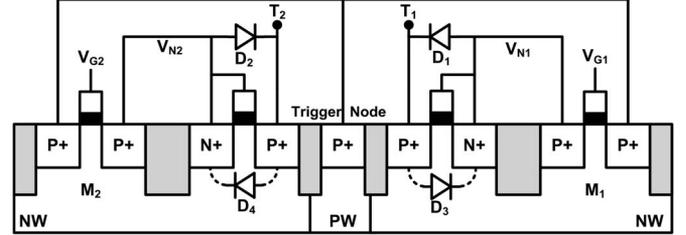
Fig. 6. Proposed DSCR structure with polybounded diodes  $D_3$  and  $D_4$ .
