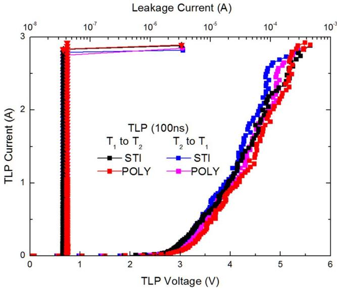
Fig. 8. TLP I-V measurement results for the implemented devices.
