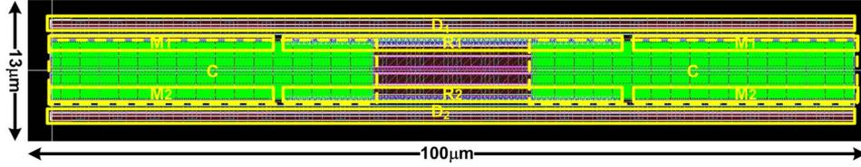
Fig. 5. Layout view of the proposed DSCR with a symmetrical trigger circuit. The total area is  $13 \mu\text{m} \times 100 \mu\text{m}$ .
