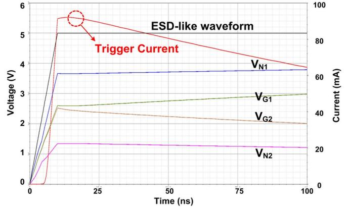
Fig. 2. Simulation result for an ESD-like waveform zapping from  $T_1$  to  $T_2$ .
