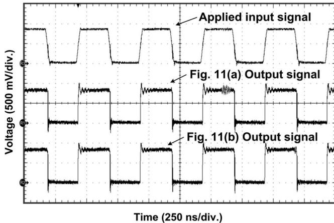
Fig. 12. Observed output waveforms of the circuits in Fig. 11 for an applied 0.9-V 2-MHz square pulse at the input pad.
