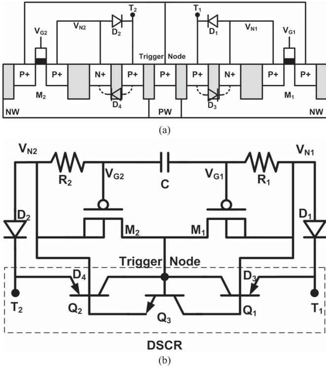
Fig. 1. Proposed DSCR structure with a symmetrical trigger circuit. (a) and (b) Device cross-sectional view and equivalent circuit, including the RCR trigger circuit, respectively.
