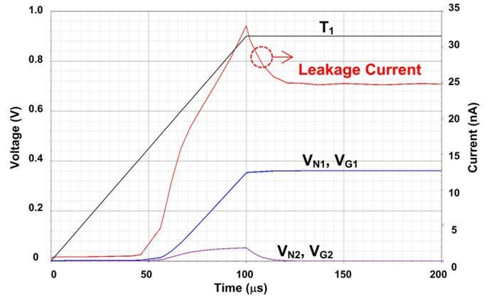
Fig. 3. Simulation result for normal circuit operation.
