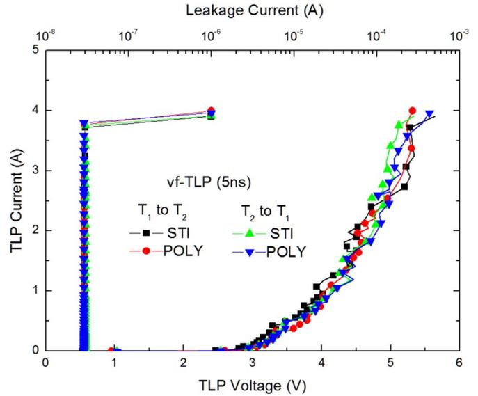
Fig. 9. vf-TLP I-V measurement results for the implemented devices.
