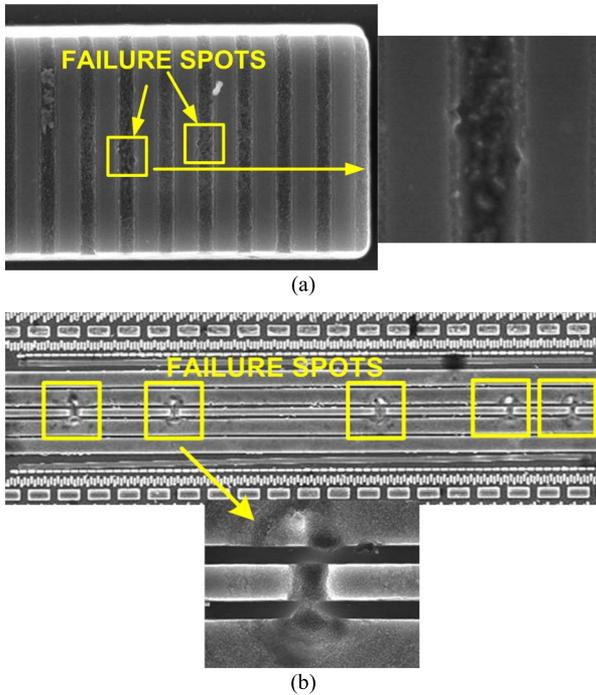
Fig. 13. (a) Failure location on the STI design after 275-V MM stress is located in the gate of the internal circuit. (b) Failure location on the POLY design after 375-V MM stress is located on the DSCR structure.
