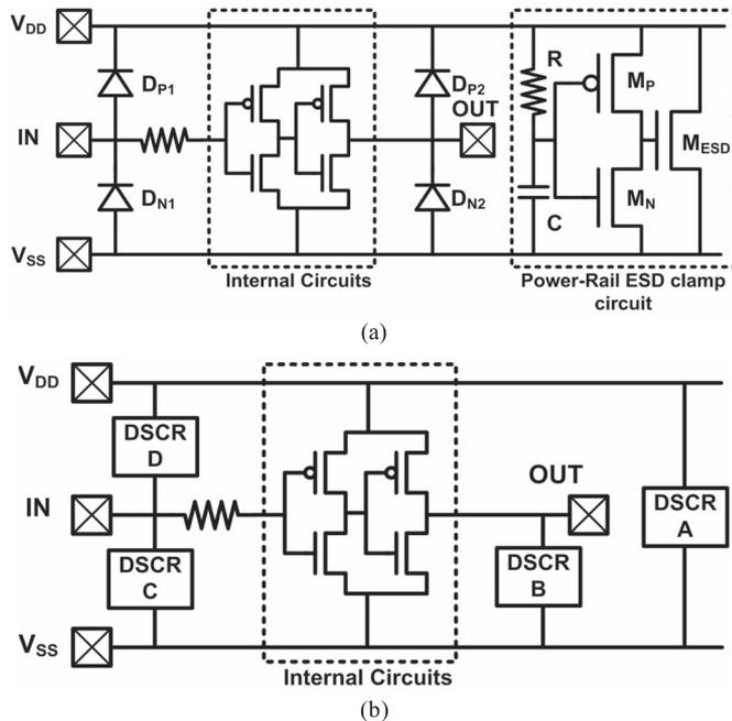
Fig. 11. Circuits used for ESD robustness measurement. (a) Circuit using the standard whole-chip ESD protection. (b) Circuit using the proposed DSCR-based whole-chip ESD protection.
