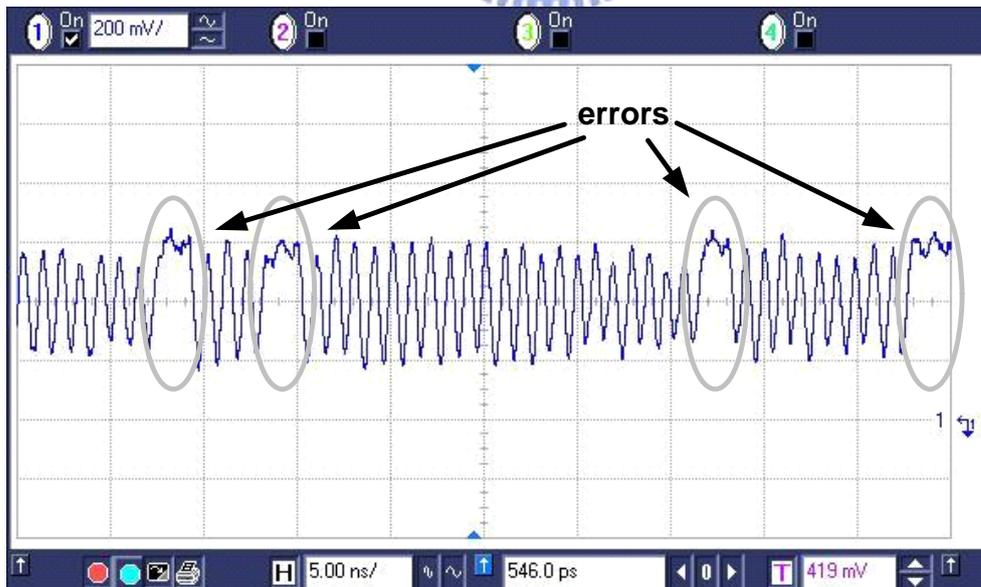
Fig. 5.9 Cyclic “010101” pattern test result at data rate up to 2 Gb/s
