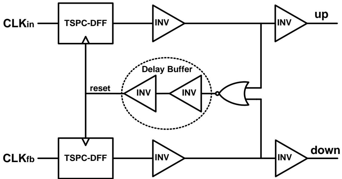
Fig. 4.19 Schematic diagram of the PFD
