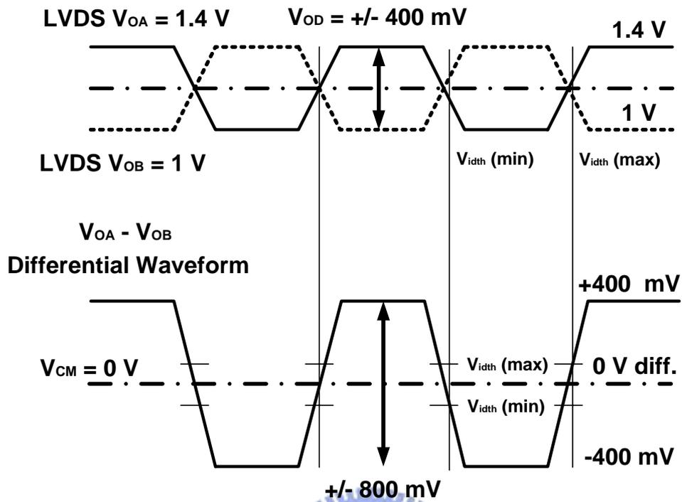
Fig. 2.2 The driver signal level of LVDS for 1.2V  $V_{OS}$
