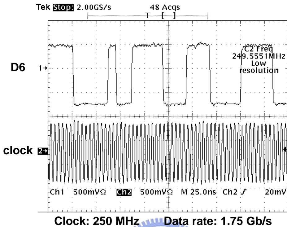
Fig. 5.28 LVDS Link measurement result at data rate up to 1.75 Gb/s
