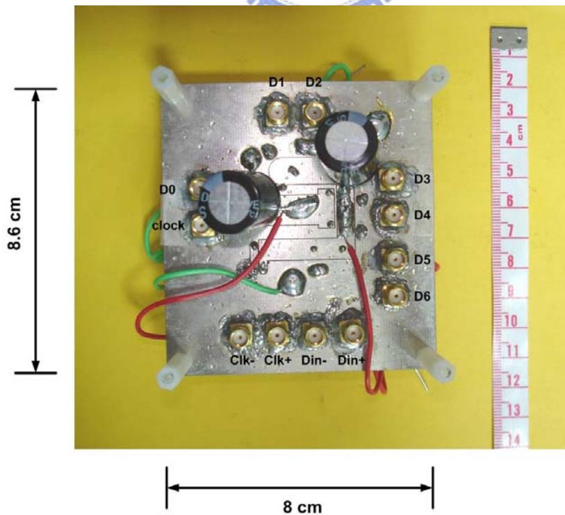
Fig. 5.17 Bottom view of the parallel output testing PCB photo
