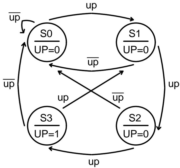
Fig. 4.15 State diagram of DLPF
