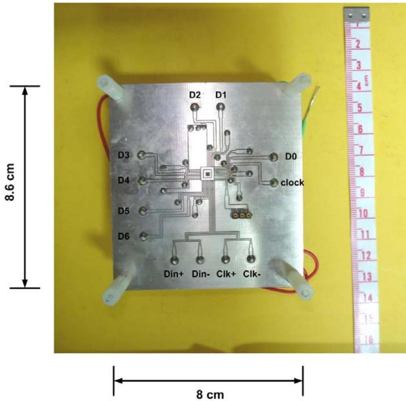
Fig. 5.16 Top view of the parallel output testing PCB photo
