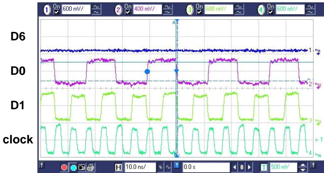
Fig. 5.22 Parallel output testing result when set a 150ps skew in pattern generator
