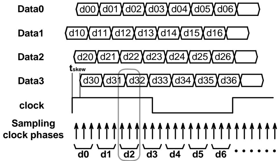
Fig. 3.7 Operation timing of three times oversampling when skews happen
