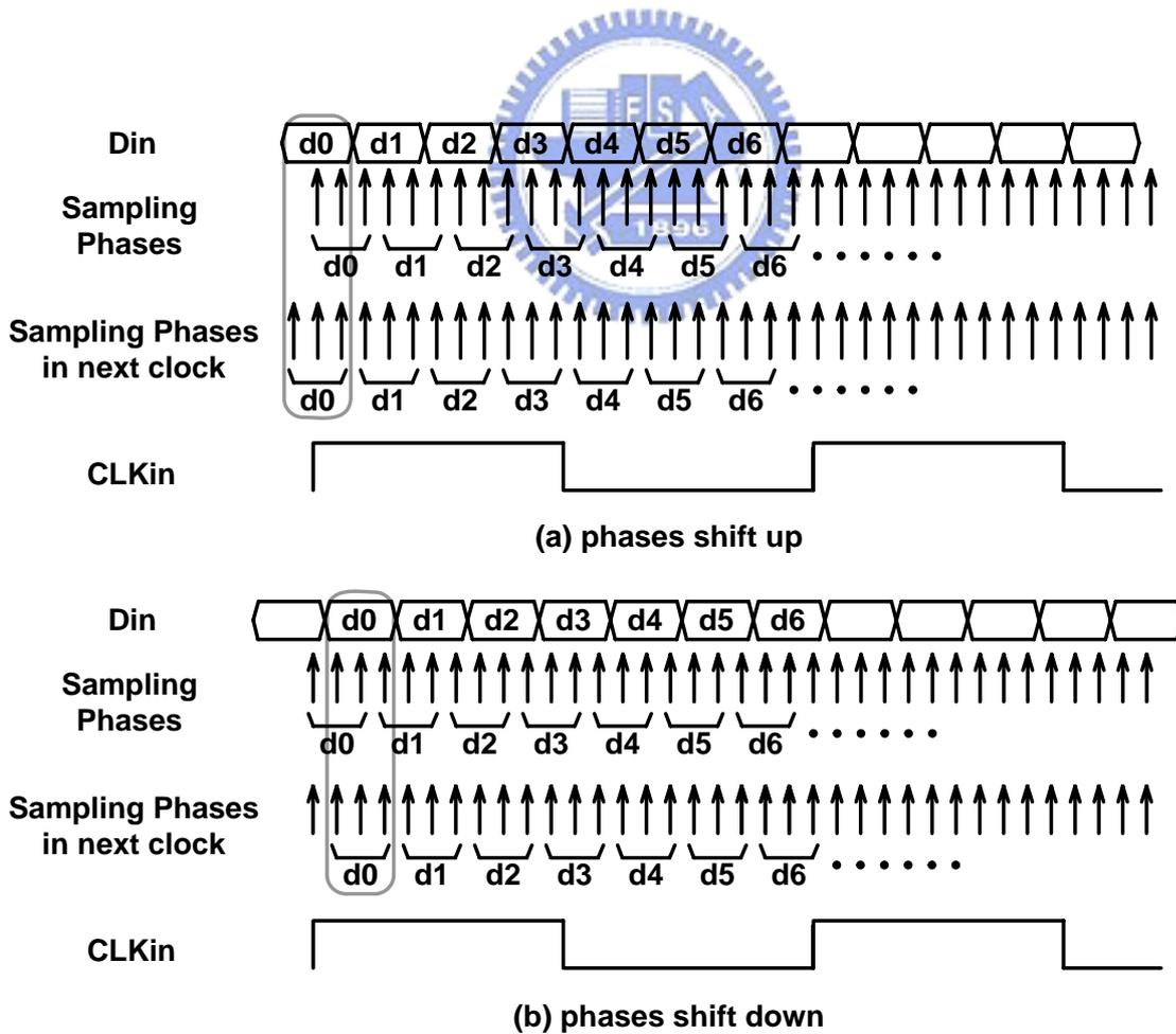
Fig. 3.12 Operation of phase selector
