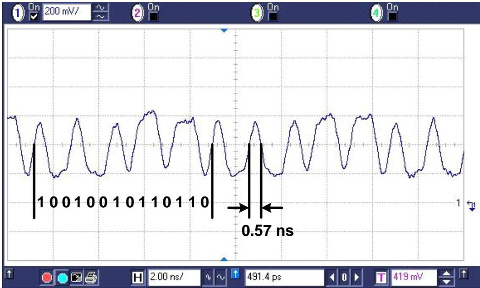
Fig. 5.12 Cyclic “1001001 0110110” pattern test result at data rate up to 1.8 Gb/s
