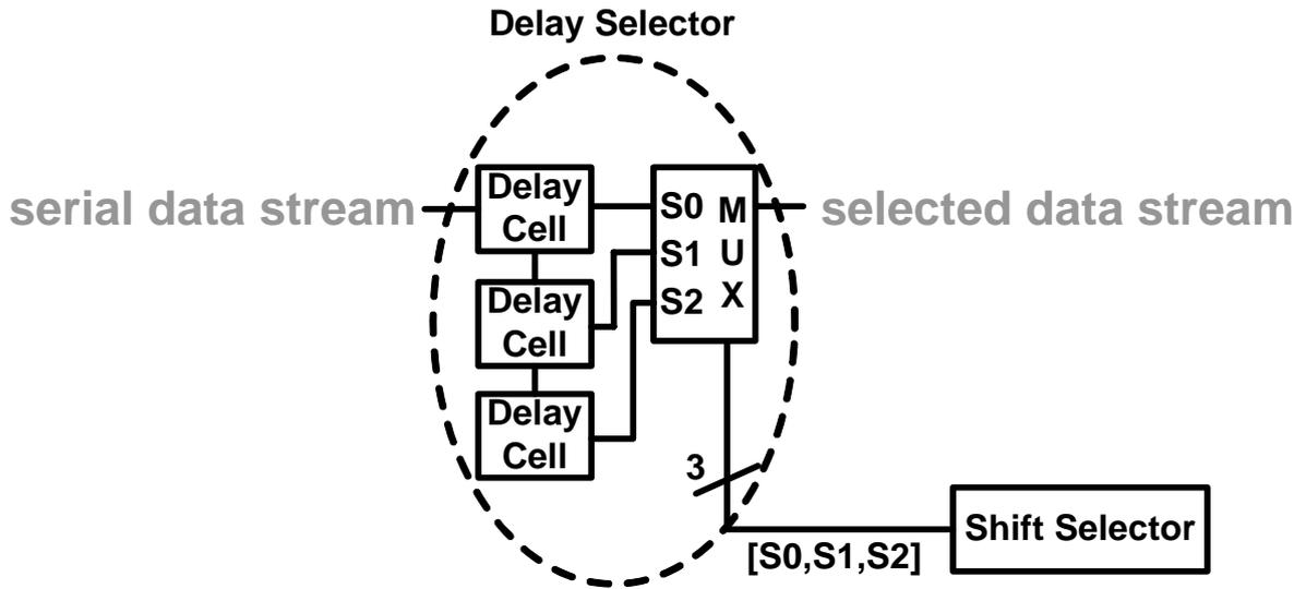
Fig. 4.17 Sifter selector and delay selector
