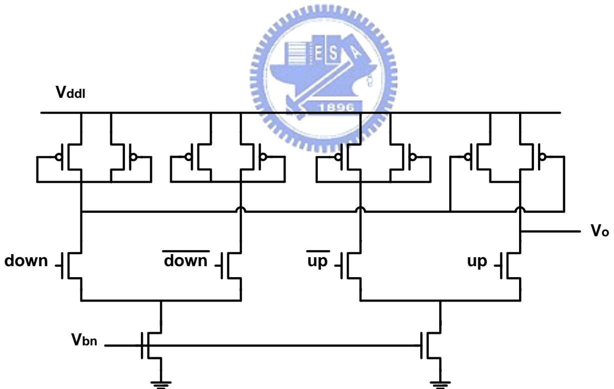
Fig. 4.20 Schematic diagram of the charge pump
