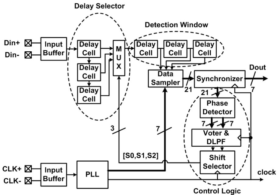
Fig. 3.20 Architecture of a "delay selecting" CDR
