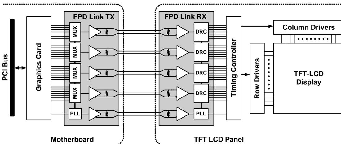
Fig. 1.2 A typical FPD Link application
