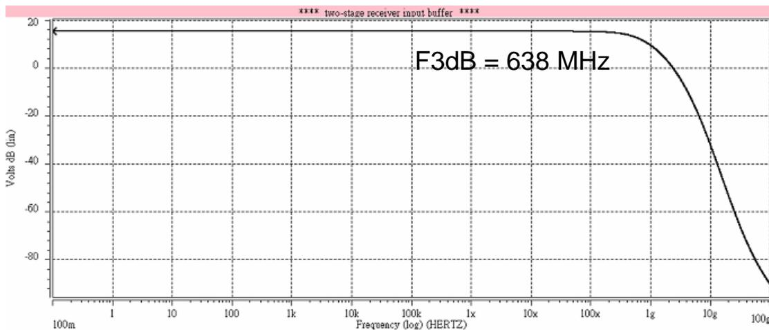
Fig. 4.4 Simulated frequency response of the LVDS receiver input buffer (Fig. 4.3)
