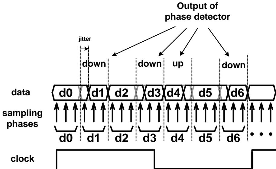
Fig. 3.11 Operation of phase detector when jitters happen
