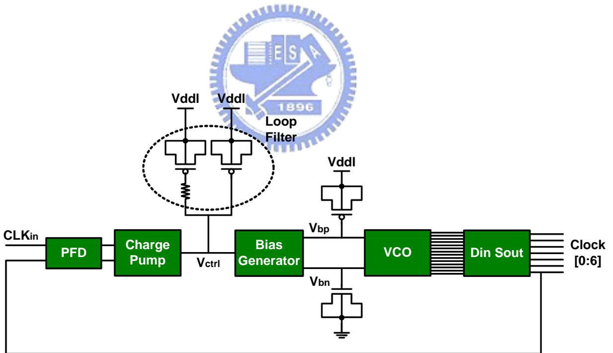
Fig. 4.18 Architecture of the designed PLL
