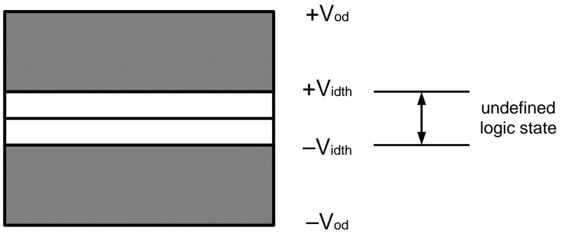
Fig. 2.4 Receiver input signal levels
