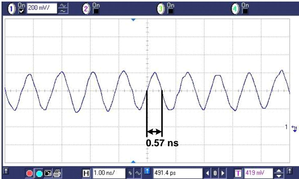
Fig. 5.8 Cyclic “010101” pattern test result at data rate up to 1.8 Gb/s
