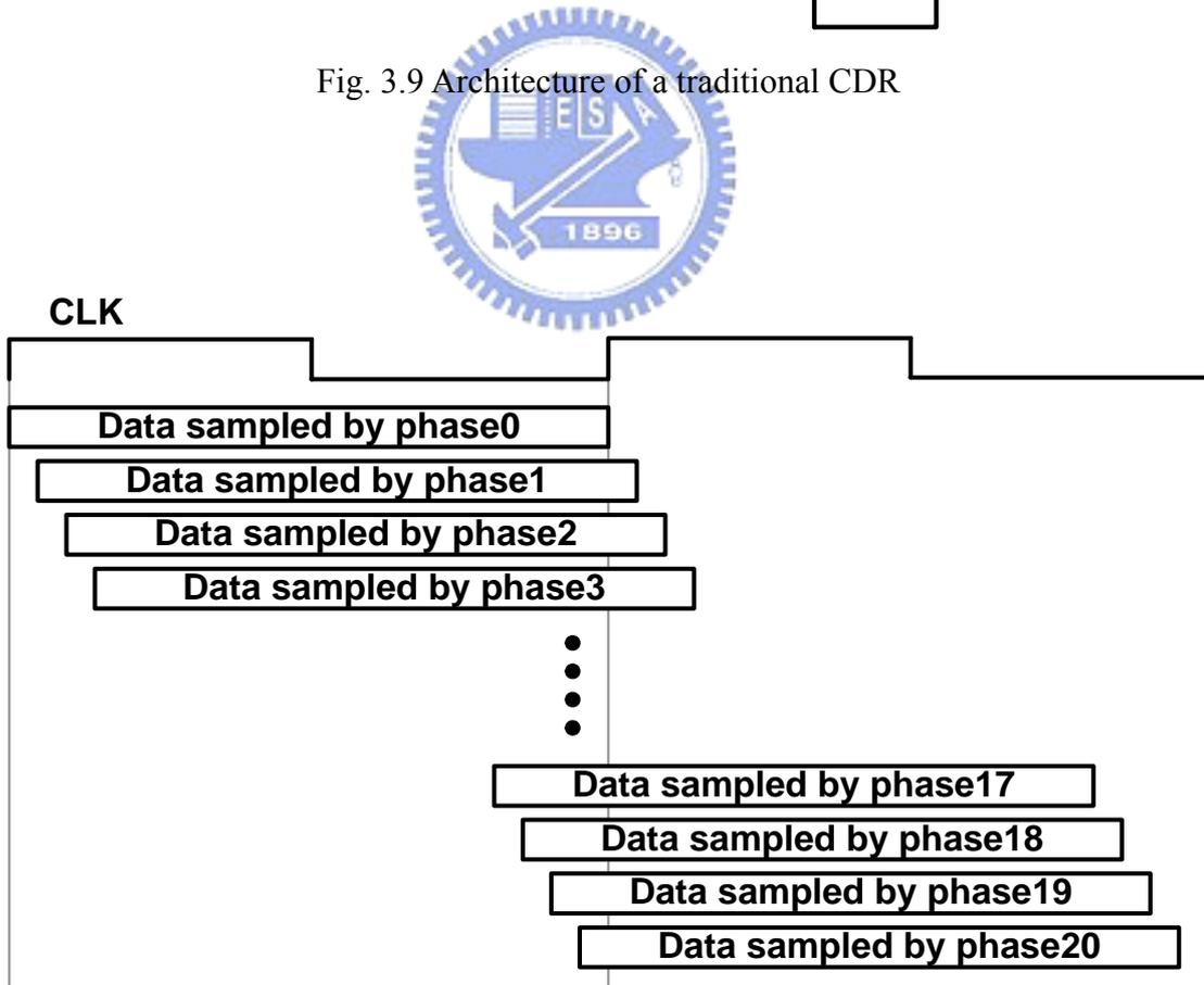
Fig. 3.10 Timing relation between sampled data
