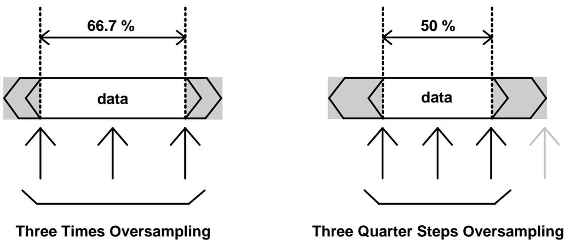
Fig. 3.18 Comparison of eye diagram tolerance in lock state
