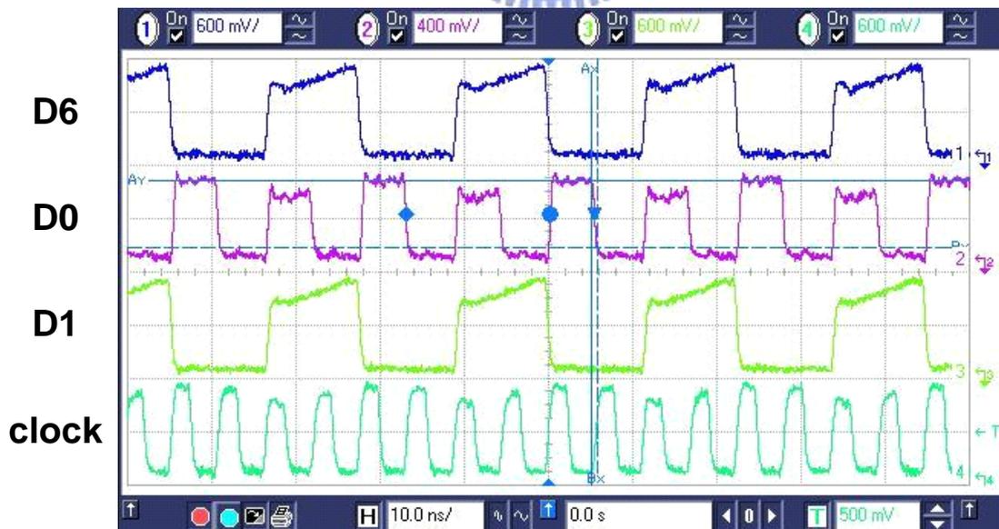
Fig. 5.21 Parallel output testing result when set a 100ps skew in pattern generator
