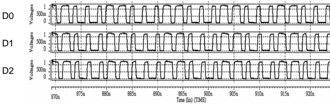
Fig. 4.8 Simulation result of the delay cells and differential to the single ended converters
