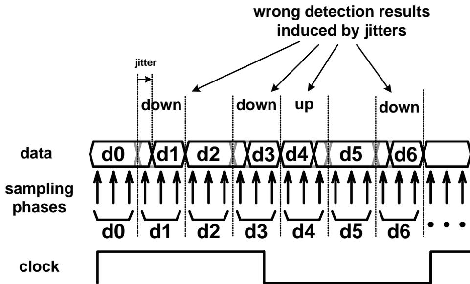
Fig. 4.13 Wrong detection results induced by jitters
