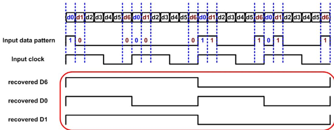
Fig. 5.18 Test pattern for skew tolerance test
