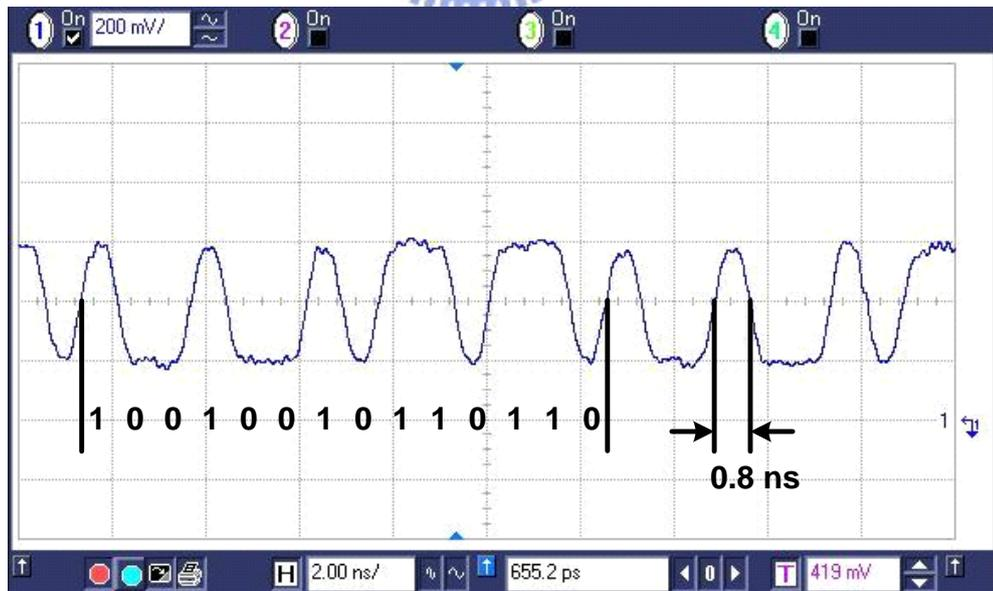
Fig. 5.11 Cyclic “1001001 0110110” pattern test result at data rate up to 1.25 Gb/s
