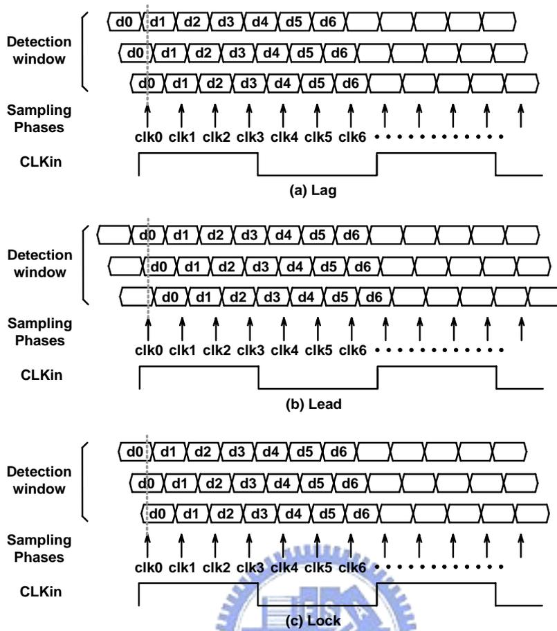
Fig. 3.19 Operation of the detection window
