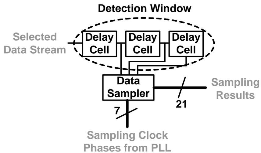
Fig. 4.10 Detection window and data sampler
