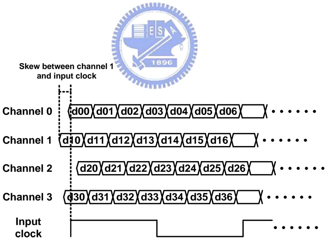
Fig. 1.4 The timing relation between data and clock when skews happen
