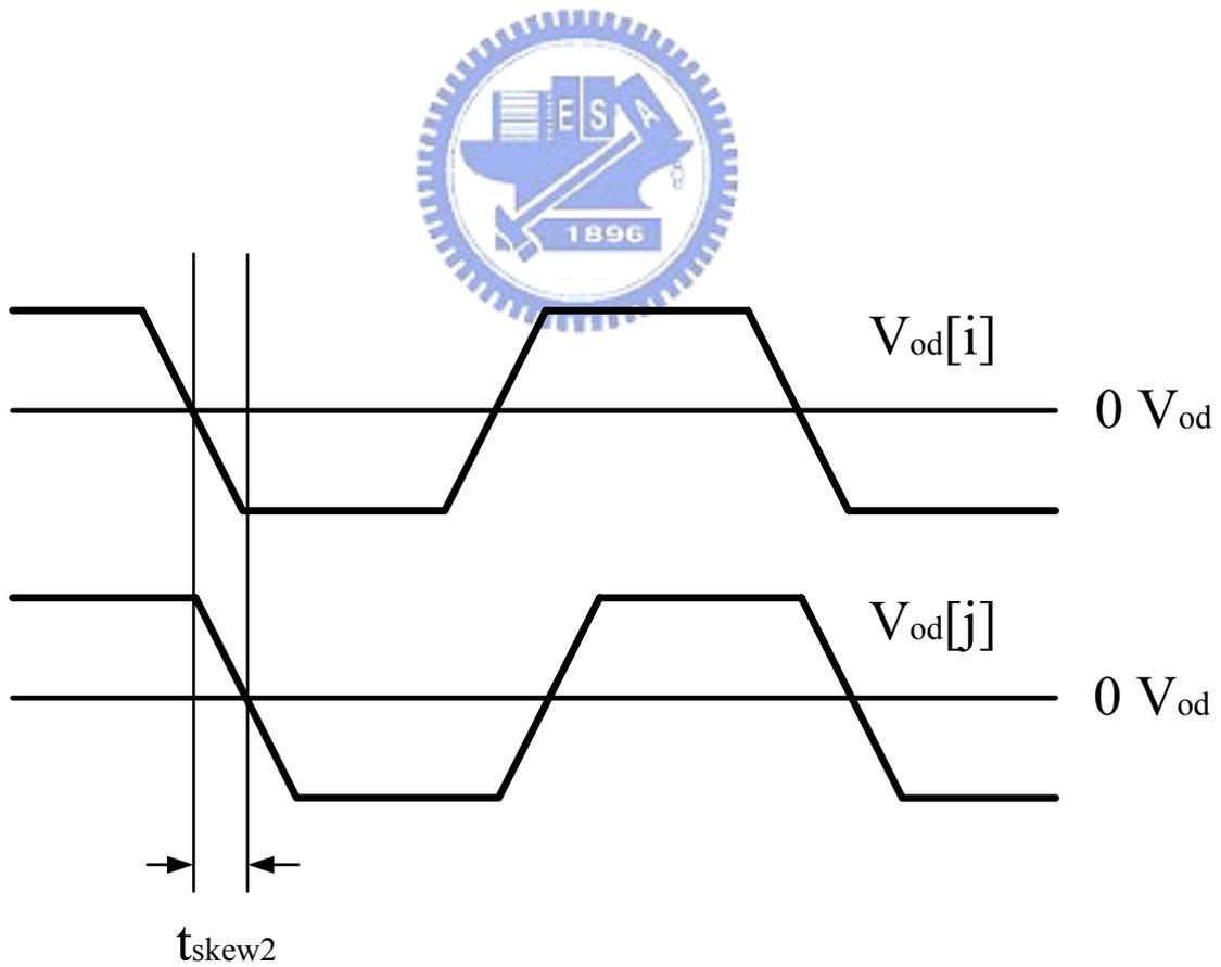
Fig. 2.9  $t_{skew2}$  between any parallel signals
