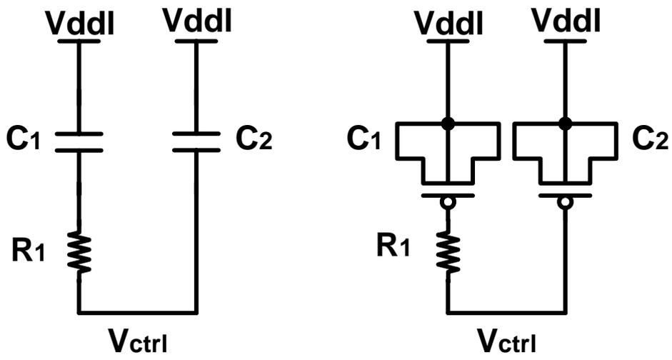
Fig. 4.21 Schematic diagram of the loop filter
