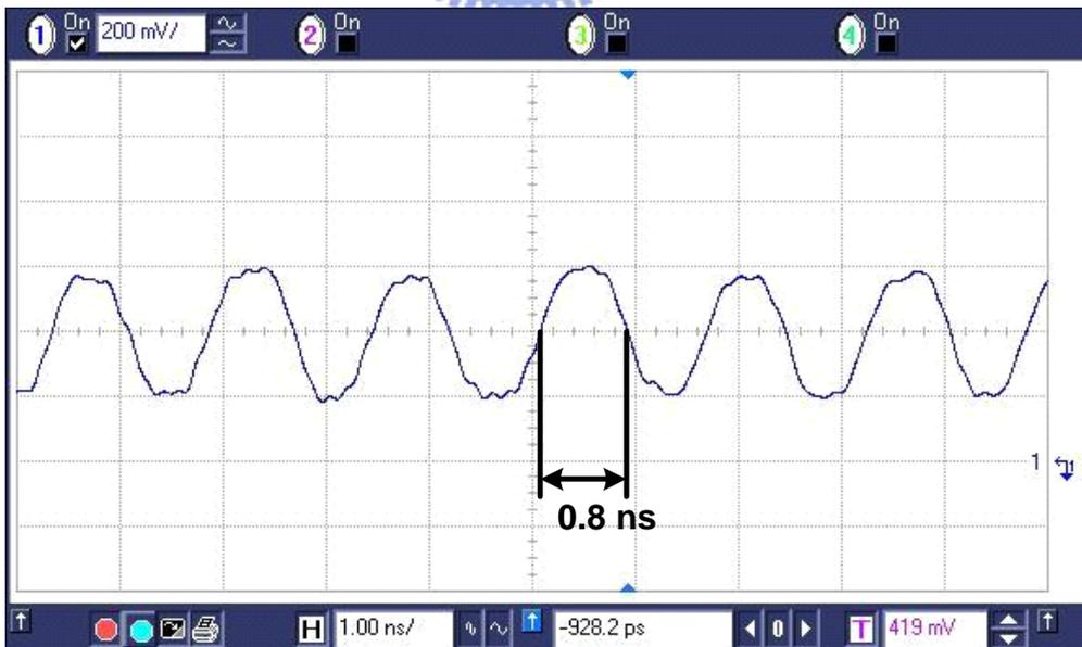
Fig. 5.7 Cyclic “010101” pattern test result at data rate up to 1.25 Gb/s
