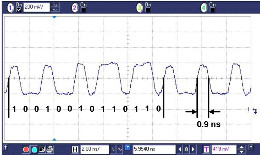
Fig. 5.10 Cyclic “1001001 0110110” pattern test result at data rate up to 1.1 Gb/s
