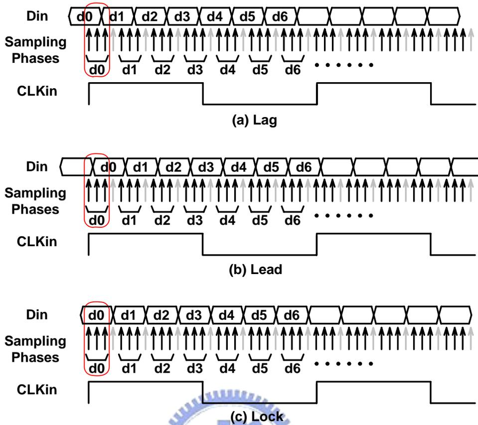
Fig. 3.17 Operation of “three quarter steps oversampling”
