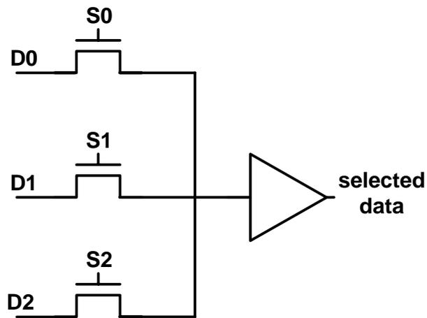
Fig. 4.9 Schematic diagram of the three to one MUX
