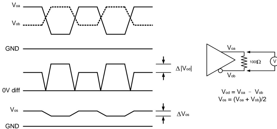
Fig. 2.3 The definition of  $\Delta V_{od}$  and  $\Delta V_{os}$
