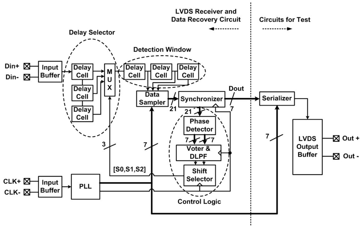
Fig. 5.2 Block diagrams of the serial output test circuit in the tap out test chip
