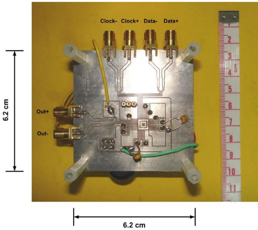
Fig. 5.4 Top view of the serial output testing PCB photo
