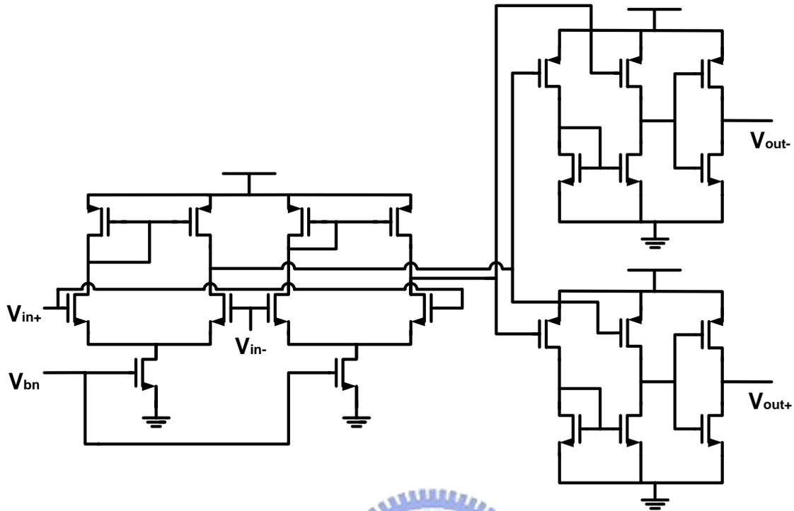
Fig. 4.7 Schematic diagram of the differential to single ended converter
