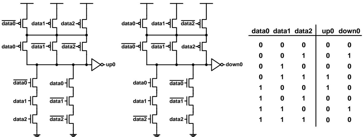
Fig. 4.12 Schematic diagram and truth table of the phase detector
