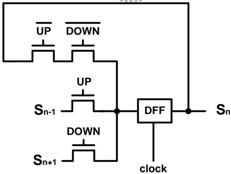
Fig. 4.16 Schematic diagram of the shift selector
