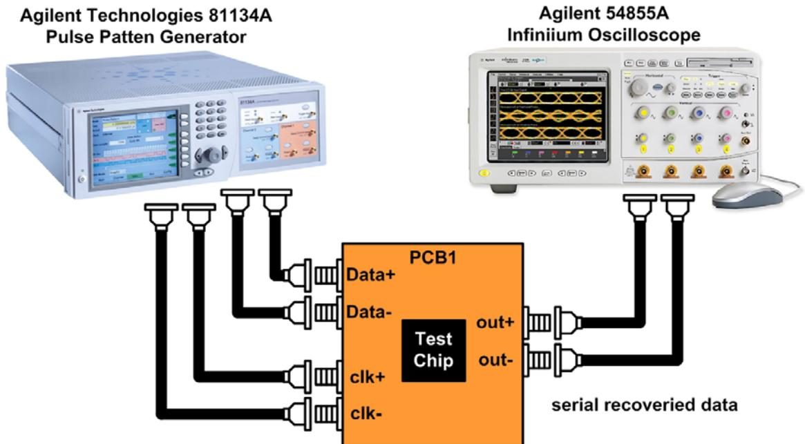
Fig. 5.3 Measurement environment setting of the serial output test
