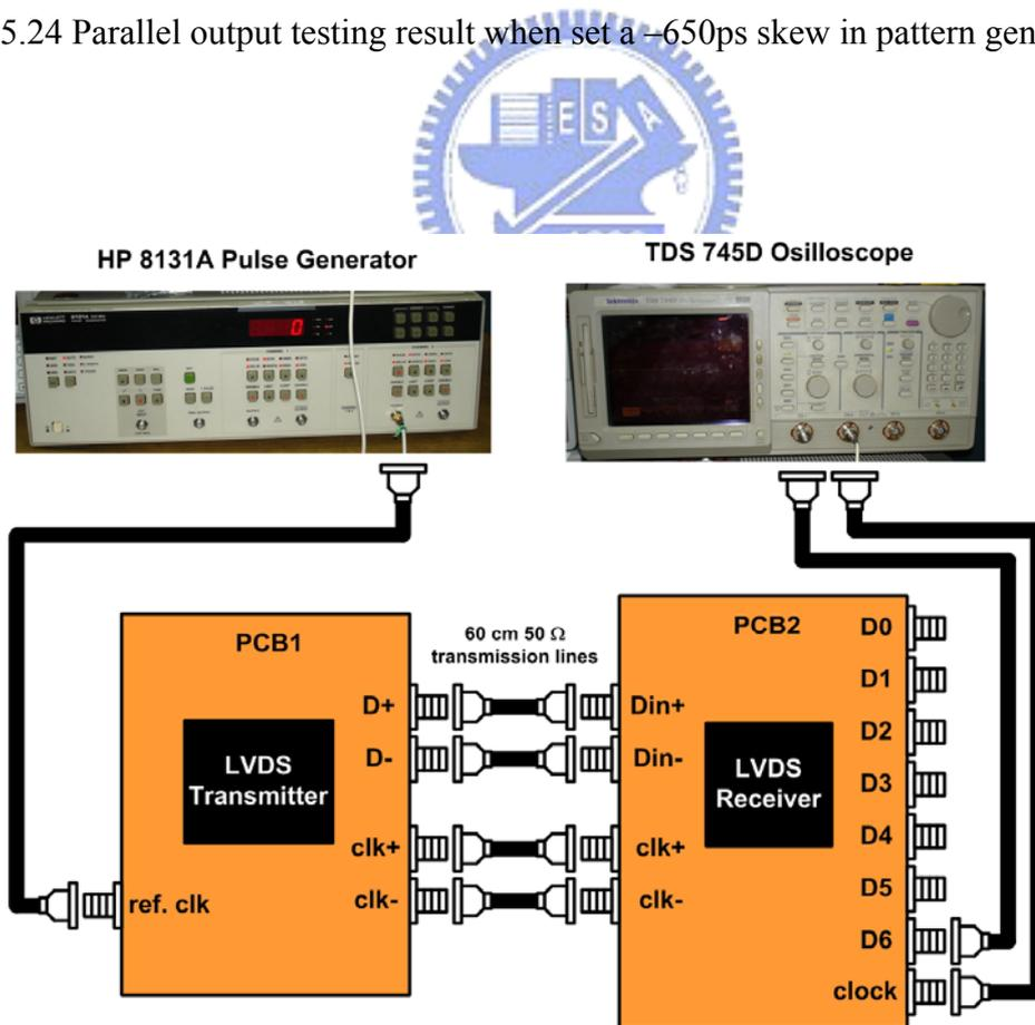
Fig. 5.25 Measurement environment setup of the LVDS Link test
