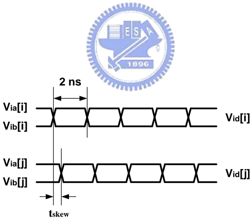
Fig. 2.7  $t_{skew}$  between two receiver inputs
