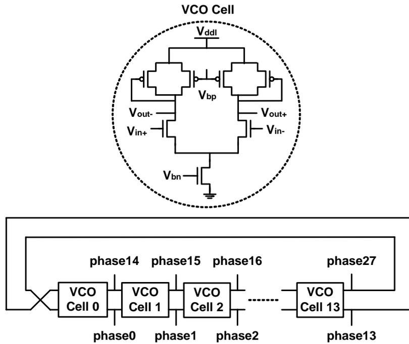
Fig. 4.23 Schematic diagram of the VCO
