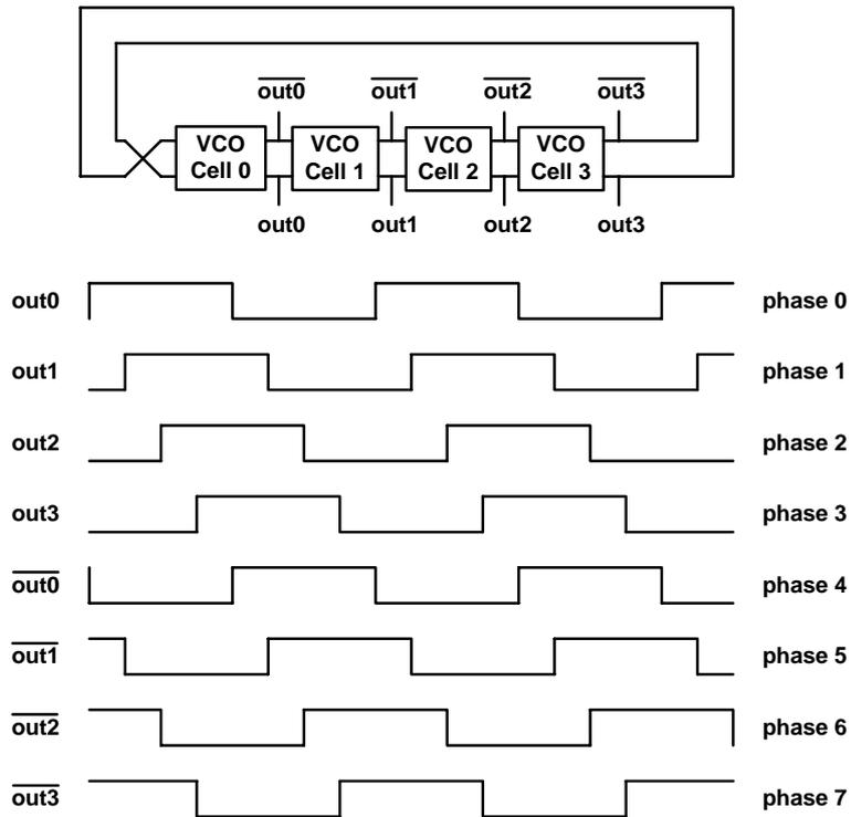
Fig. 3.15 Timing relation between VCO cells outputs
