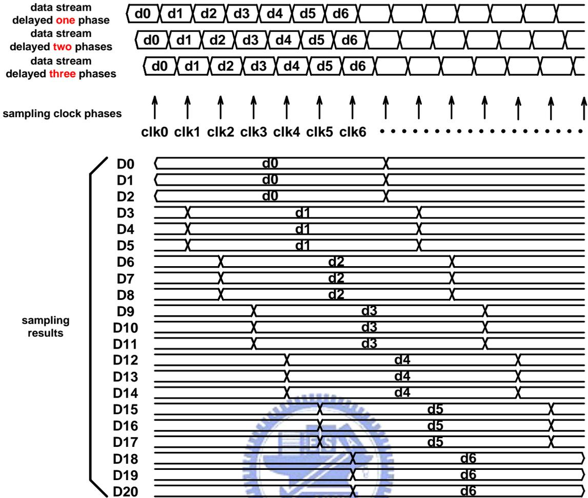
Fig. 4.11 Operation timing of the data sampler
