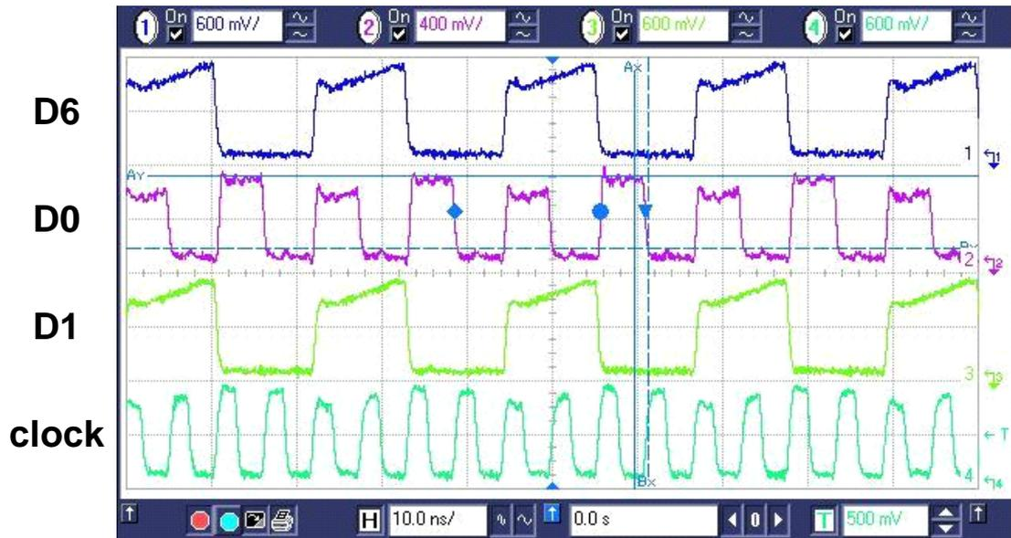
Fig. 5.20 Parallel output testing result when no skew is set in pattern generator
