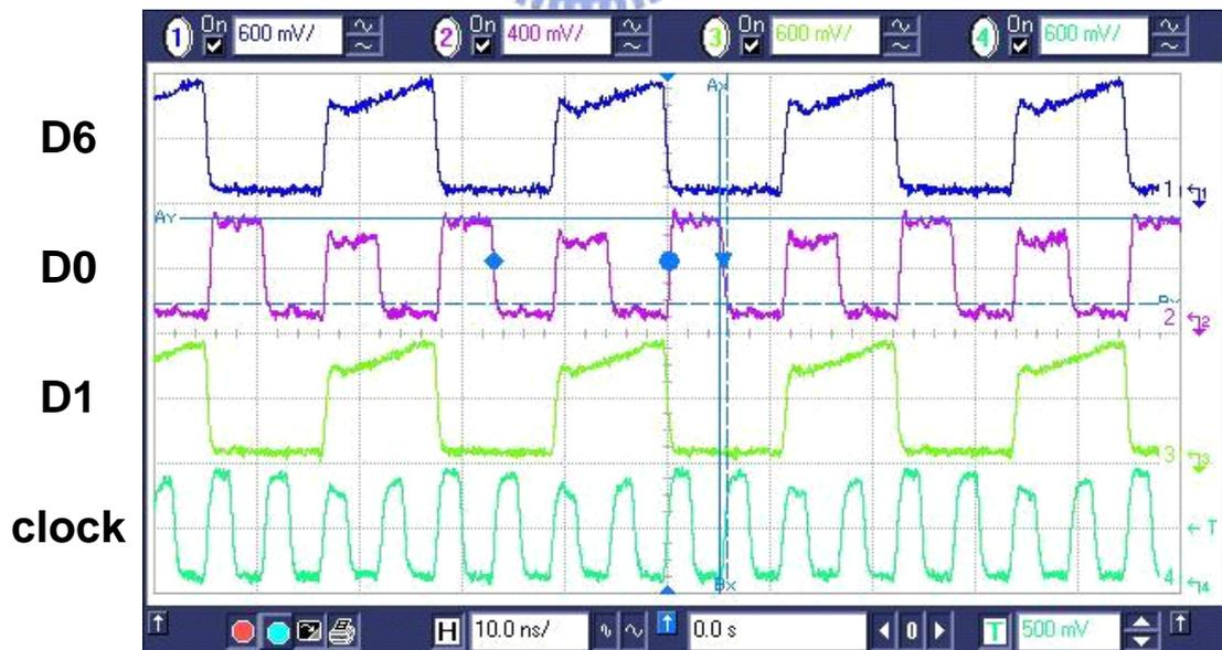
Fig. 5.23 Parallel output testing result when set a -600ps skew in pattern generator
