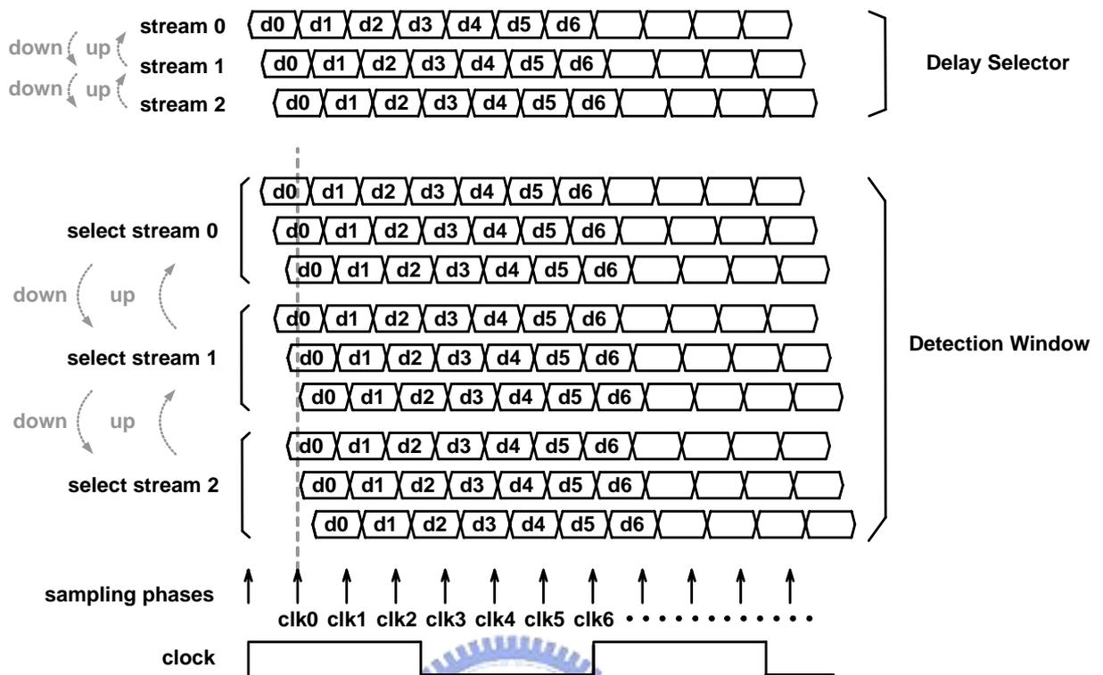
Fig. 3.21 Operation of the "delay selecting" CDR
