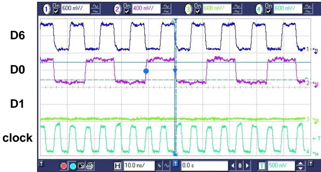
Fig. 5.24 Parallel output testing result when set a -650ps skew in pattern generator
