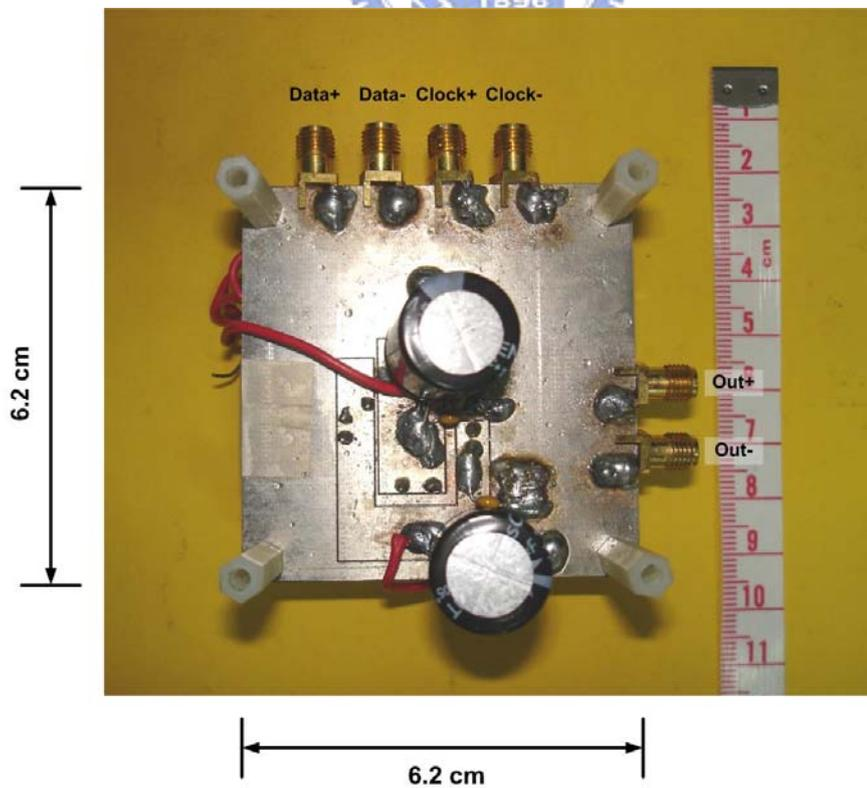
Fig. 5.5 Bottom view of the serial output testing PCB photo
