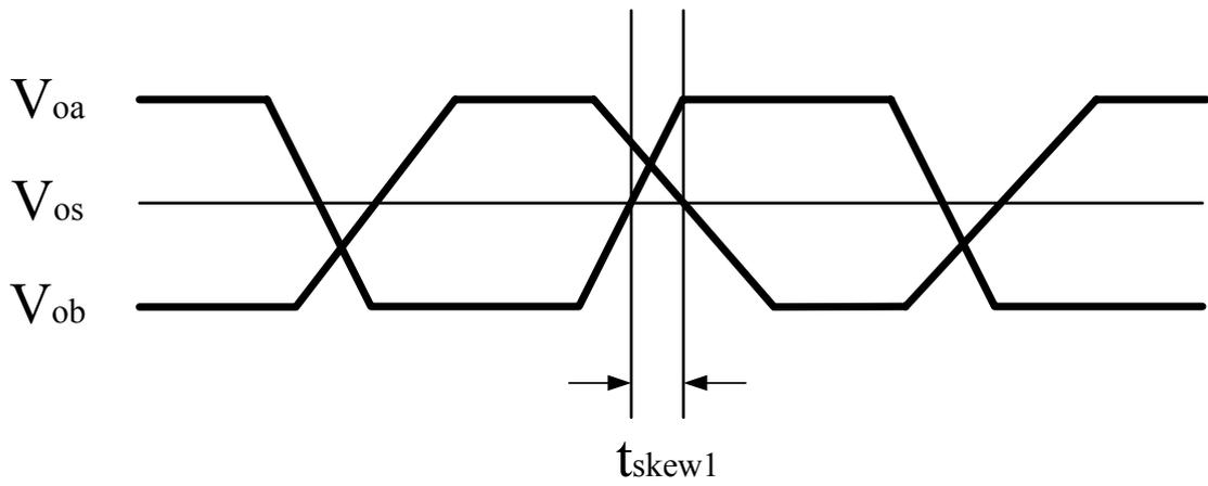
Fig. 2.8  $t_{skew1}$  between complementary single-ended signals
