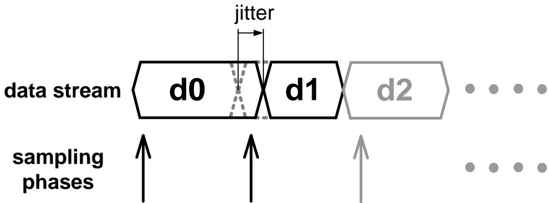
Fig. 3.5 Operation timing when jitters happen, d0 is double sampled and d1 is missed
