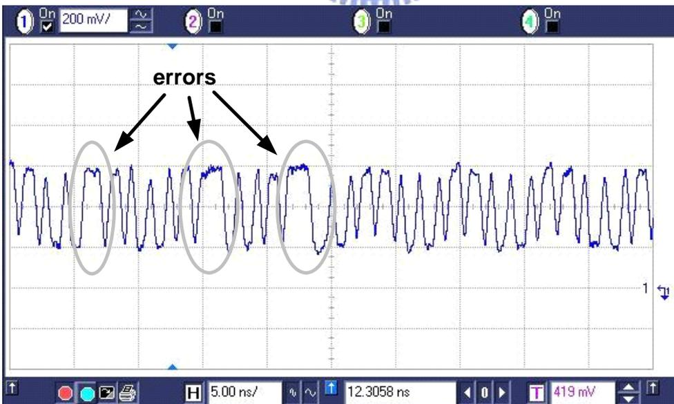
Fig. 5.13 Cyclic “1001001 0110110” pattern test result at data rate up to 2 Gb/s
