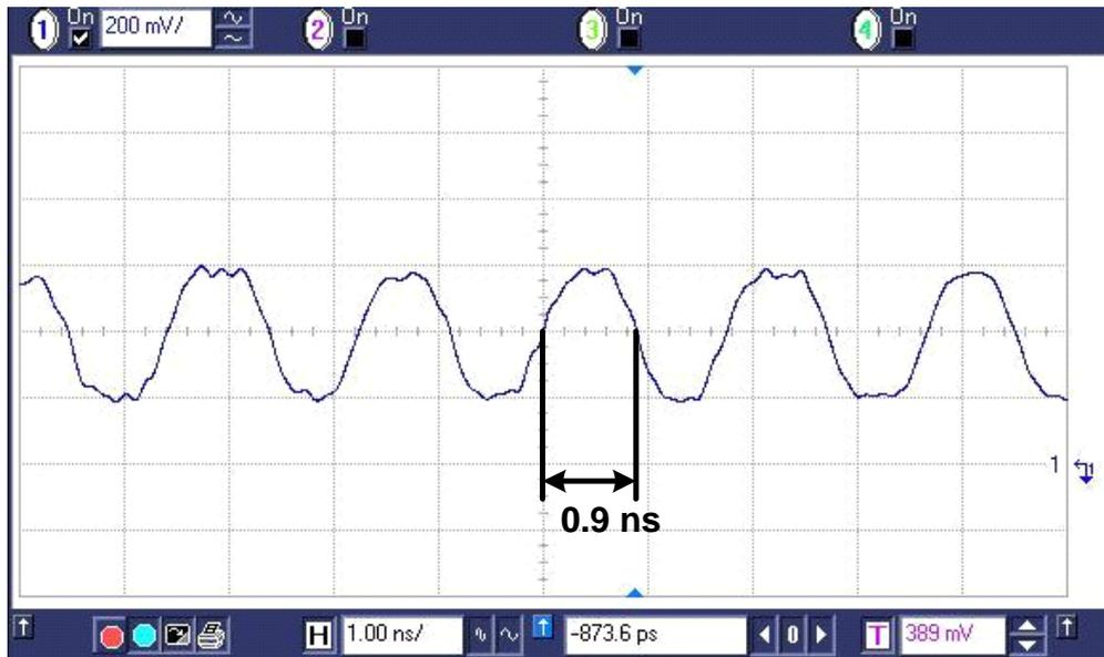
Fig. 5.6 Cyclic “010101” pattern test result at data rate up to 1.1 Gb/s
