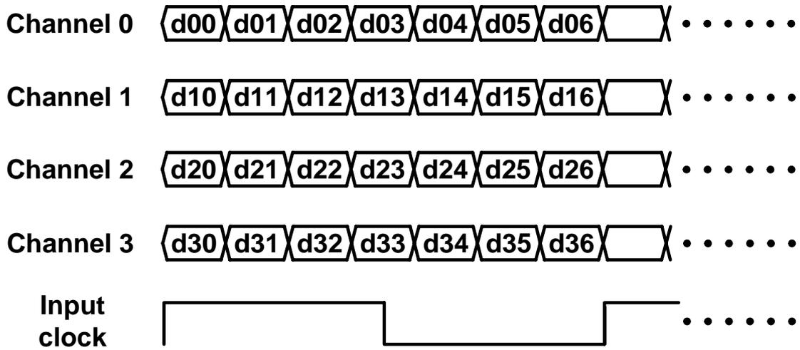
Fig. 1.3 The timing relation between input data and input clock in channels
