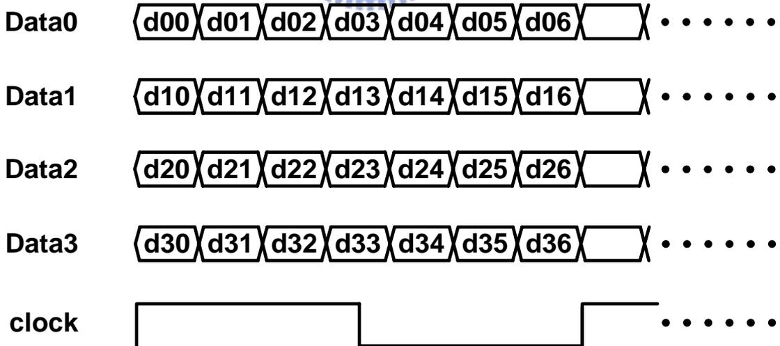
Fig. 3.2 Timing relation between clock and serial data streams
