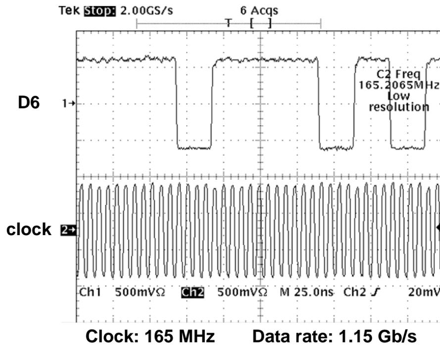
Fig. 5.26 LVDS Link measurement result at data rate up to 1.15 Gb/s
