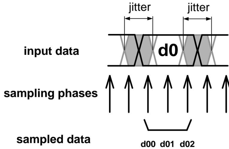
Fig. 3.13 Data sampling timing when jitters happen
