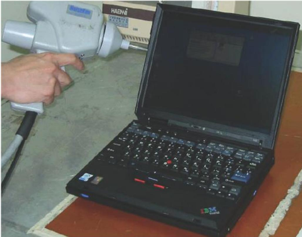
Fig. 1.4 System-level EMC/ESD test on LCD panel of notebook by an ESD gun.
