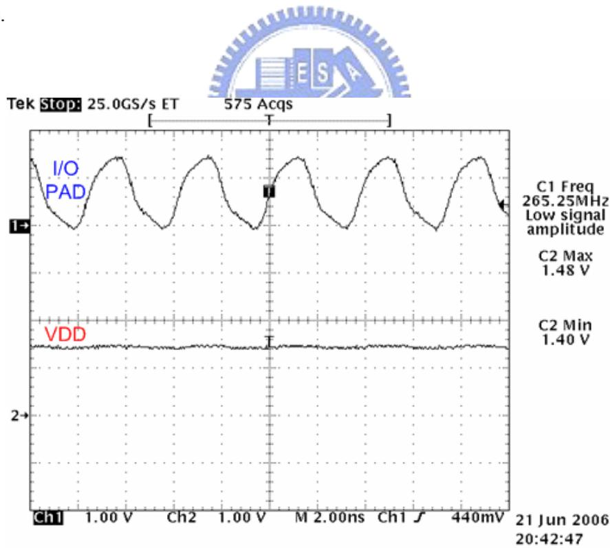
Fig. 4.31 Measured ground bounce on VDD pad of TBNMXIO-SR (with slew-rate control).
