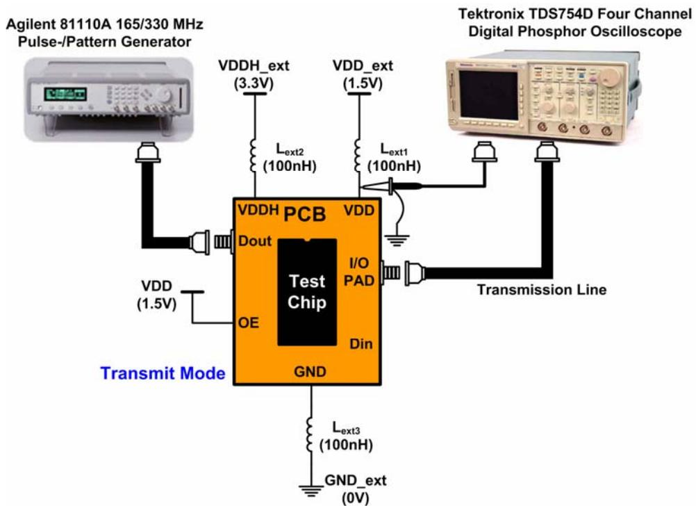
Fig. 4.29 The setup for ground bounce measurement.
