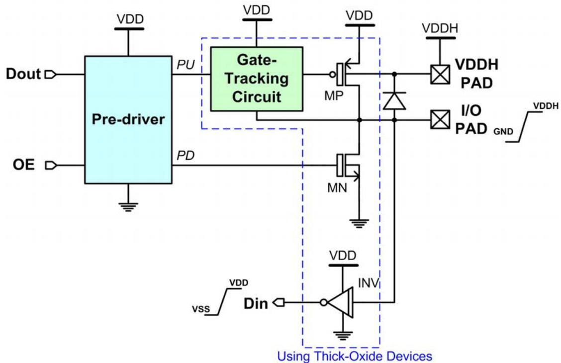
Fig. 1.2 Block diagram of a mixed-voltage I/O buffer with dual-oxide devices and an external n-well bias voltage.
