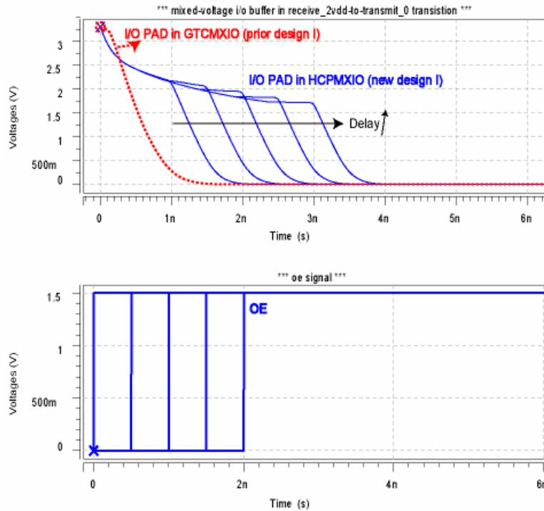
Fig. 3.12 Simulation waveforms of the HCPMXIO in transition with increasing the delay of high level at OE signal.
