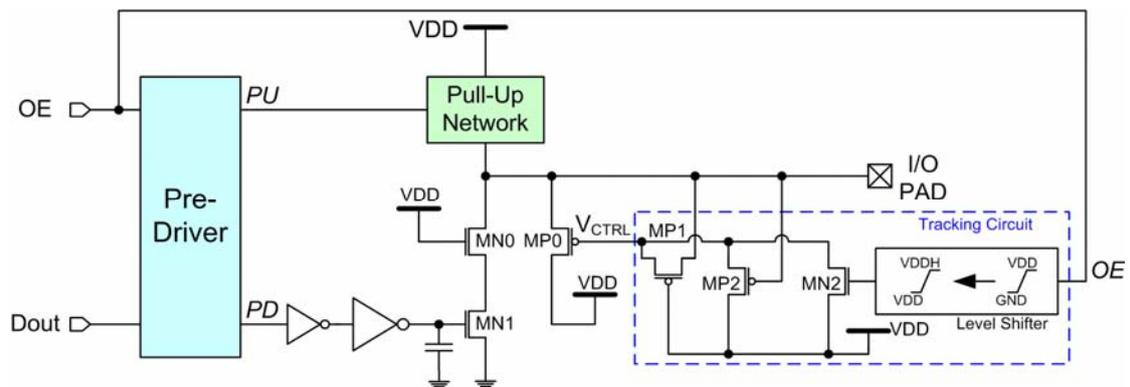
Fig. 3.4 The implementation of the new proposed hot-carrier-prevented circuit for  $2xVDD$ -tolerant I/O buffer with two-stacked transistors.
