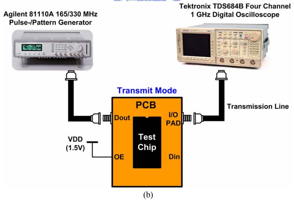
Fig. 3.20 The measurement setup of mixed-voltage I/O buffer (a) in receive mode and (b) in transmit mode.
