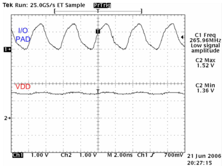
Fig. 4.30 Measured ground bounce on VDD pad of TBNMXIO (without slew-rate control).
