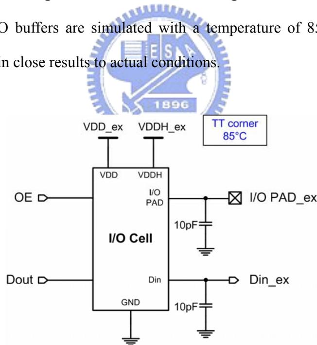
Fig. 3.7 The simulation environment.
