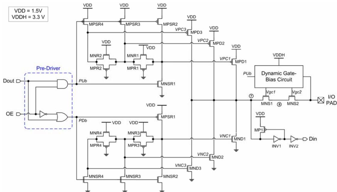
Fig. 4.4 The TBNMXIO with slew-rate control.
