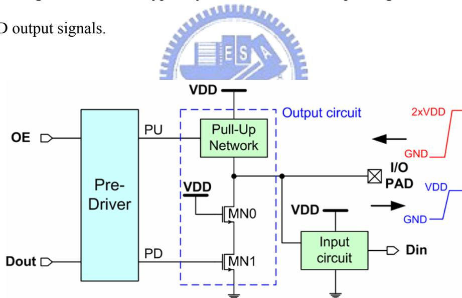
Fig. 1.3 Simplified mixed-voltage I/O buffer with two-stacked transistors.
