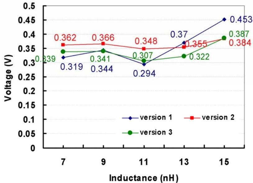
Fig. 4.19 The undershoot on VDD power line with different transistor sizes of output driver.
