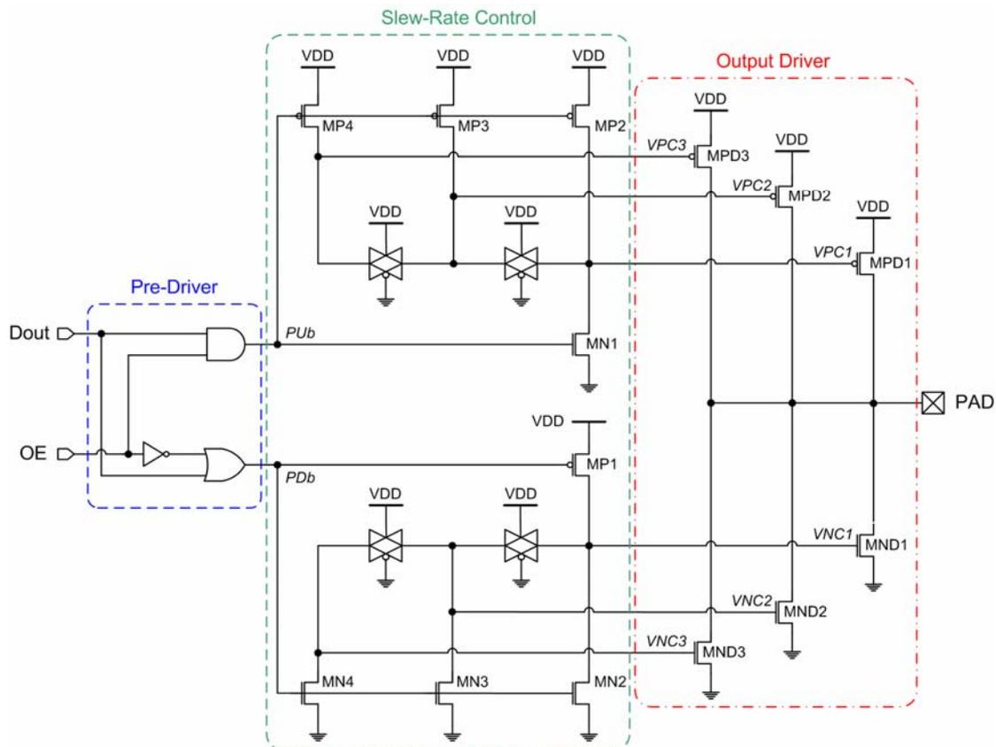
Fig. 4.3 Output buffer with an improved slew-rate control to reduce short-circuit current.
