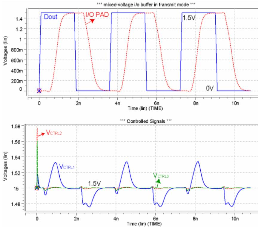
Fig. 3.9 Simulation waveforms of the HCPMXIO in transmitting mode with 266-MHz output signals.
