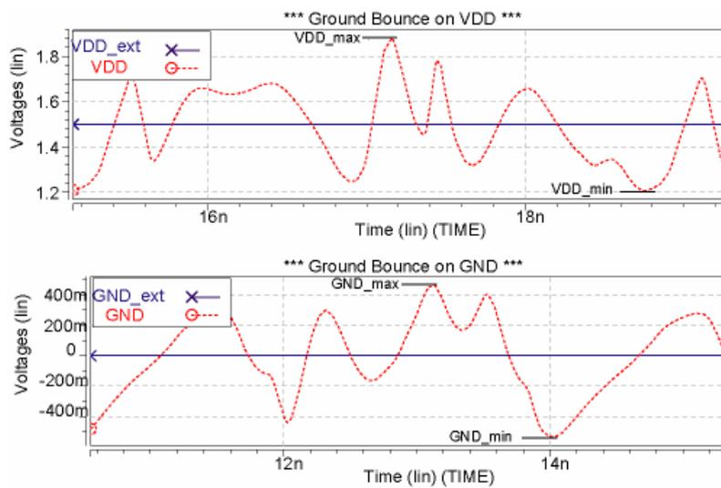
Fig. 4.7 Simulation waveforms of ground bounce effects on power lines.
