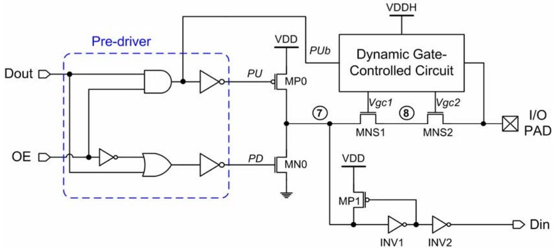
Fig. 3.13 The new proposed 2xVDD-tolerant I/O buffer with two blocking NMOS devices and dynamic gate-controlled circuit to solve the hot-carrier reliability issue (TBNMXIO).
