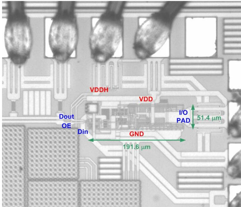
Fig. 3.18 The photograph of the new proposed 2xVDD-tolerant I/O buffer with hot-carrier-prevented circuits (HCPMXIO) in a 0.18- $\mu\text{m}$  1.8-V CMOS process.
