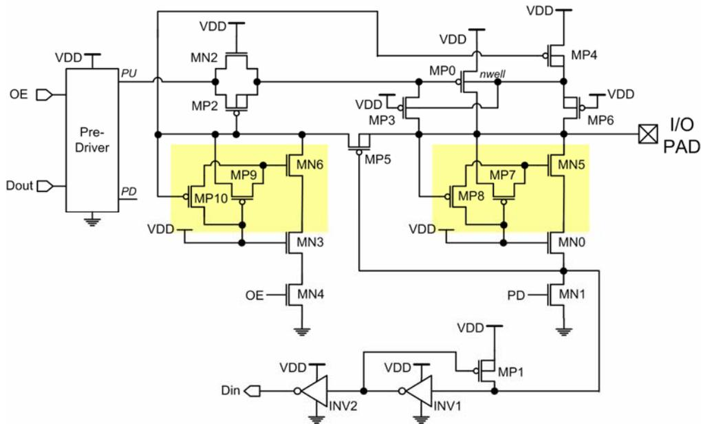
Fig. 3.2 The mixed-voltage I/O buffer using three-stacked NMOS transistors (TSTMXIO).
