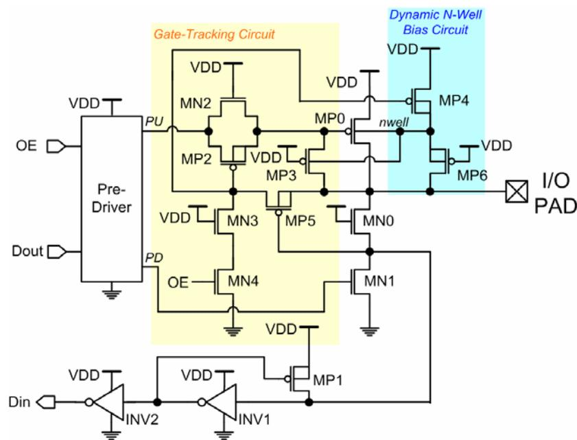
Fig. 2.3 The mixed-voltage I/O buffer with gate-tracking circuit and dynamic n-well bias circuit proposed in [9].
