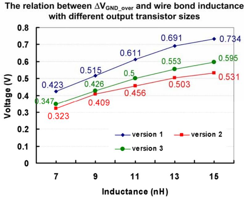
Fig. 4.20 The overshoot on GND power line with different transistor sizes of output driver.
