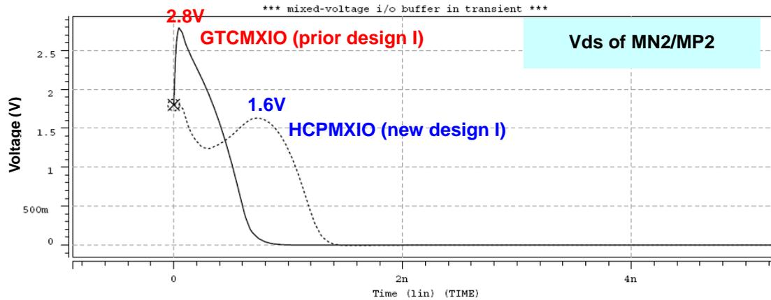
Fig. 3.11 The drain-source voltages of MN2 during the transition from receiving 3.3-V input signal to transmitting 1.5-V output signal.
