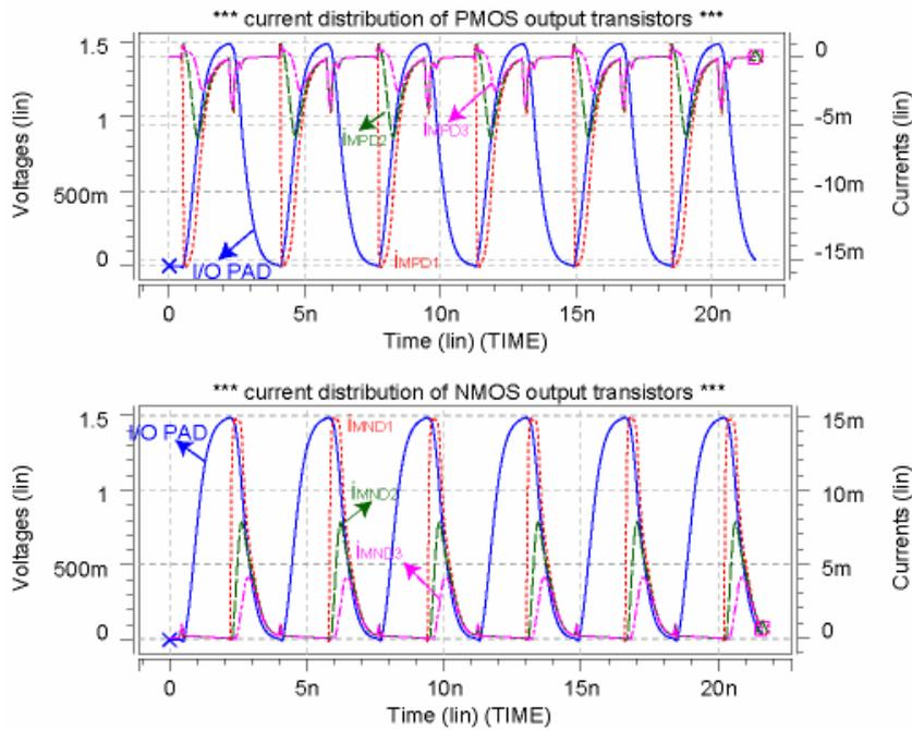
Fig. 4.18 Current distributions of output transistors in the TBNMXIO-SR operated in receive mode.
