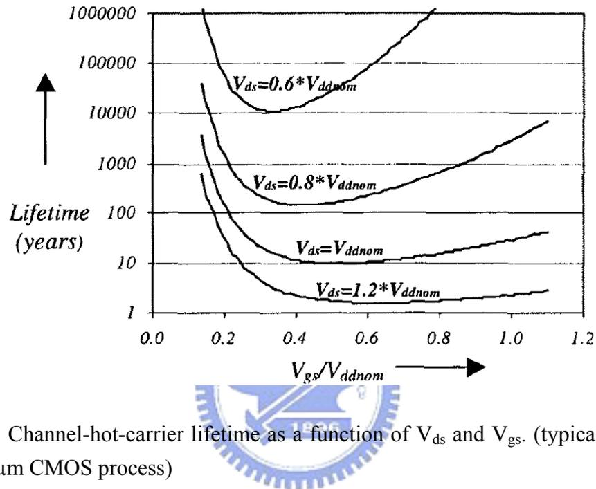
Fig. 1.5 Channel-hot-carrier lifetime as a function of  $V_{ds}$  and  $V_{gs}$ . (typical behavior for 0.25- $\mu\text{m}$  CMOS process)
