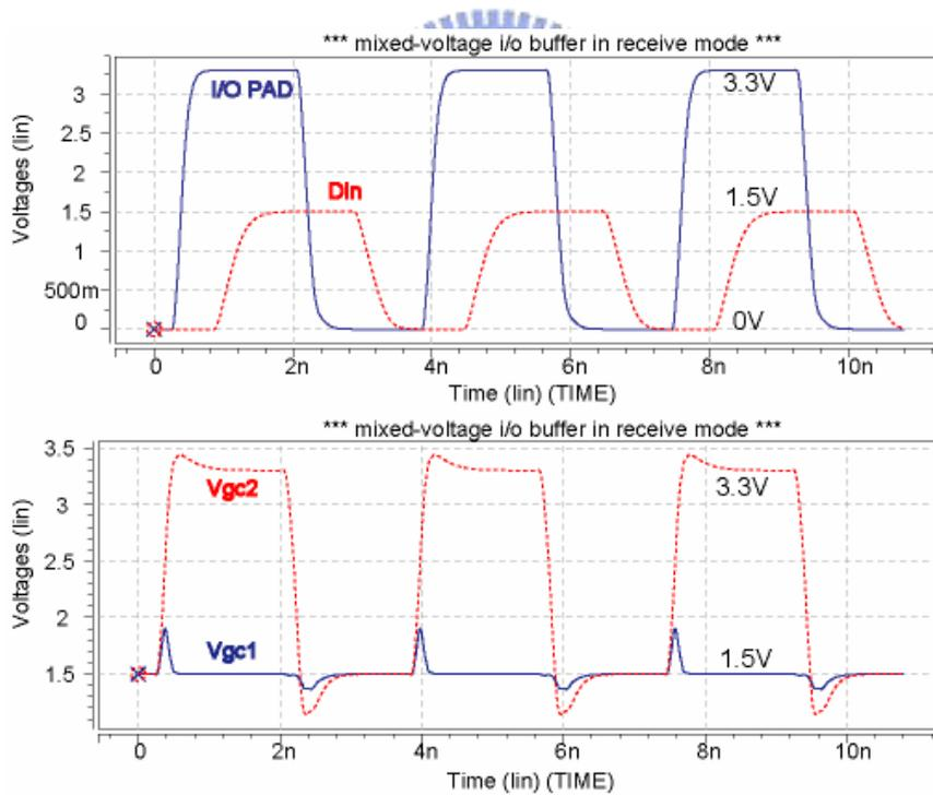
Fig. 3.15 Simulation waveforms of the TBNMXIO operating at 266 MHz when receiving 0V-to-3.3V input signals at I/O PAD.
