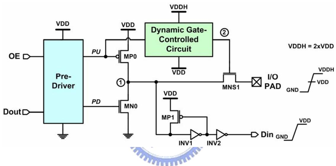
Fig. 2.4 The mixed-voltage I/O buffer with a blocking NMOS and a dynamic gate-controlled circuit.
