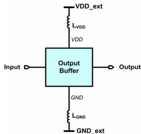
Fig. 4.1 The model for ground bounce effect.
