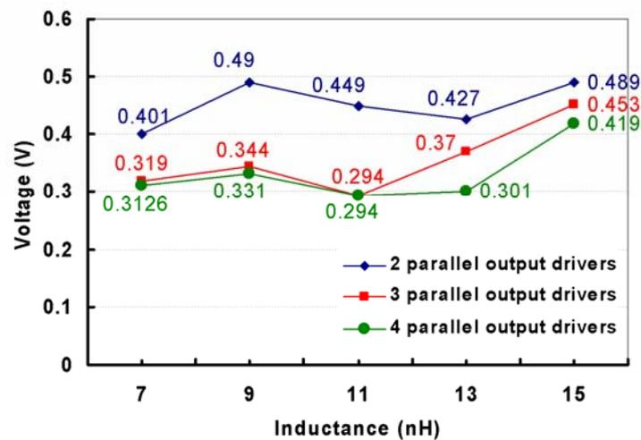
Fig. 4.16 The undershoot on VDD power line with different number of parallel output drivers.
