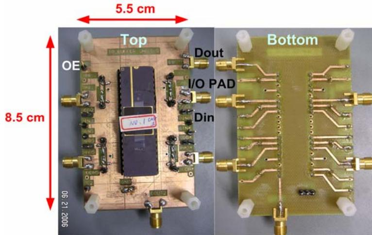
Fig. 3.21 The PCB view of tested mixed-voltage I/O buffers.
