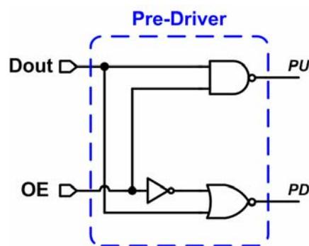
Fig. 2.2 The circuit implementation of pre-driver.
