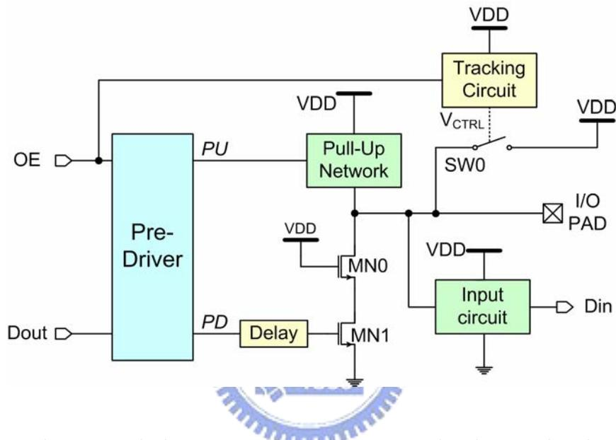
Fig. 3.3 The new design concept to overcome the hot-carrier issue in the  $2xVDD$ -tolerant I/O buffer with only two-stacked transistors.
