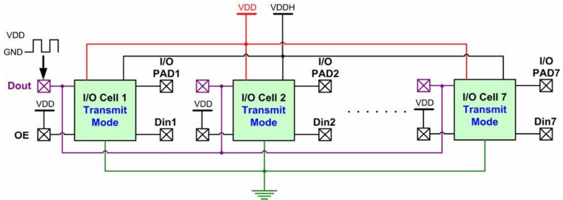
Fig. 4.32 The measurement method of ground bounce effect where seven I/O cells switch simultaneously.
