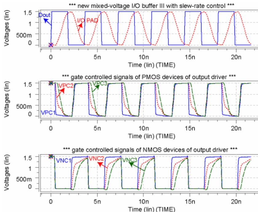
Fig. 4.13 Simulation waveforms of the HCPMXIO-SR operating at 266 MHz when transmitting 0V-to-1.5V output signals to I/O PAD.
