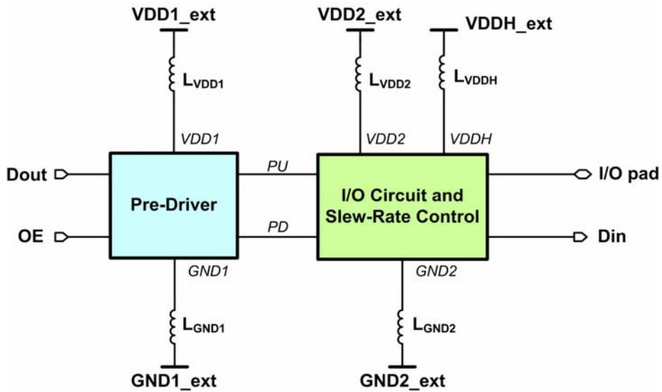
Fig. 4.21 The second simulation model of ground bounce using two separate VDD pads.
