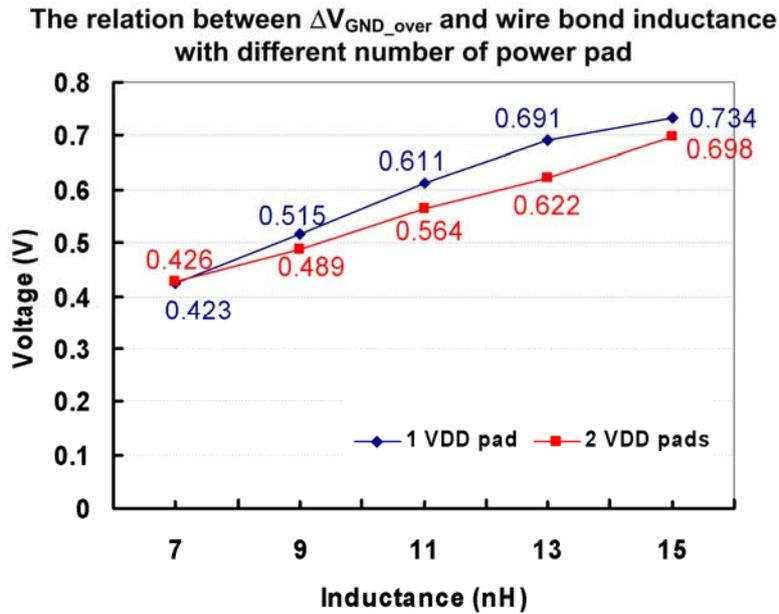
Fig. 4.23 The overshoot on GND power line with different number of power pad.
