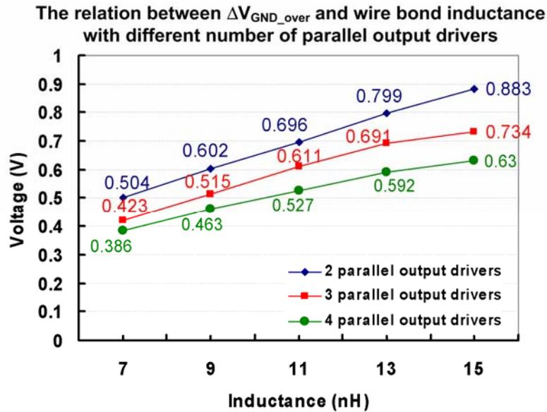
Fig. 4.17 The overshoot on GND power line with different number of parallel output drivers.
