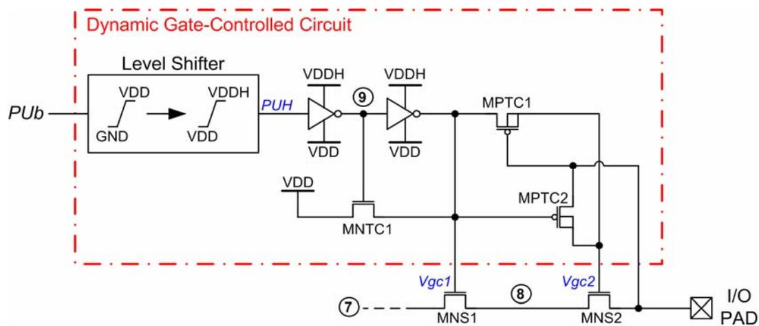
Fig. 3.14 Circuit implementation of the dynamic gate-controlled circuit in the TBNMXIO.
