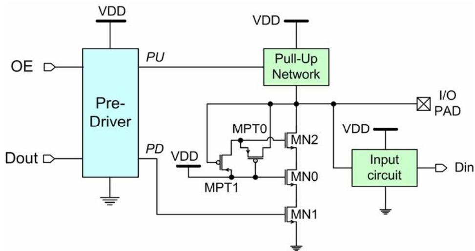
Fig. 3.1 The brief schematic of 2xVDD-tolerant I/O buffer with three-stacked transistors to overcome hot-carrier issue.
