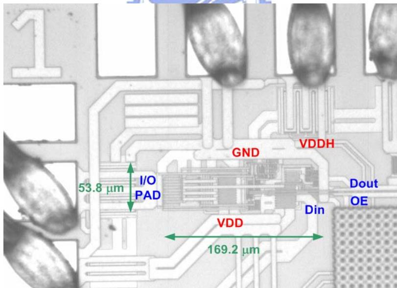
Fig. 3.19 The photograph of the new proposed 2xVDD-tolerant I/O buffer with blocking NMOS devices (TBNMXIO) in a 0.18- $\mu\text{m}$  1.8-V CMOS process.
