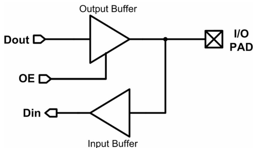
Fig. 1.1 Block diagram of bidirectional I/O buffer.
