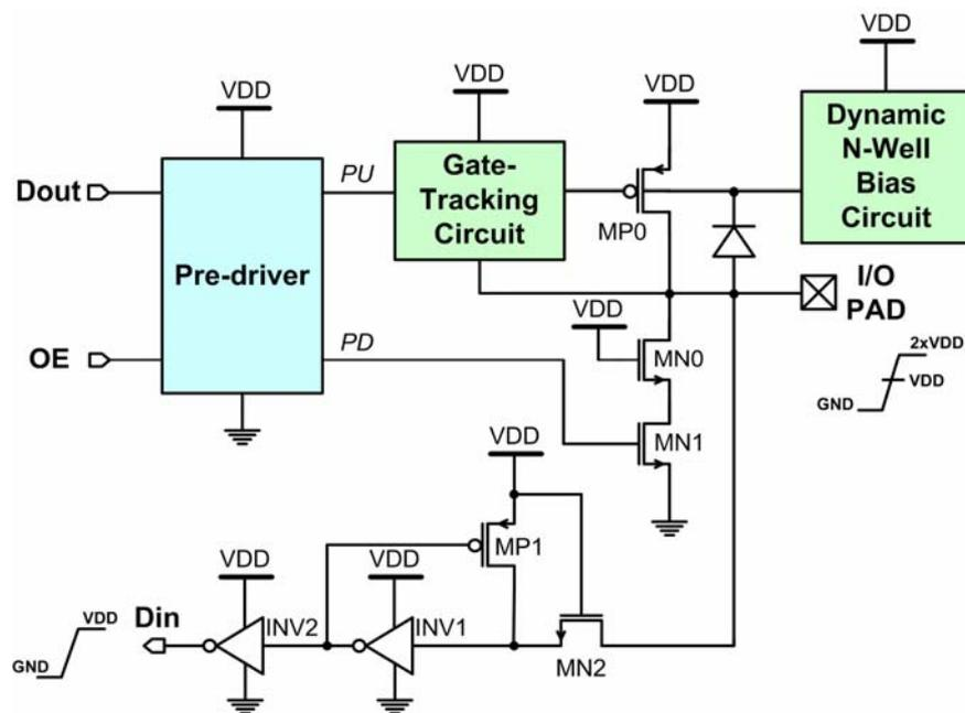
Fig. 2.1 Basic design concept for mixed-voltage I/O buffer realized with only thin-oxide devices.
