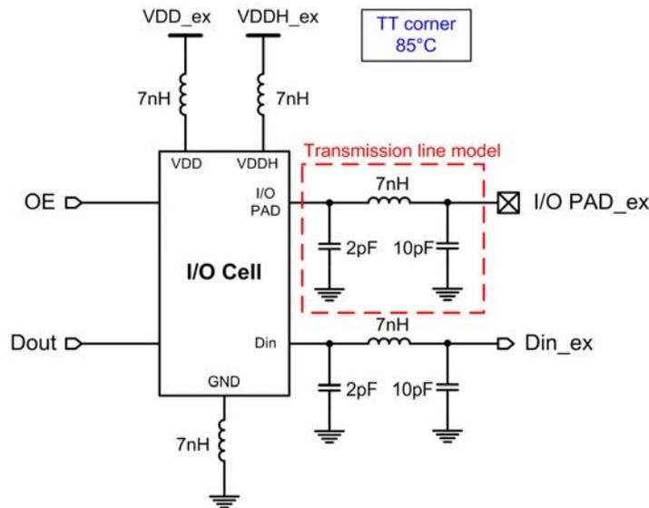
Fig. 3.28 Modified simulation model with bonding wire and transmission line effects.
