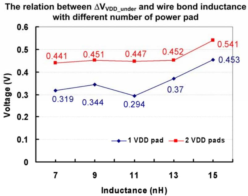
Fig. 4.22 The undershoot on VDD power line with different number of power pad.
