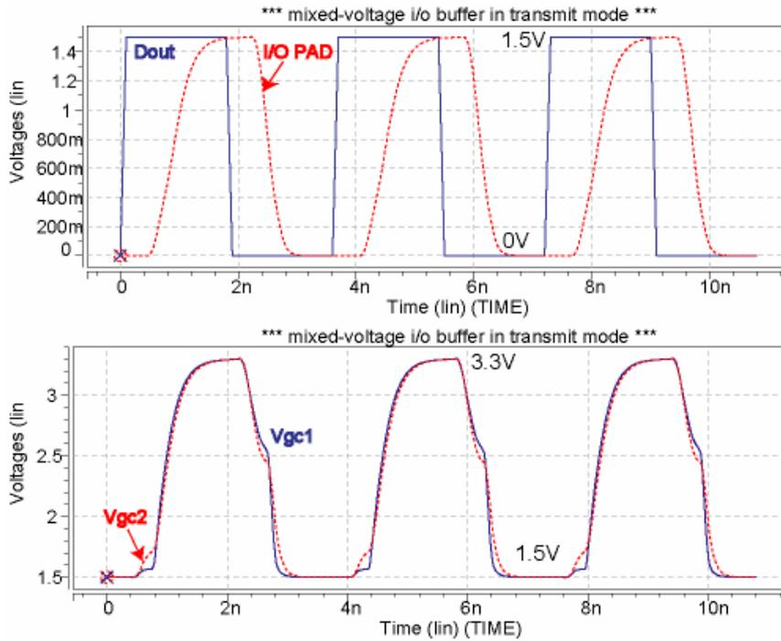
Fig. 3.16 Simulation waveforms of the TBNMXIO operating at 266 MHz when transmitting 0V-to-1.5V output signals to I/O PAD.
