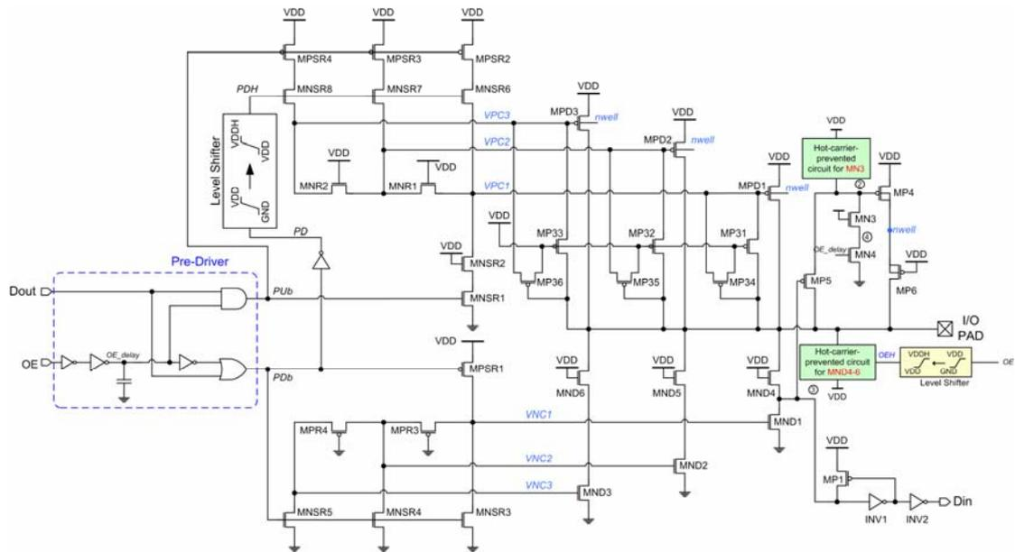
Fig. 4.12 The HCPMXIO with modified slew-rate control.
