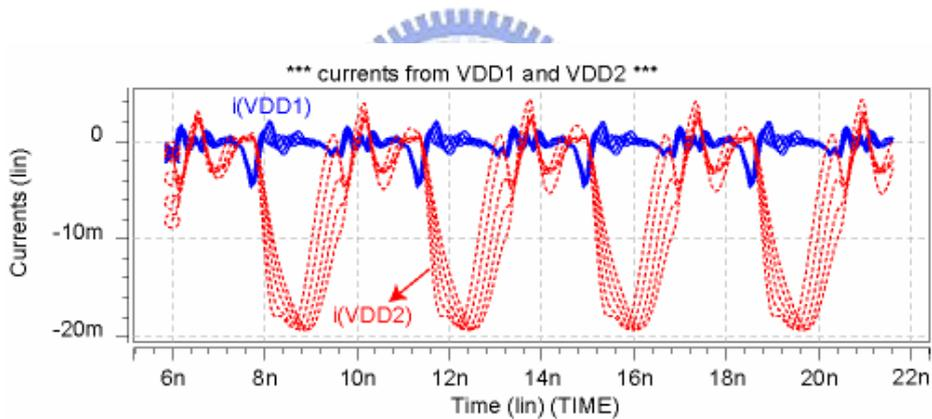
Fig. 4.24 Simulated currents from VDD1 and VDD2 power supply.
