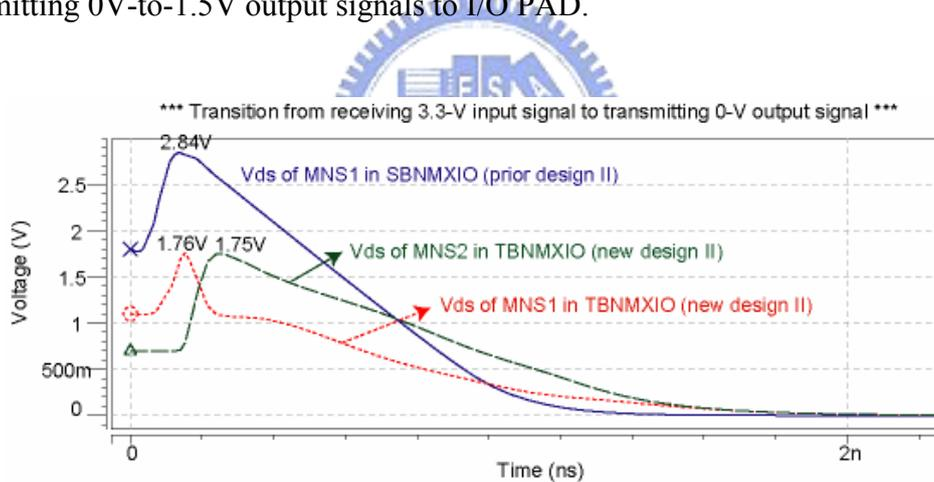
Fig. 3.17 Comparisons of drain-source voltages between the prior design SBNMXIO and new design TBNMXIO during the transition from receiving  $2 \times V_{DD}$  input signal to transmitting 0-V output signal.
