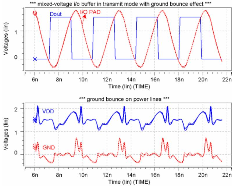
Fig. 4.8 Simulation waveforms of the TBNMXIO-SR with ground bounce effect in transmit mode.
