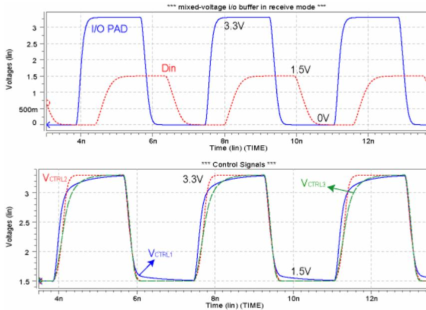
Fig. 3.8 Simulation waveforms of the HCPMXIO in receiving mode with 3.3-V 266-MHz input signals.
