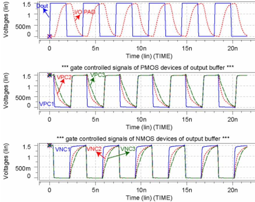
Fig. 4.5 Simulation waveforms of the TBNMXIO-SR operating at 266 MHz when transmitting 0V-to-1.5V output signals to I/O PAD.
