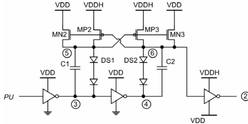
Fig. 2.5 Circuit implementation of the dynamic gate-controlled circuit in the SBNMXIO.
