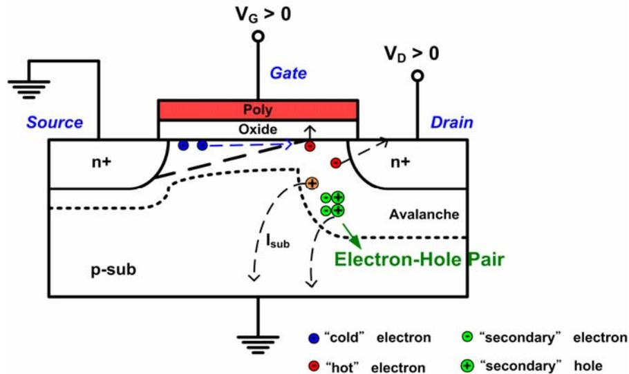
Fig. 1.4 The diagram of hot-carrier effect.
