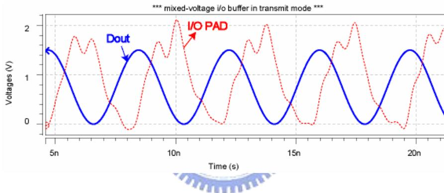
Fig. 3.29 Simulation waveforms of the HCPMXIO with transmission line effect in transmit mode with an operating speed of 266 MHz.
