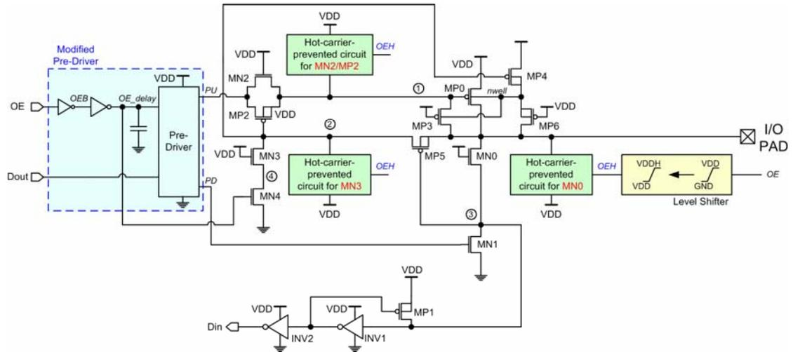
Fig. 3.5 The new mixed-voltage I/O buffer with hot-carrier-prevented circuits (HCPMXIO).
