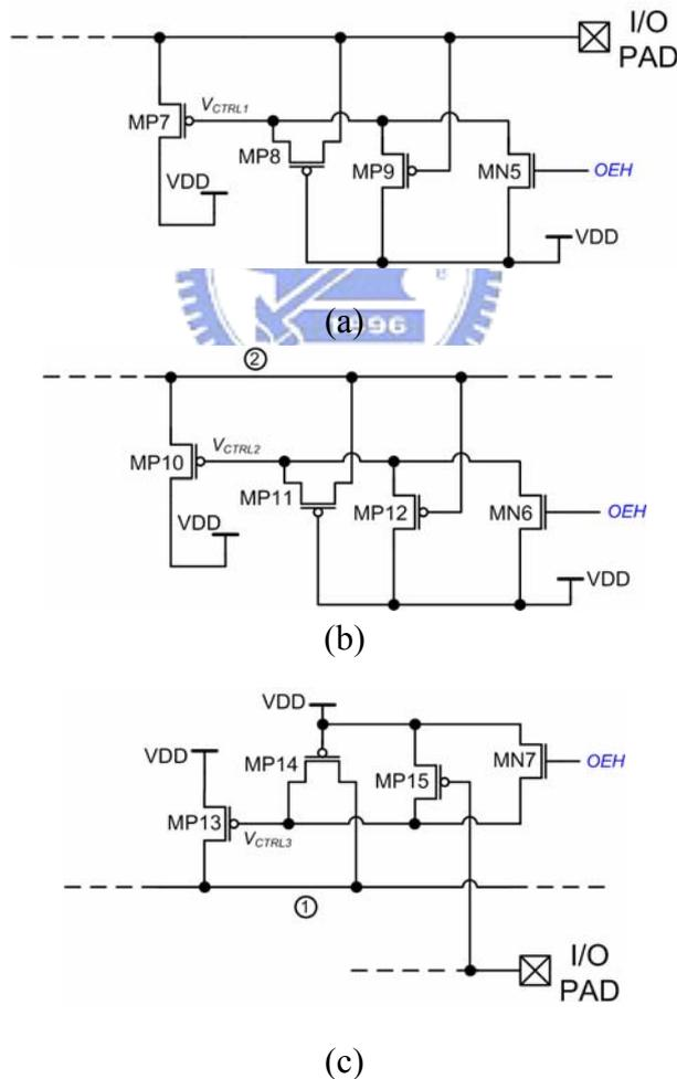
Fig. 3.6 The corresponding hot-carrier-prevented circuits in HCPMXIO. (a) The hot-carrier-prevented circuit for the MN0. (b) The hot-carrier-prevented circuit for the MN3. (c) The hot-carrier-prevented circuit for the MN2 and MP2.
