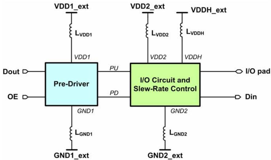
Fig. 4.6 Simulated model of ground bounce.
