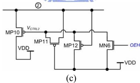
Fig. 4.11 (a) The mixed-voltage I/O buffer based on the HCPMXIO with slew-rate control. (b) The hot-carrier-prevented circuit for transistor MN0 ,and (c) the hot-carrier-prevented circuit for transistor MN3.
