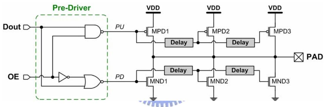
Fig. 4.2 Output buffer with conventional slew-rate control.
