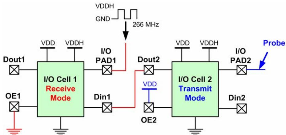
Fig. 4.33 The measurement setting for testing the receiving operations of mixed-voltage I/O buffer.
