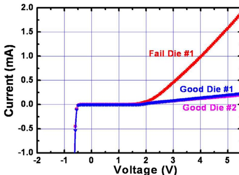
Fig. 7.2. After ND-mode MM ESD stress on I/O pins, the I-V characteristics of VDD2-to-VSS2 showed higher leakage currents than that before ESD stress.
