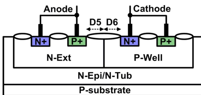
Figure 2.1 The cross-sectional view of triple-well SCR structure.
