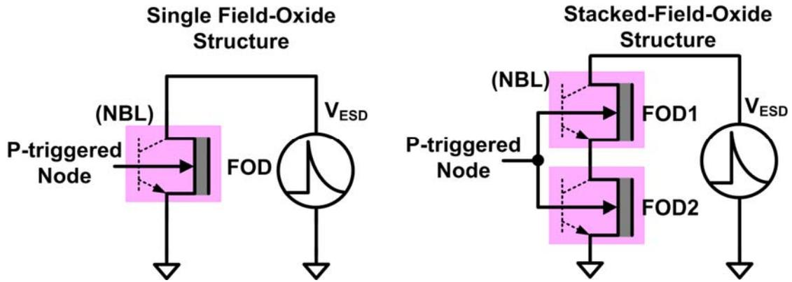
Figure 2.7 The measurement setup of single high-voltage FOD device and stacked-field-oxide structure under TLP stress.
