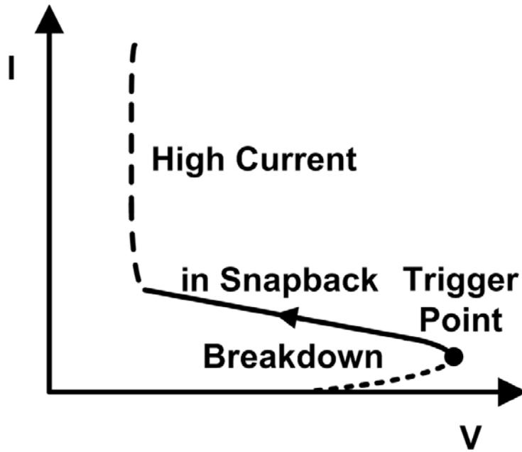
Figure 1.9 The I-V curves for different current regimes of ggLDNMOS: breakdown, BJT triggering, snapback and high current region after holding voltage [8].
