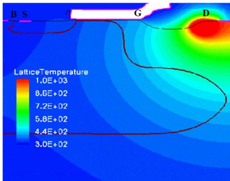
Figure 1.8 The device simulation data on the junction temperature profile within the LDNMOS during the snapback breakdown condition [7].
