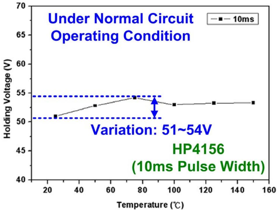
Figure 2.15 Measurement of the temperature dependence of the holding voltage of GC-HVSCR under normal circuit operating condition.
