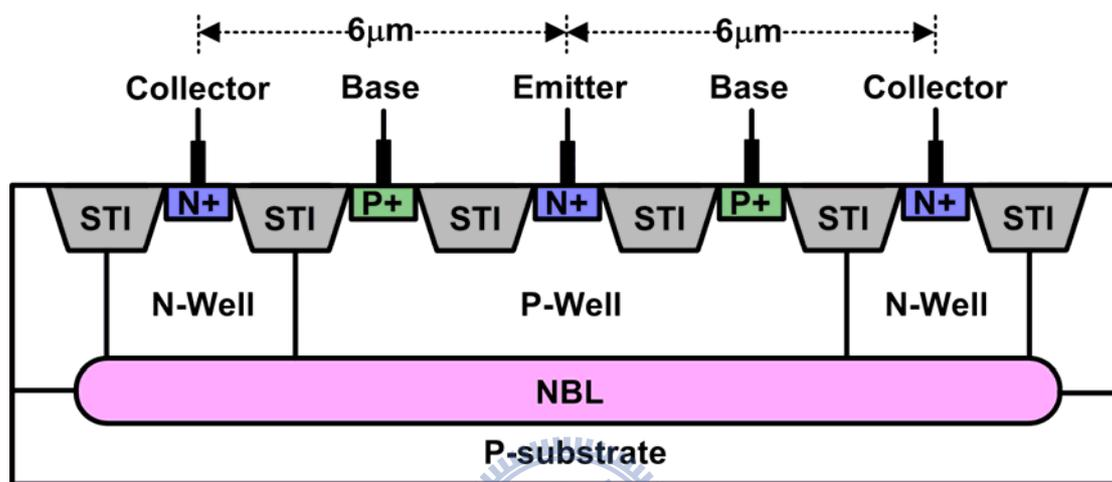
Figure 2.6 The cross-sectional view of high-voltage field-oxide (FOD) device.
