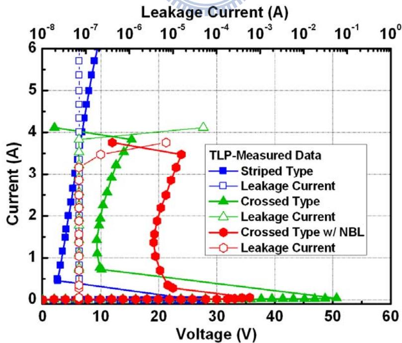
Figure 4.9 The TLP-measured I-V characteristics among the striped type SCR and crossed type SCR and crossed type SCR with NBL.
