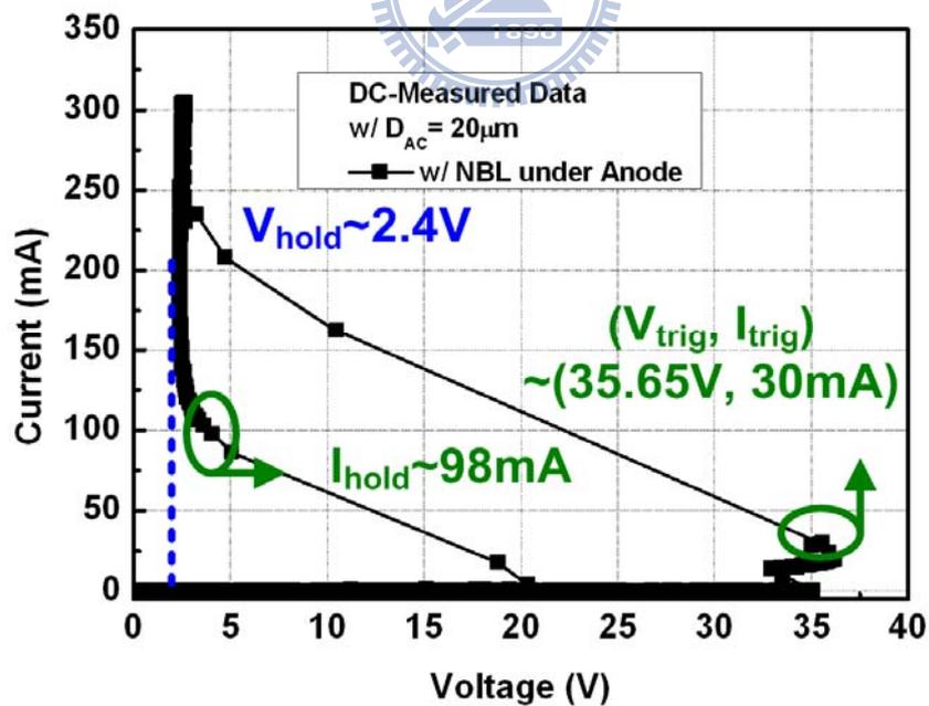
Figure 4.6 The DC-measured I-V characteristics of the single SCR devices (a) without NBL and (b) with NBL under anode while  $D_{AC}$  are  $20\mu\text{m}$ .
