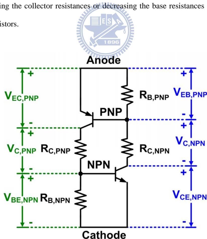
Figure 3.2 The sketch of voltage drops in the SCR device.
