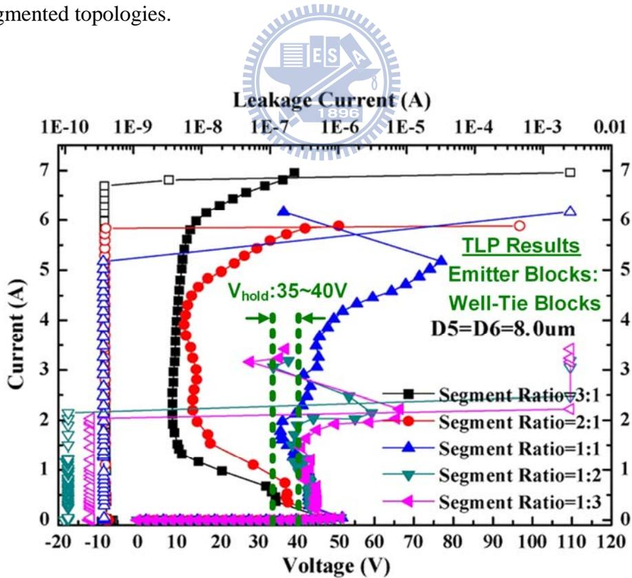
Figure 2.4 The TLP-measured I-V characteristics of SCR devices with different segment ratios and  $D5= D6= 8\mu\text{m}$ .
