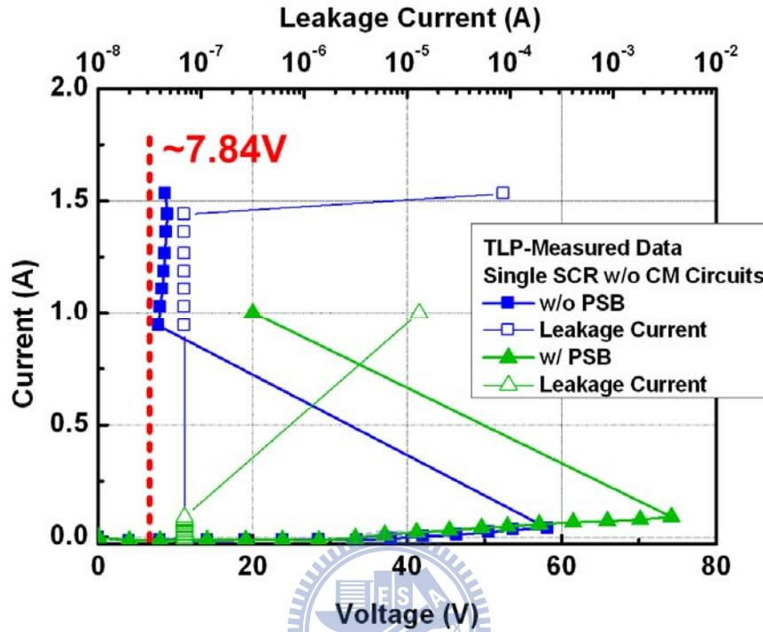
Figure 5.3 The TLP-measured I-V characteristics of single SCR devices without current mirror trigger circuits.
