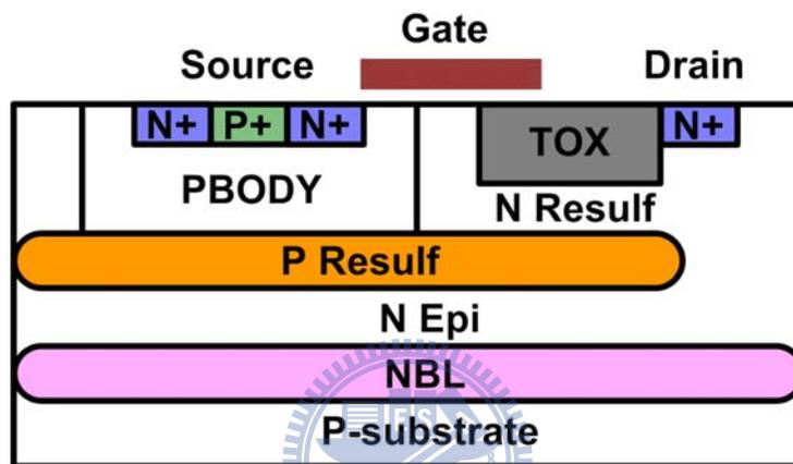
Figure 1.7 The cross-sectional views of RESURF LDMOS [7].
