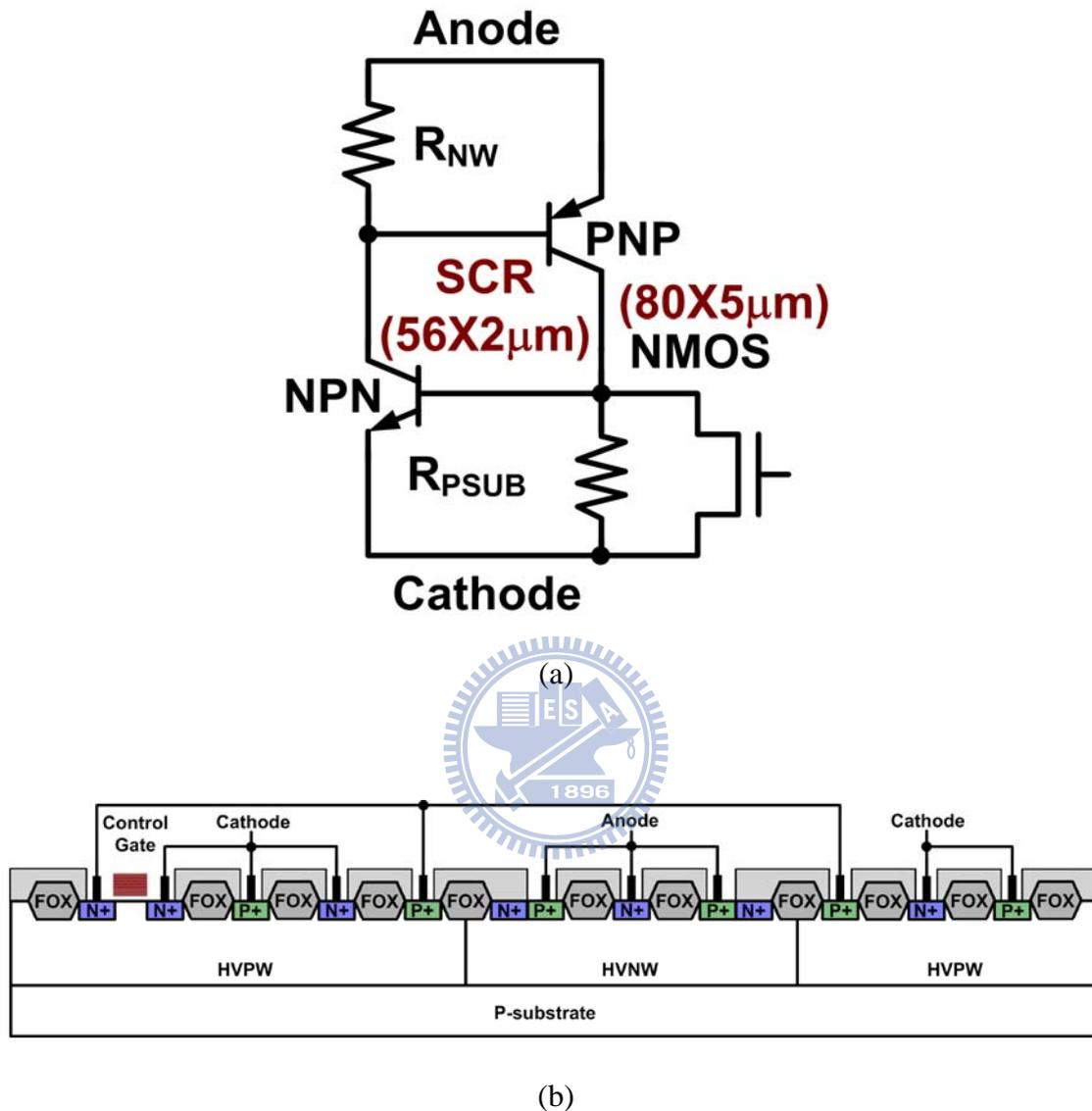
Figure 2.12 The (a) equivalent circuit and (b) cross-sectional view of the GC-HVSCR device.
