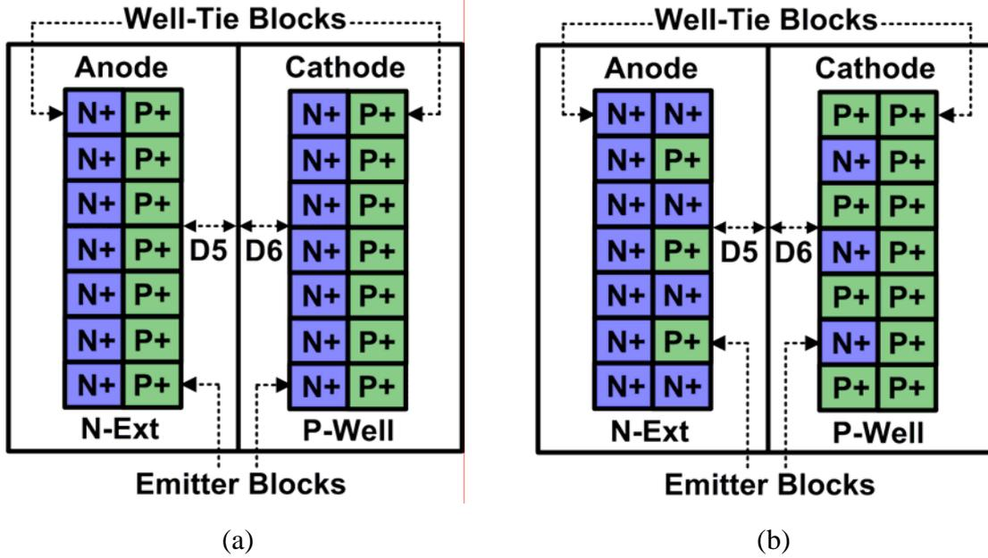
Figure 2.2 The top views of SCR with (a) traditional stripe topology and (b) novel segmented topology.
