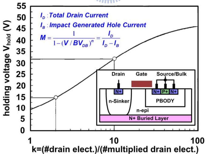
Figure 1.12 Dependence of holding voltage from the ration of the number of electrons that reach the drain to number of avalanche amplified electrons [8].
