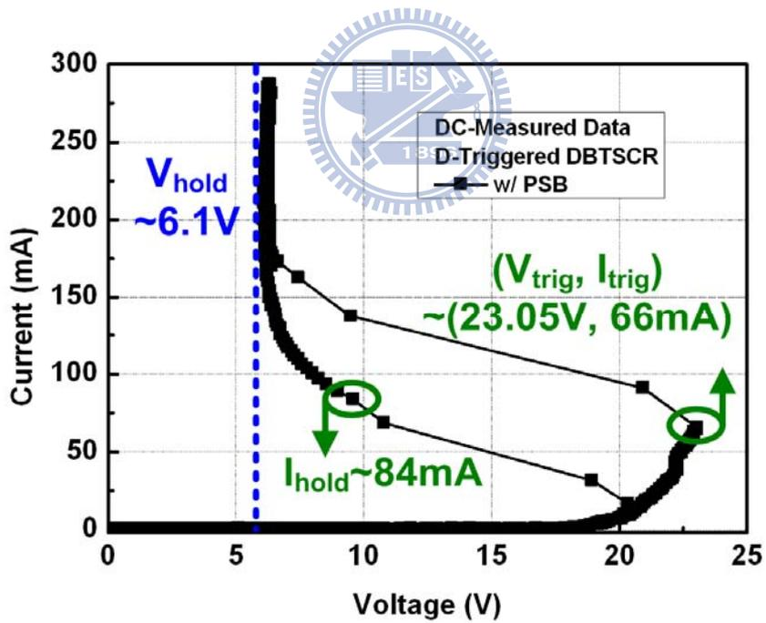
Figure 5.8 The (a) TLP-measured and (b) DC-measured I-V characteristics of d-triggered DBTSCR with PSB.
