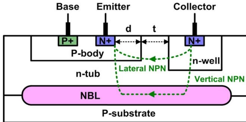
Figure 2.16 The cross-sectional view of the NPN bipolar transistor.
