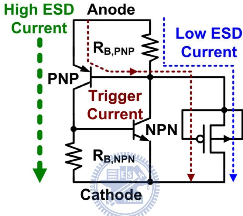
Figure 2.20 The equivalent circuit of PMOS-triggered HVSCR.
