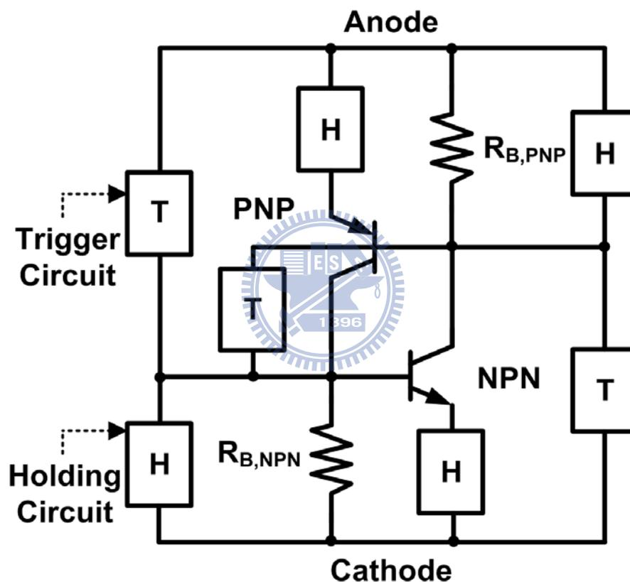
Figure 3.4 The engineering of trigger and holding voltages of the SCR device.
