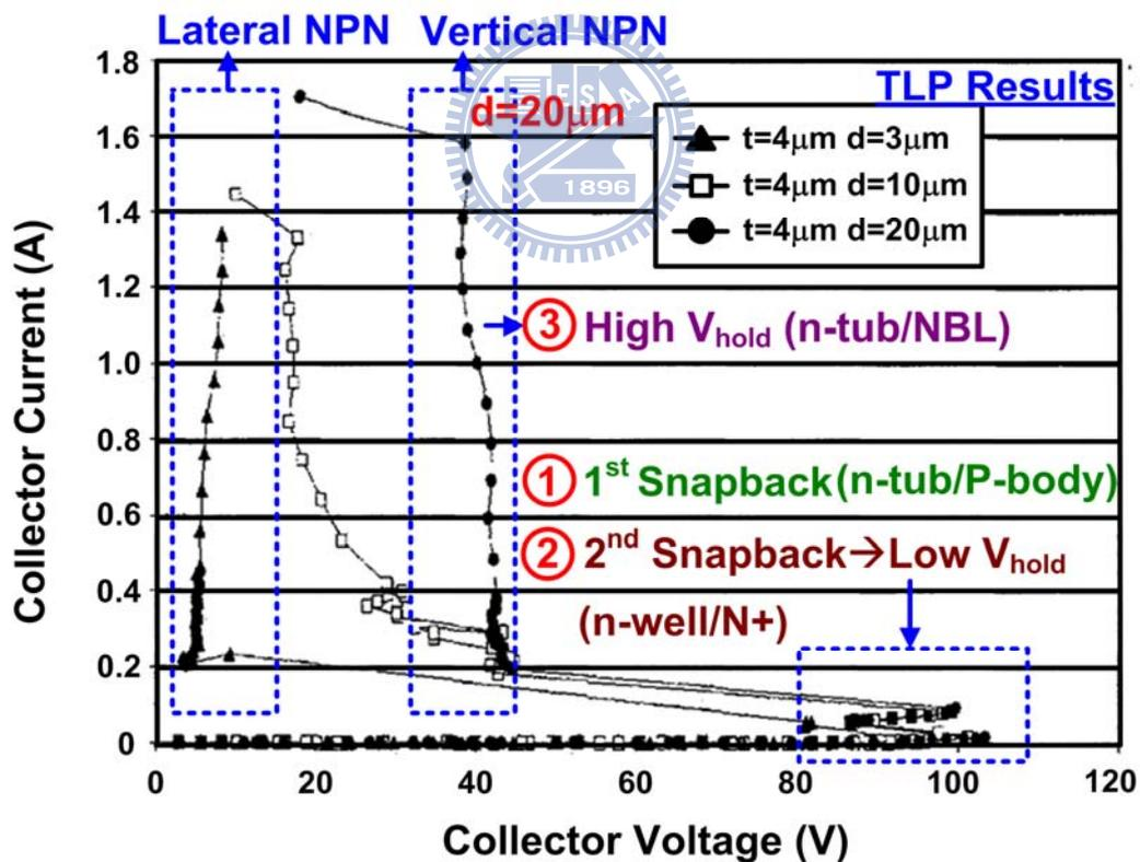
Figure 2.17 The TLP-measured I-V characteristics of the NPN bipolar transistor under different  $d$  values.
