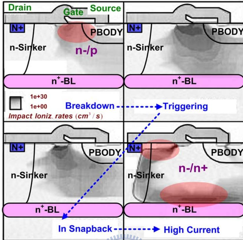
Figure 1.11 Impact ionization rates for different current regimes of ggLDMOS [8].
