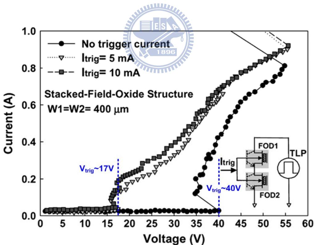
Figure 2.9 The TLP-measured I-V characteristics of the stacked FOD devices with different substrate-triggered currents.
