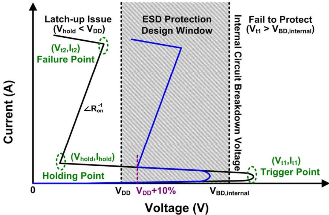
Figure 1.2 The ESD protection design window of HV ESD protection devices [2].
