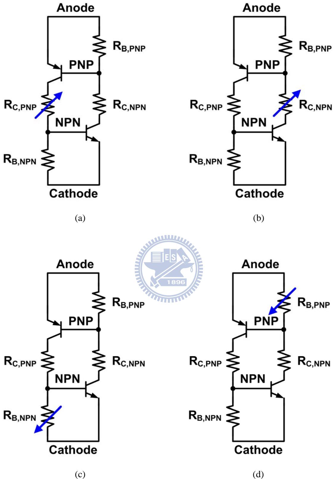
Figure 3.3 The sketches of (a) increasing  $R_{C,PNP}$  and (b) increasing  $R_{C,NPN}$  and (c) decreasing  $R_{B,NPN}$  and (d) decreasing  $R_{B,PNP}$  to boost the holding voltage of SCR devices.
