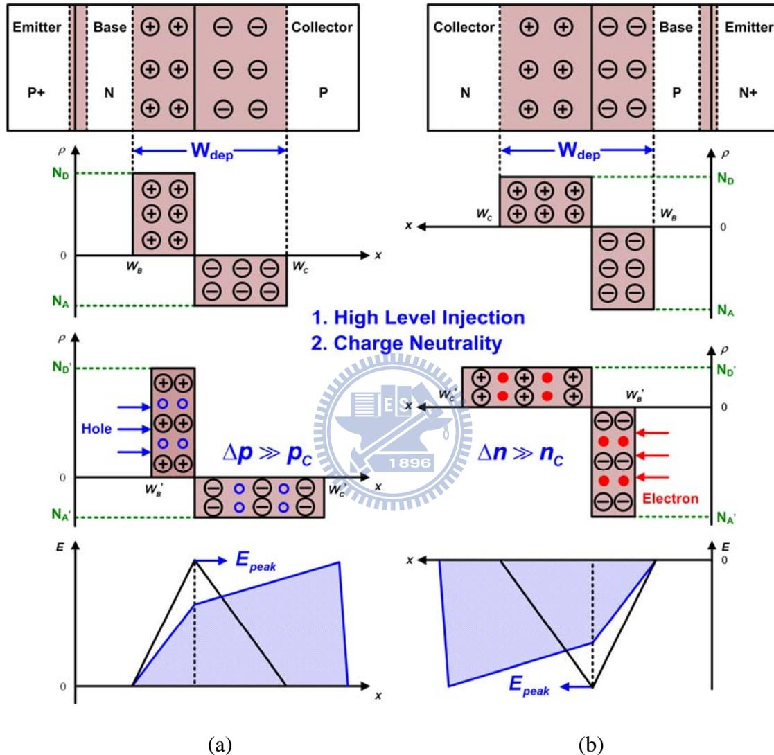
Figure 1.3 The onset schemes of Kirk effect in BJT devices of (a) p-n-p devices and (b) n-p-n devices [3], [4].
