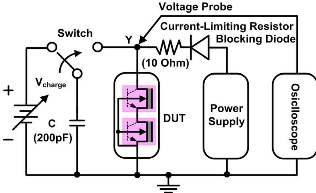
Figure 2.10 Measurement setup for TLU test.
