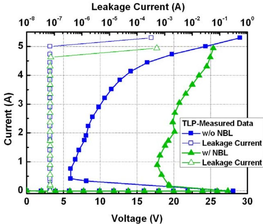
Figure 4.13 The TLP-measured I-V characteristics of the anode-extended SCR devices with and without NBL.
