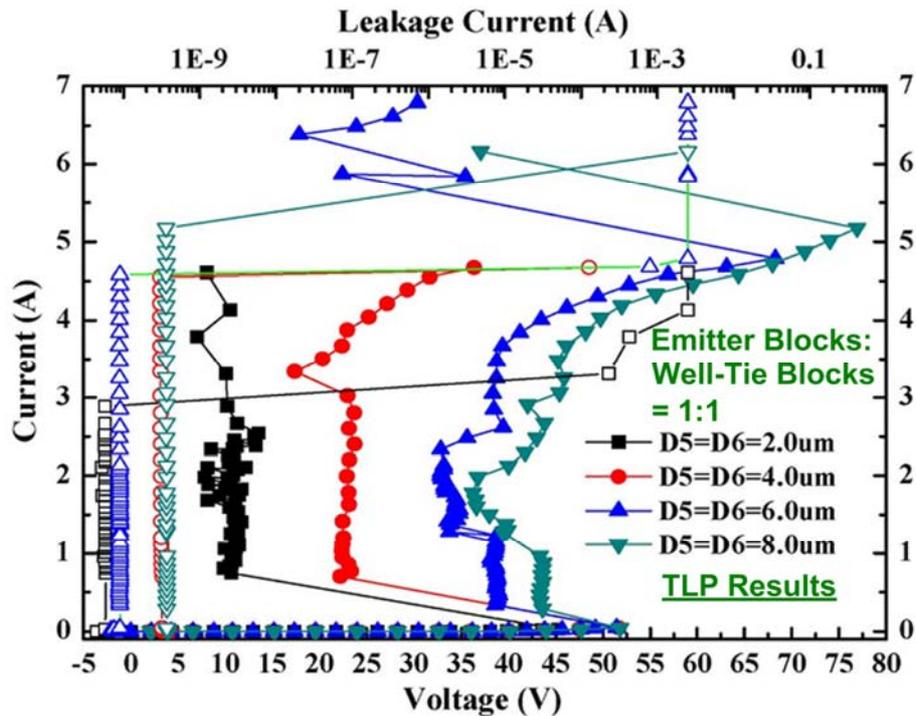
Figure 2.5 The TLP-measured I-V characteristics of SCR devices with 1:1 segment ratio having four D5/ D6 lengths.
