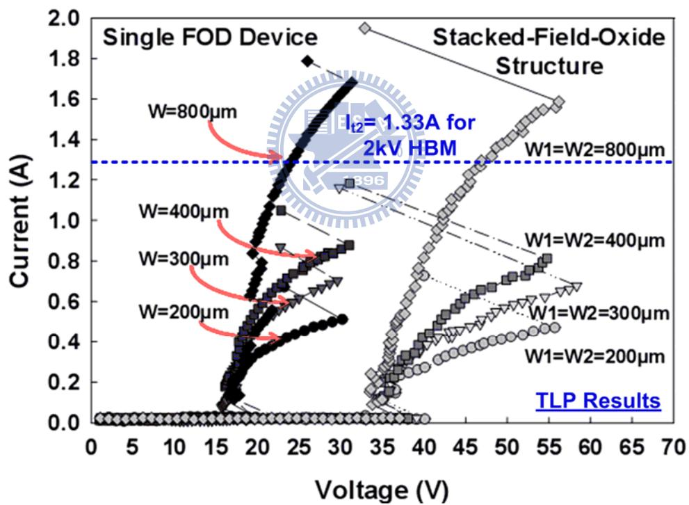
Figure 2.8 The TLP-measured I-V characteristics of single FOD and stacked FOD devices with different device widths.  $W1$  is the channel width of FOD1, and  $W2$  is the channel width of FOD2.
