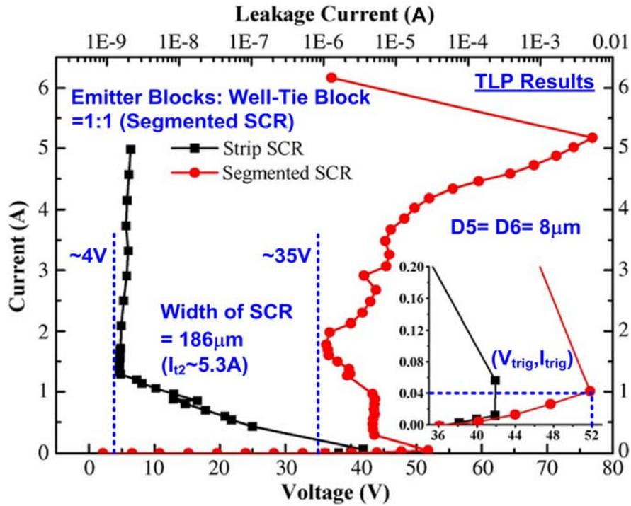
Figure 2.3 The TLP-measured I-V characteristics for two SCR devices with the stripe and segmented topologies.
