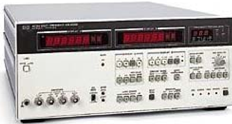
Fig. 3.4 The LCR meter which is used for the measurement of capacitance (Agilent 4275A).
