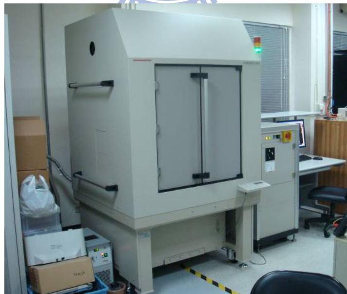
Fig. 2.3 HAMAMATSU Phemos-1000 Emission Microscope system.
