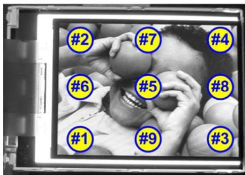
Fig. 4.12 Test points definition on display panel under system-level ESD tests with air-discharge test mode.
