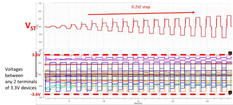
Fig. 2.22 Overstress test under (a) current-mode (b) voltage-mode stimulation.
