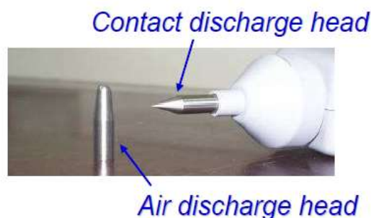
Fig. 2.2 Discharge heads of ESD gun that used under system-level ESD test with contact-discharge mode and air-discharge mode.
