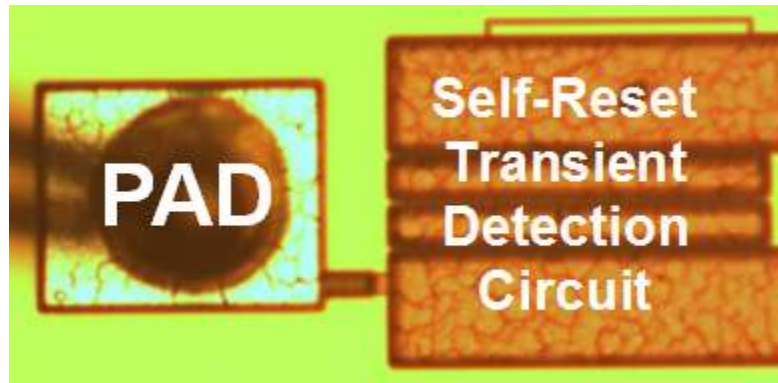
Fig. 4. 8 Die photo of the proposed on-chip self-reset transient detection circuit.
