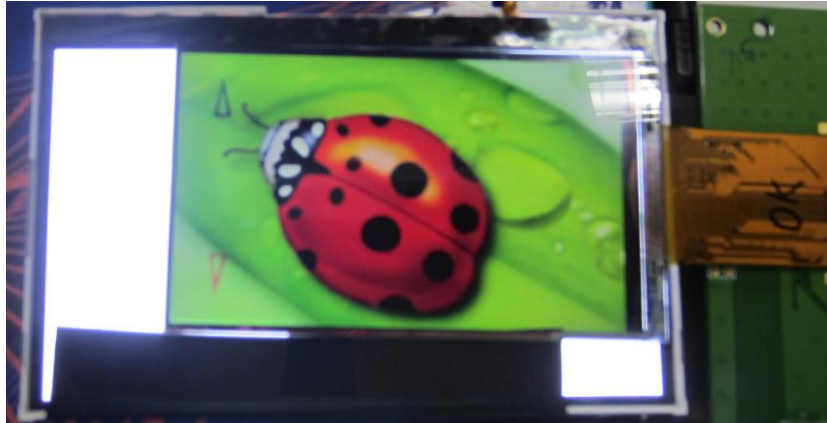
Fig. 3.12. The display image of a 4.5-inch WXGA panel for (a) forward direction scanning and (b) backward direction scanning.
