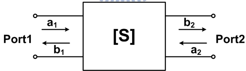
Fig. 2.1. A two-port network described with S-parameters.
